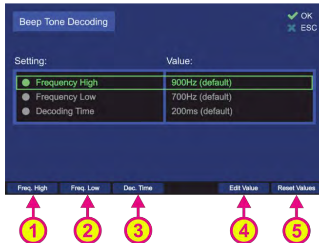
Figure 97. Beep tone decoding settings
