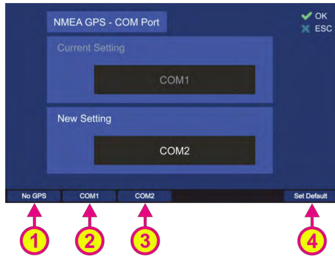
Figure 121. NMEA GPS communication port settings
