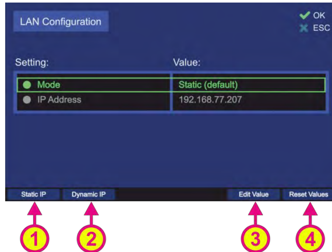
Figure 113. LAN configuration menu
