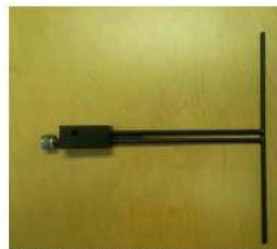
Figure 1 – MVG COMOSAR Validation Dipole
