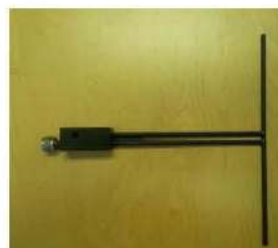
Figure 1 – MVG COMOSAR Validation Dipole
