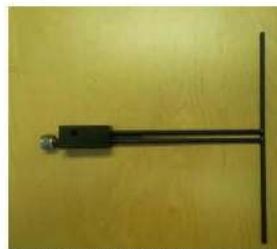
Figure 1 – MVG COMOSAR Validation Dipole
