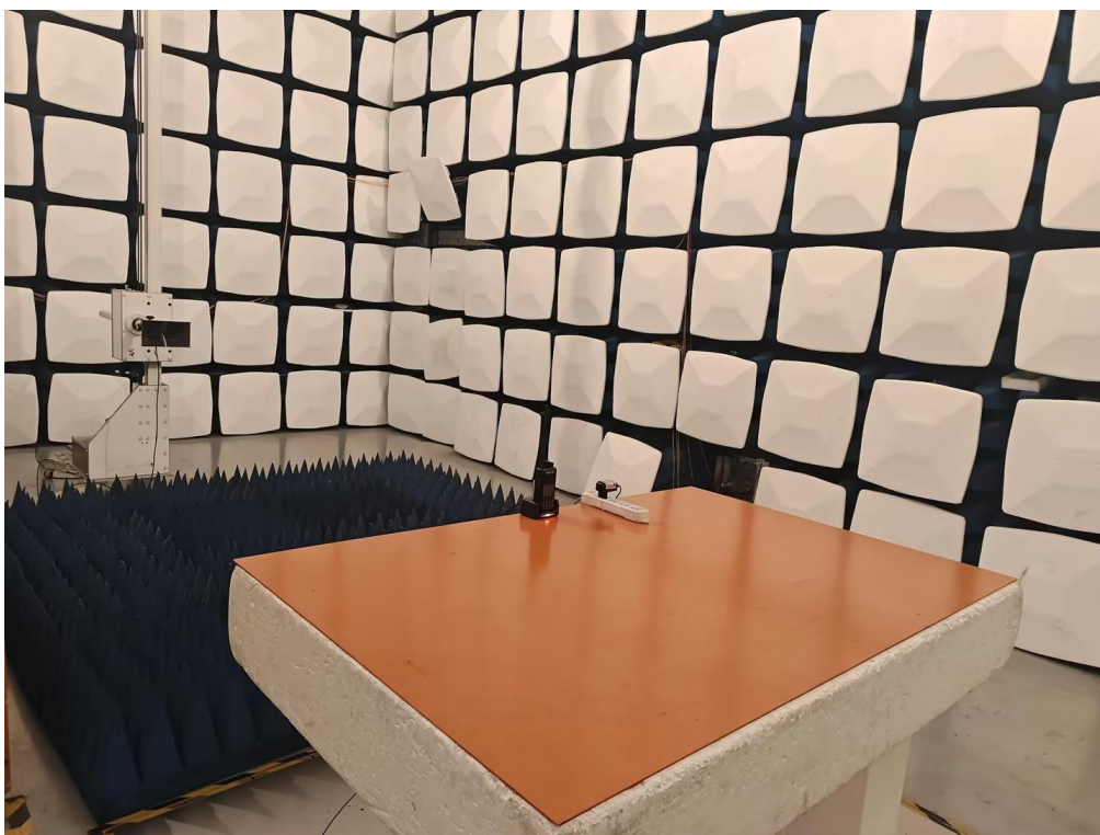
Photo of Radiated Measurement (Above 1GHz)
