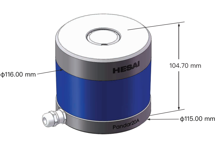
Figure 2.1 Pandar20A/B Side View
