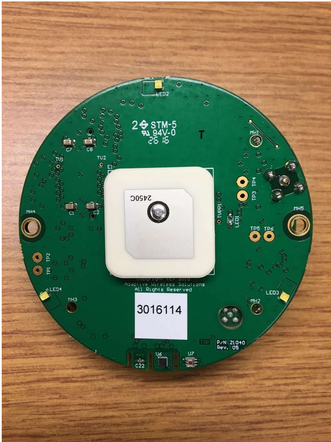
Top of RF PCB (BLE WLP.2450.25.4.A.02 antenna)
