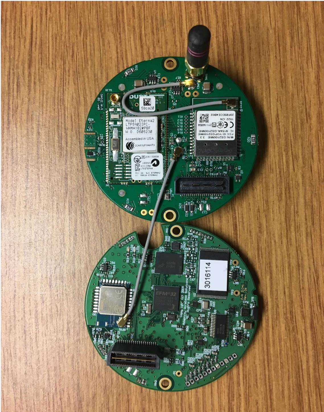
Top of Sensor PCB (lower) & Bottom of RF PCB (upper)
