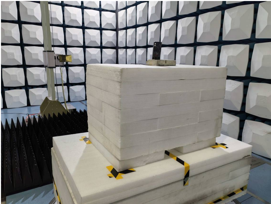
Radiated Emission 18-26.5GHz View
