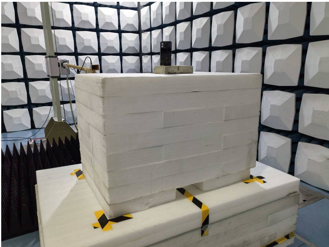
Radiated Emission 18-26.5GHz View
