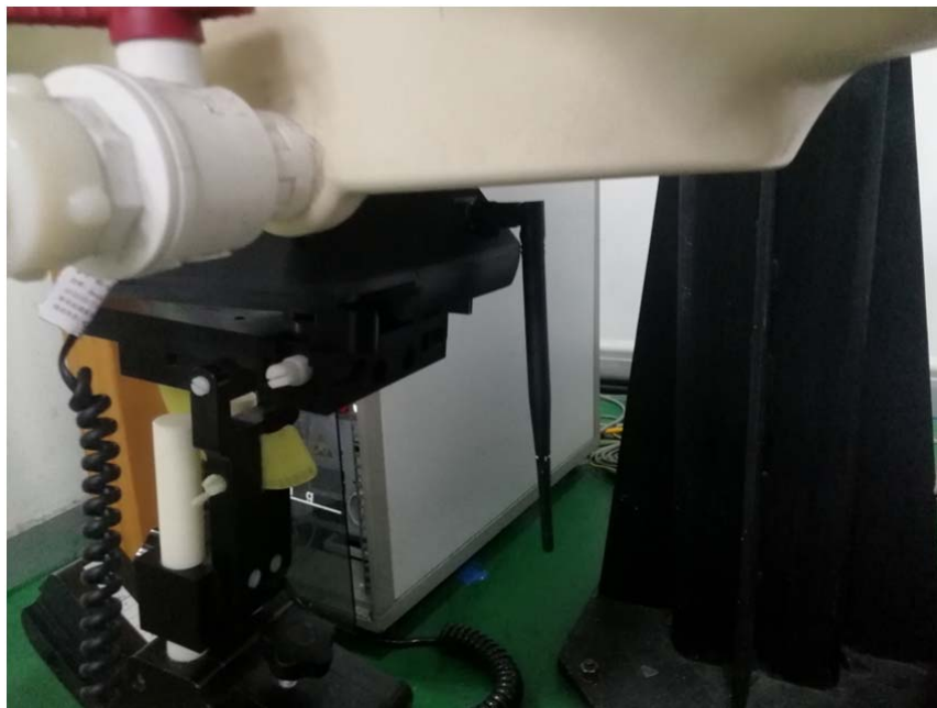
Body (Worn) Back With Antenna Vertical Setup Photo (0mm)
