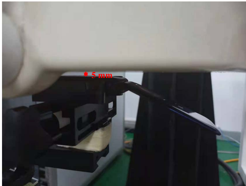
Body Back Setup Photo (5mm)
