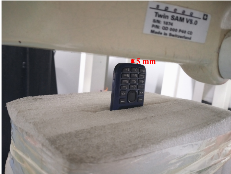
Body Bottom Setup Photo (5 mm)
