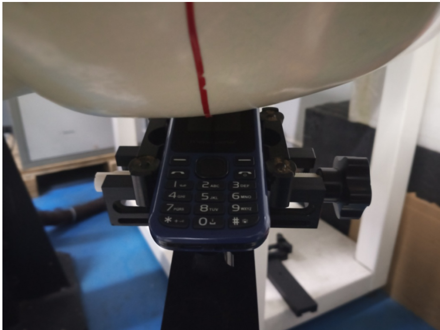
Head Left Tilt Setup Photo(0mm)
