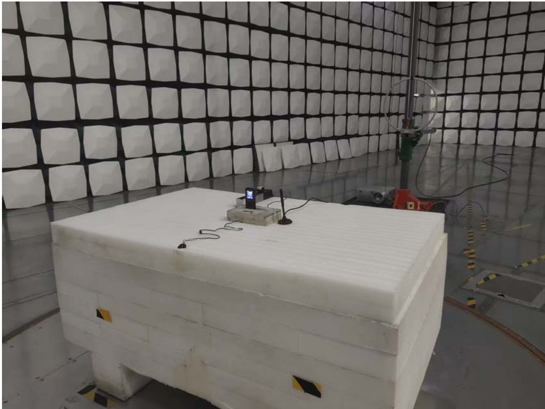
Radiated Emission 9kHz-30MHz Perpendicular View
