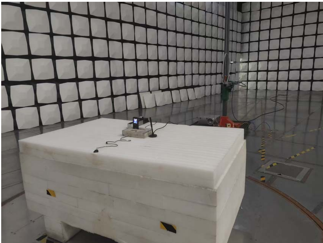
Radiated Emission 9kHz-30MHz Perpendicular View
