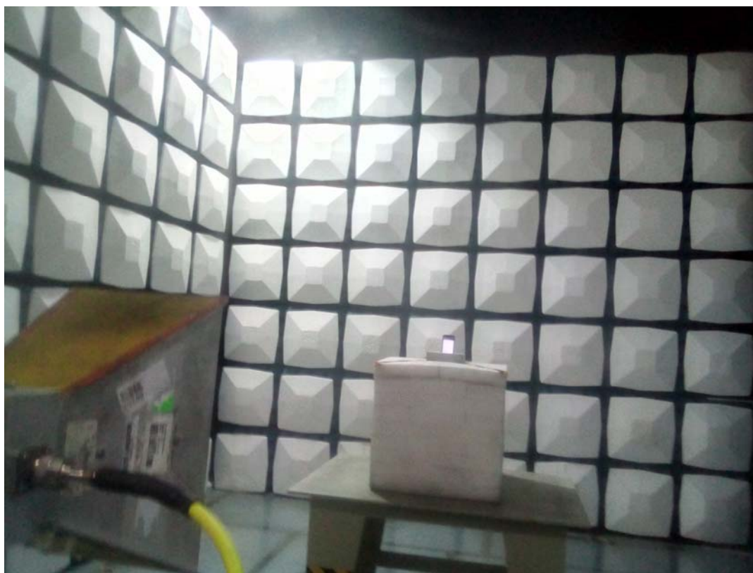
Radiated Emission Above 1GHz View
