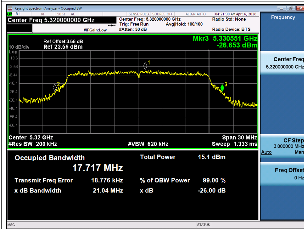
-26dB Bandwidth NVNT n20 5320MHz Ant B
