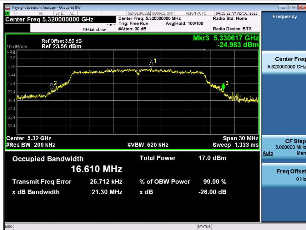
-26dB Bandwidth NVNT n20 5260MHz Ant B
