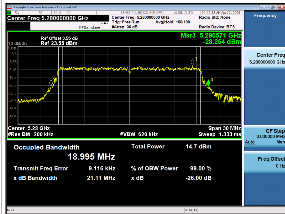
-26dB Bandwidth NVNT ax20 5280MHz Ant A
