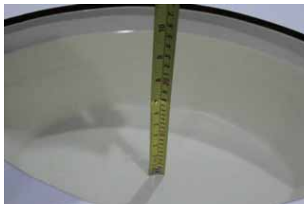
Liquid depth in the body phantom (5GHz)
