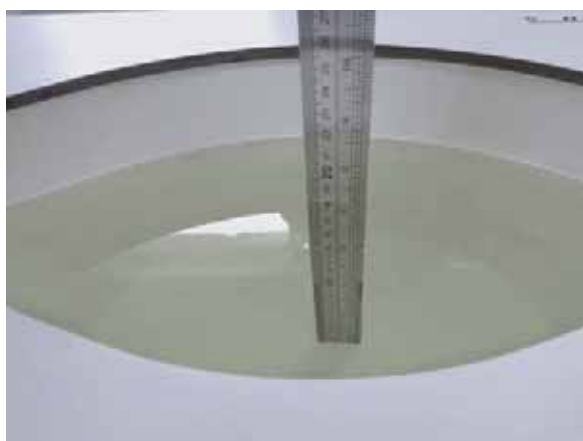
Liquid depth in the head phantom (2450MHz)
