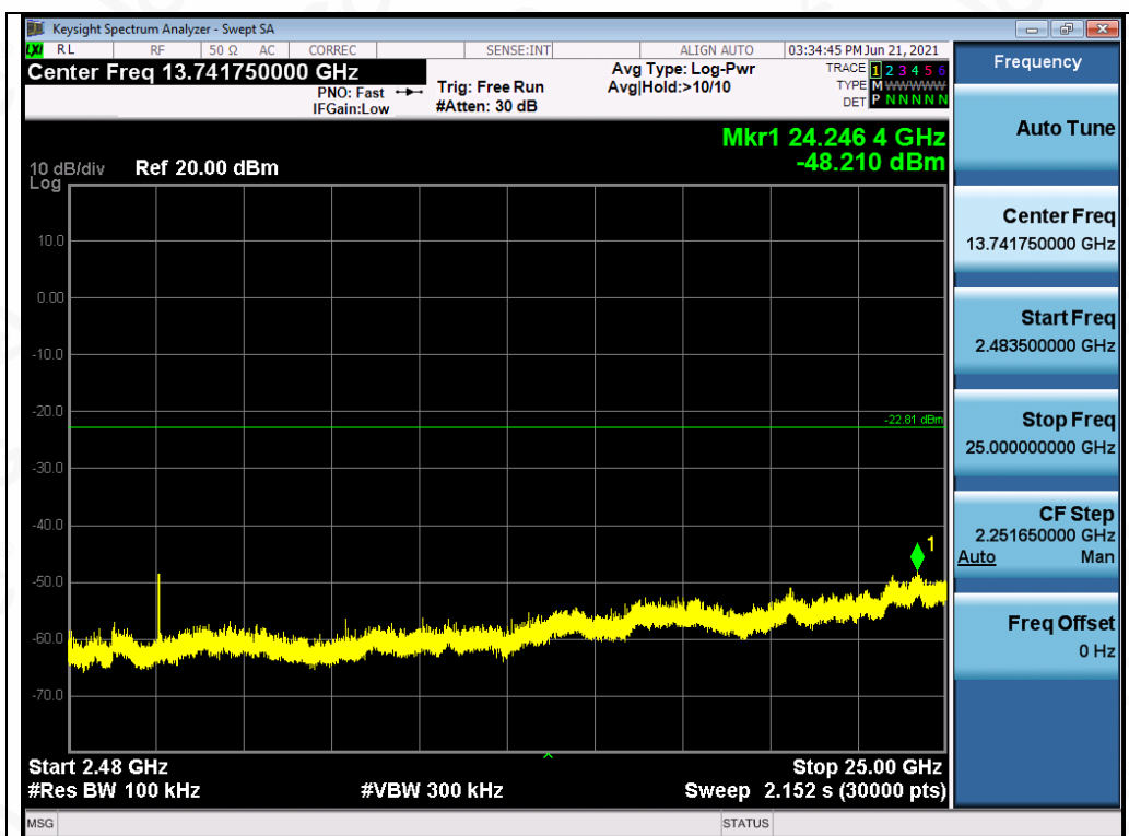
Test_Graph_BR_ANT1_2402_1Mbps_Higher Band Emissions
