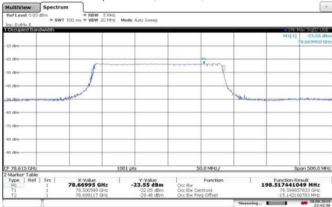
Occupied Bandwidth, Mid Channel, 198.517 MHz
