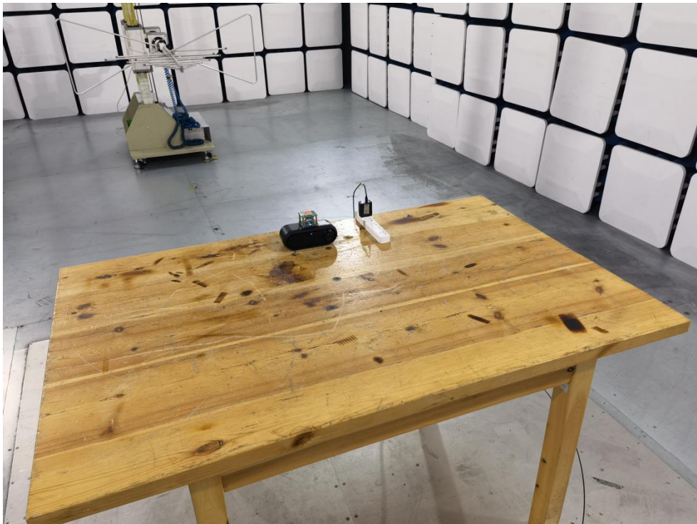
Photo of Radiation Emission Test
