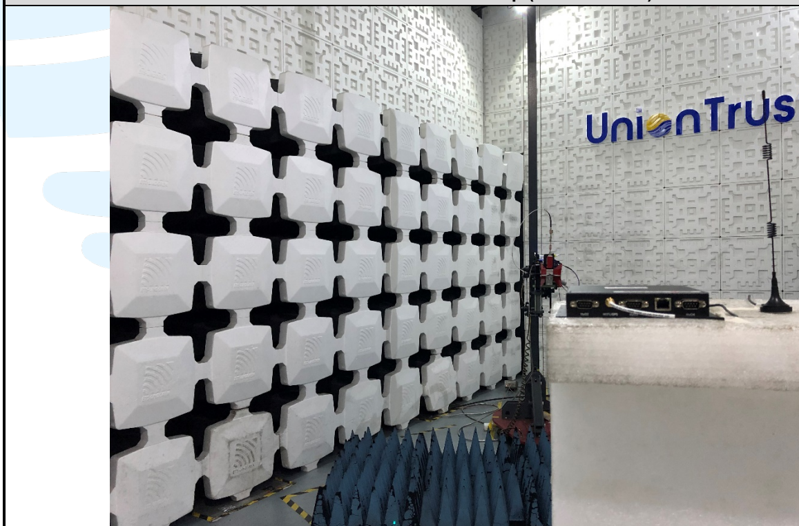
Radiated emission Test Setup (Above 1 GHz)
