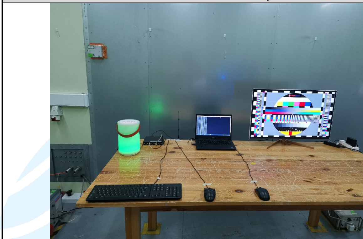
Conducted Emission Test Setup
