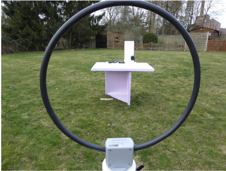
181948_7.JPG : Test setup final measurement from 9 kHz to 30 MHz
