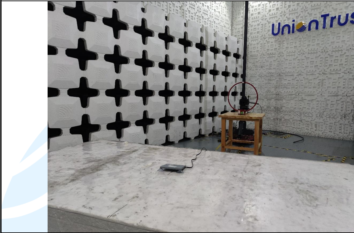
Radiated emission Test Setup (Below 30 MHz)
