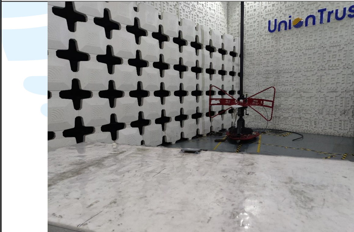
Radiated emission Test Setup (30 MHz~1 GHz)
