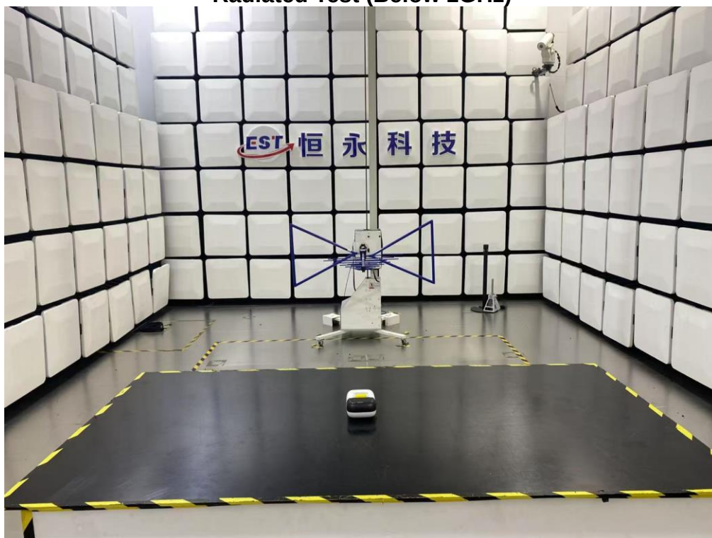
Radiated Test (Below 1GHz)
