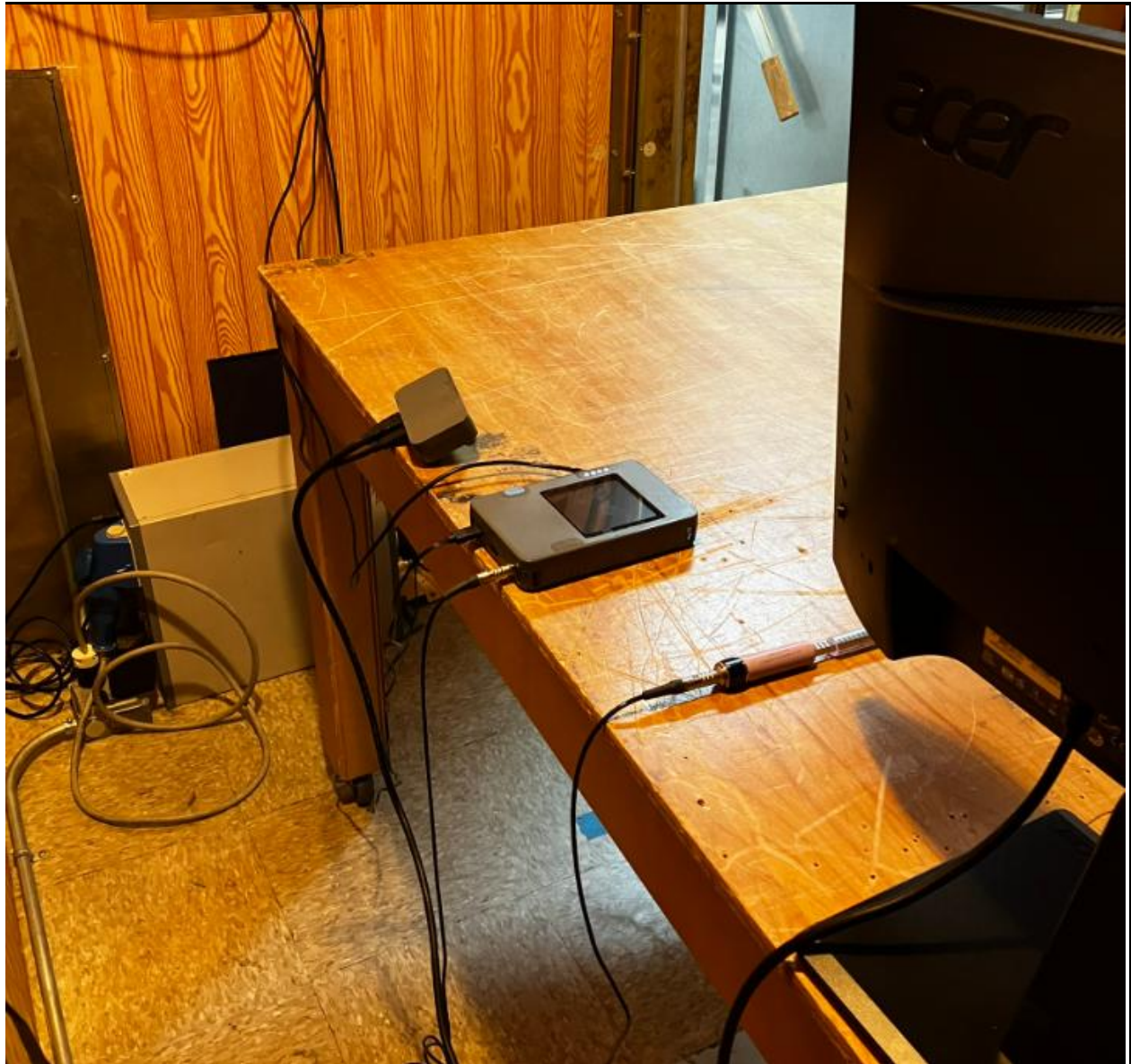
Photograph 6: AC Conducted Emissions - Rear View
