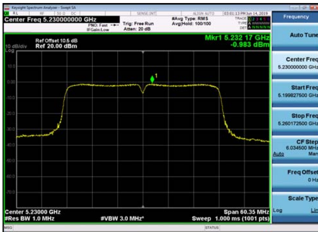
U-NII-1 Power spectral density-802.11 ac(80MHz),5210MHz,Ant0
