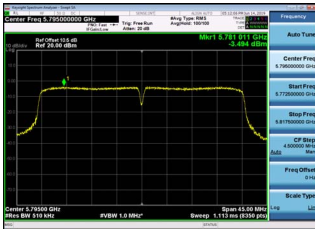
U-NII-3 Power spectral density-802.11 a(20MHz),5745MHz,Ant0
