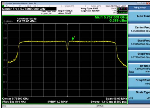
U-NII-3 Power spectral density-802.11 ac(40MHz),5795MHz,Ant0
