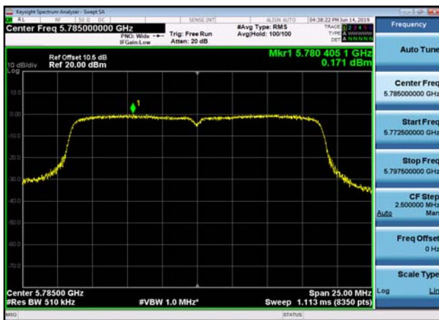
U-NII-3 Power spectral density-802.11 ac(20MHz),5785MHz,Ant0
