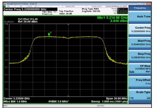
U-NII-1 Power spectral density-802.11 n(20MHz),5240MHz,Ant1
