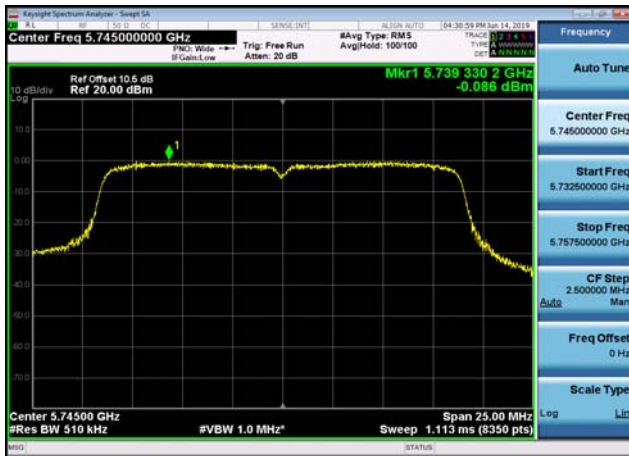
U-NII-3 Power spectral density-802.11 ac(20MHz),5785MHz,Ant0
