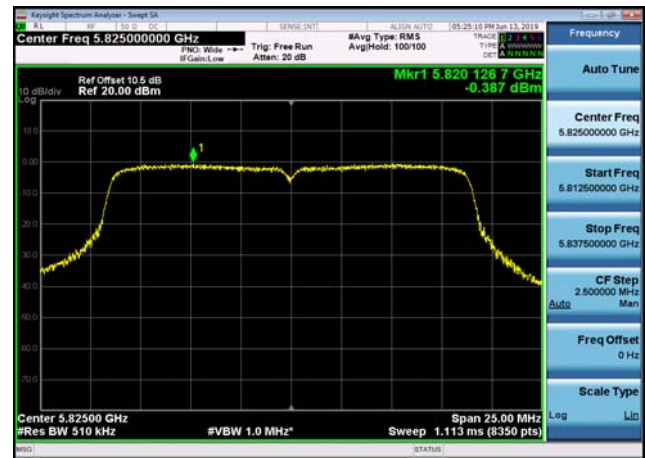
U-NII-3 Power spectral density-802.11 ac(40MHz),5755MHz,Ant1
