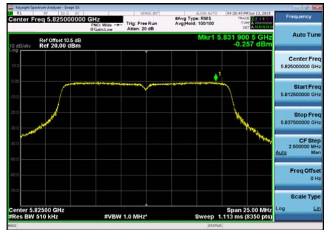
U-NII-3 Power spectral density-802.11 ac(20MHz),5745MHz,Ant1
