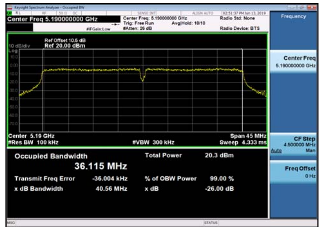
U-NII-1 26dB Bandwidth-802.11n(40MHz) ,5230MHz,Ant1
