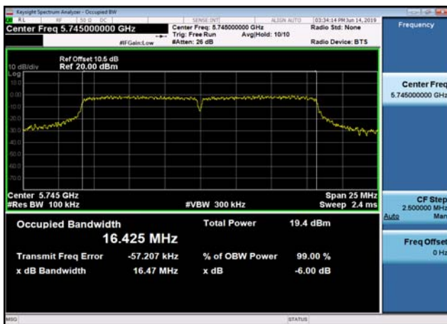
U-NII-3 6dB Bandwidth-802.11a(20MHz) ,5785MHz,Ant0
