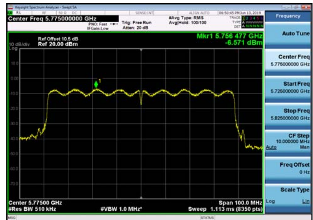
U-NII-3 Power spectral density-802.11 ac(80MHz),5775MHz,Ant1
