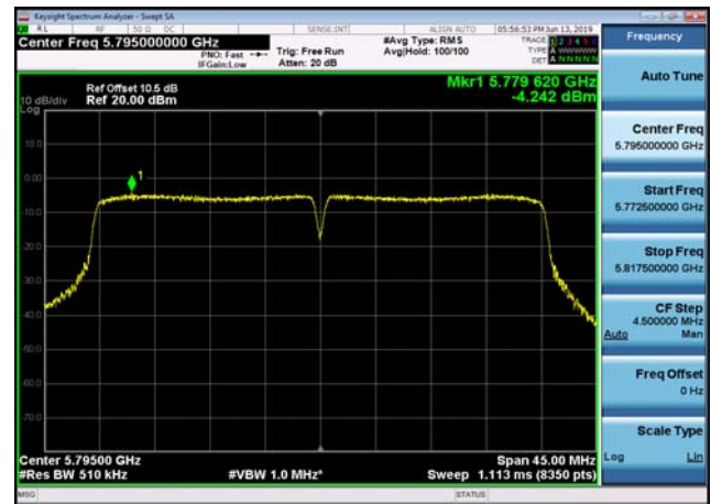
U-NII-3 Power spectral density-802.11 a(20MHz),5745MHz,Ant1
