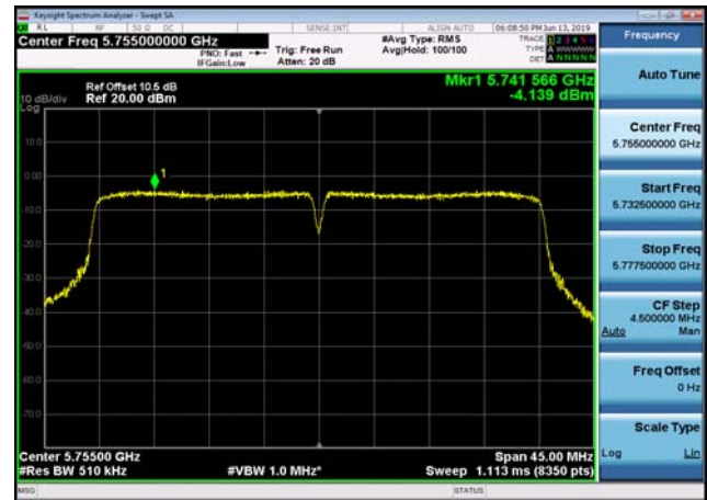
U-NII-3 Power spectral density-802.11 ac(40MHz),5795MHz,Ant1
