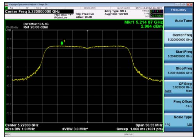
U-NII-1 Power spectral density-802.11 a(20MHz),5240MHz,Ant1
