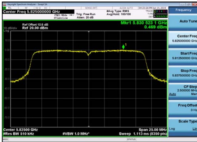
U-NII-3 Power spectral density-802.11 n(40MHz),5755MHz,Ant0
