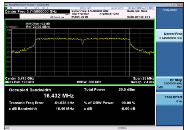
U-NII-3 6dB Bandwidth-802.11a(20MHz) ,5785MHz,Ant1
