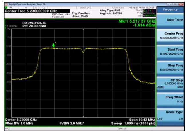
U-NII-1 Power spectral density-802.11 ac(80MHz),5210MHz,Ant1
