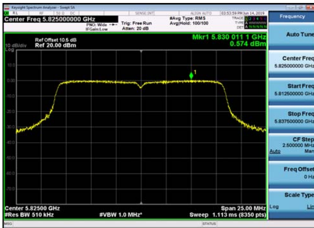
U-NII-3 Power spectral density-802.11 ac(20MHz),5745MHz,Ant0
