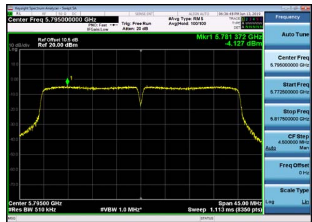
U-NII-3 Power spectral density-802.11 ac(40MHz),5795MHz,Ant1
