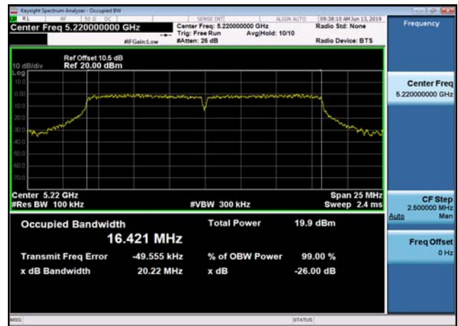
U-NII-1 26dB Bandwidth-802.11a(20MHz) ,5240MHz,Ant1
