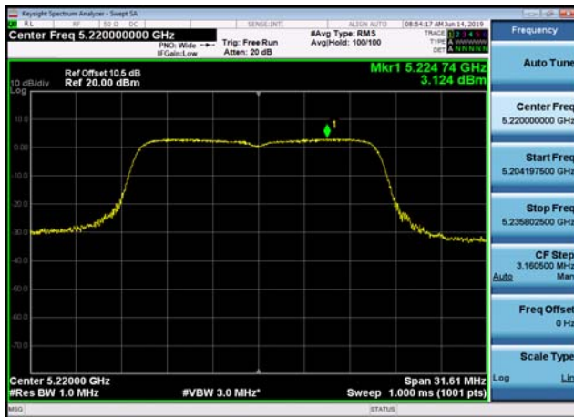
U-NII-1 Power spectral density-802.11 a(20MHz),5240MHz,Ant0
