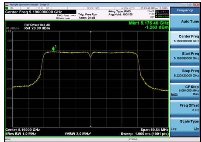
U-NII-1 Power spectral density-802.11 n(40MHz),5230MHz,Ant1
