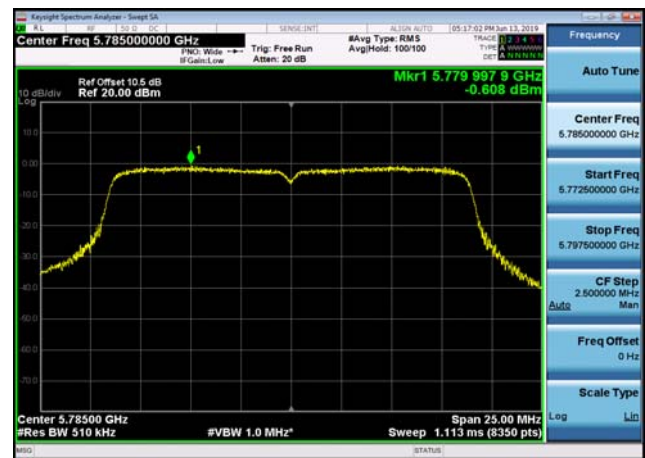
U-NII-3 Power spectral density-802.11 ac(20MHz),5785MHz,Ant1
