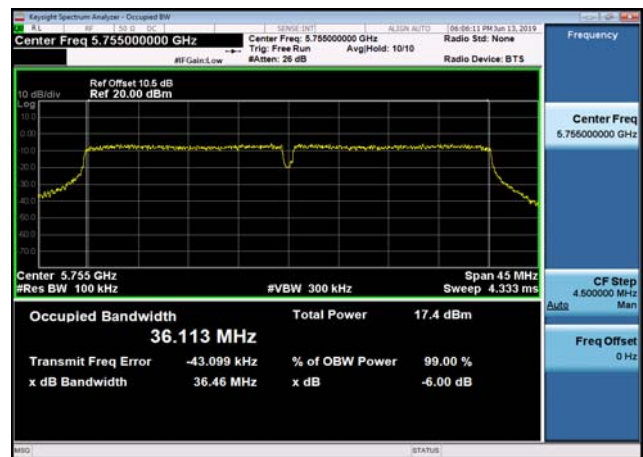
U-NII-3 6dB Bandwidth-802.11ac(40MHz) ,5795MHz,Ant1
