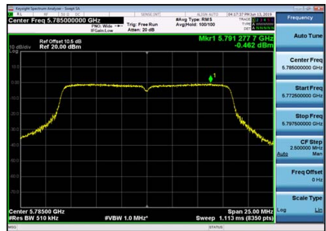
U-NII-3 Power spectral density-802.11 a(20MHz),5785MHz,Ant1
