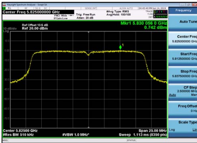
U-NII-3 Power spectral density-802.11 ac(40MHz),5755MHz,Ant0
