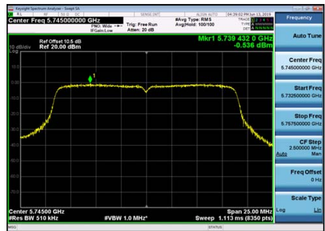
U-NII-3 Power spectral density-802.11 n(20MHz),5745MHz,Ant1
