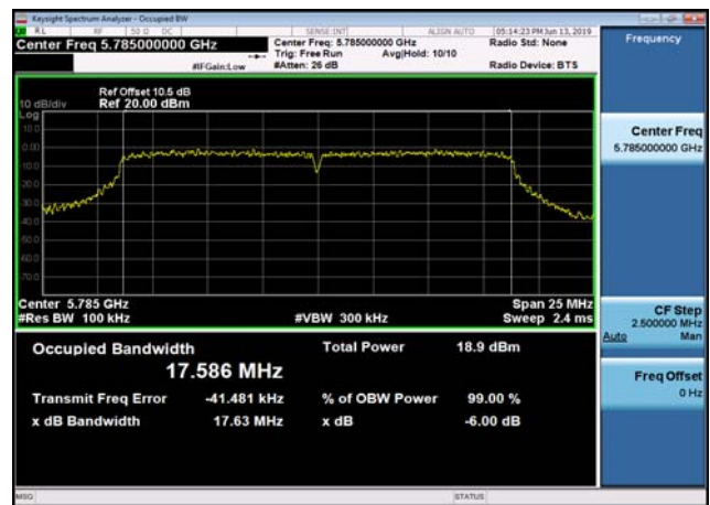
U-NII-3 6dB Bandwidth-802.11ac(20MHz) ,5785MHz,Ant1
