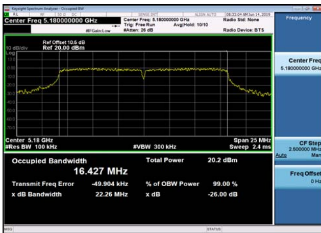
U-NII-1 26dB Bandwidth-802.11a(20MHz) ,5180MHz,Ant0
