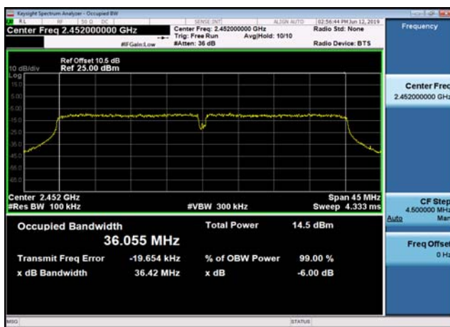
6dB Bandwidth-802.11n(HT40),2452MHz ,Ant0
