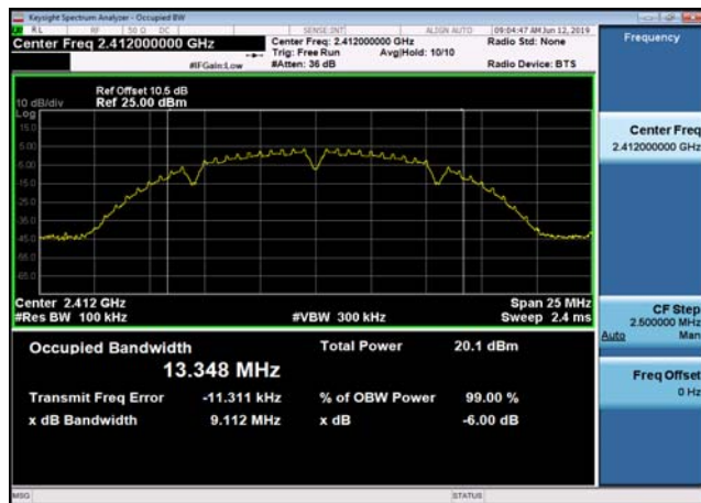
6dB Bandwidth-802.11b,2437MHz,Ant0
