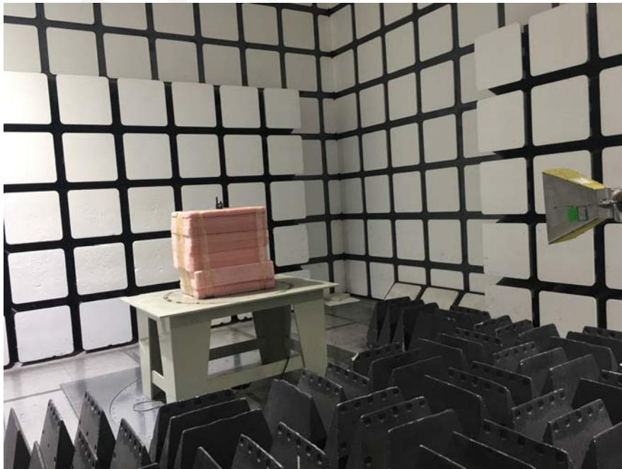
Radiated Emissions View (Above 1 GHz)
