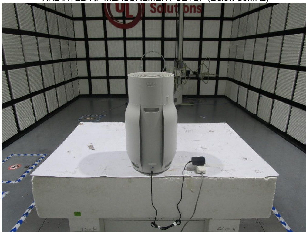
RADIATED RF MEASUREMENT SETUP (Below 30MHz)
