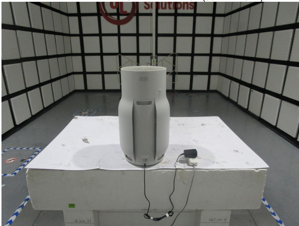
RADIATED RF MEASUREMENT SETUP (Below 30MHz)
