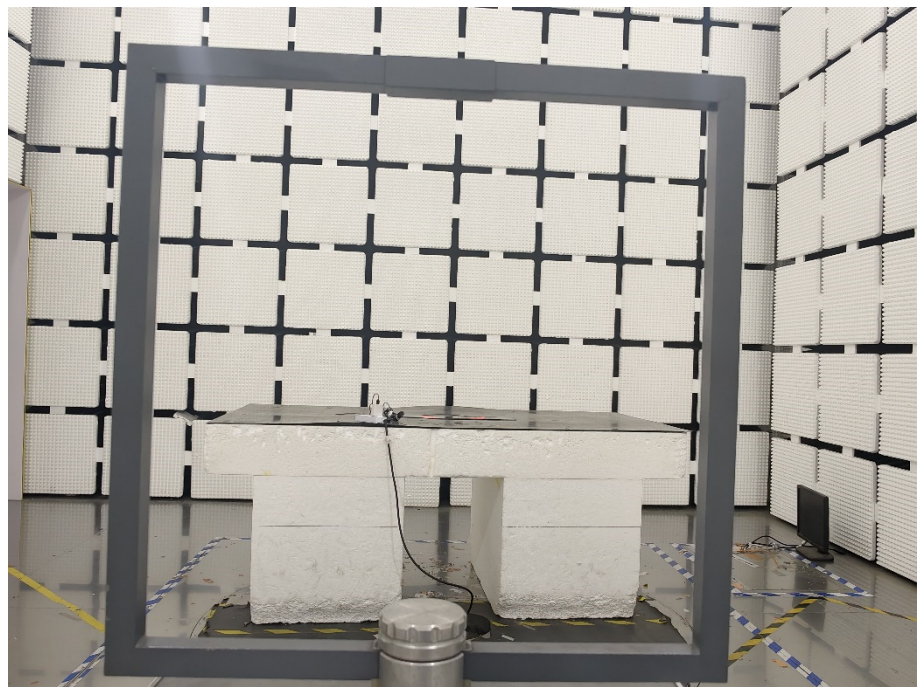
Radiation Emission Test Setup (Below 30MHz)
