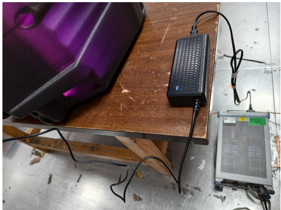
Conducted Emission Test Setup(close up)
