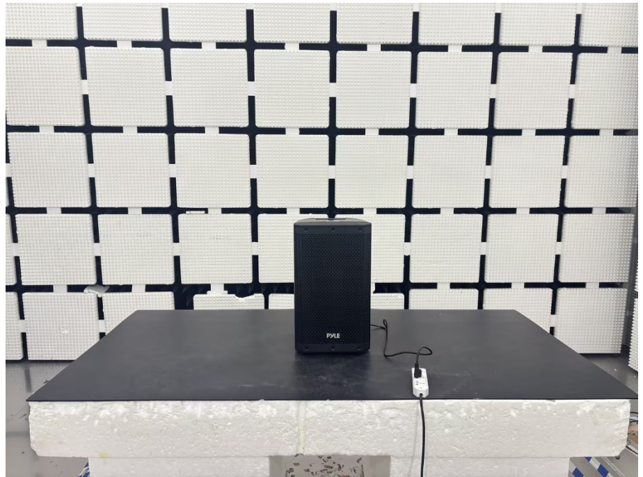
Radiation Emission Test Setup(close up)
