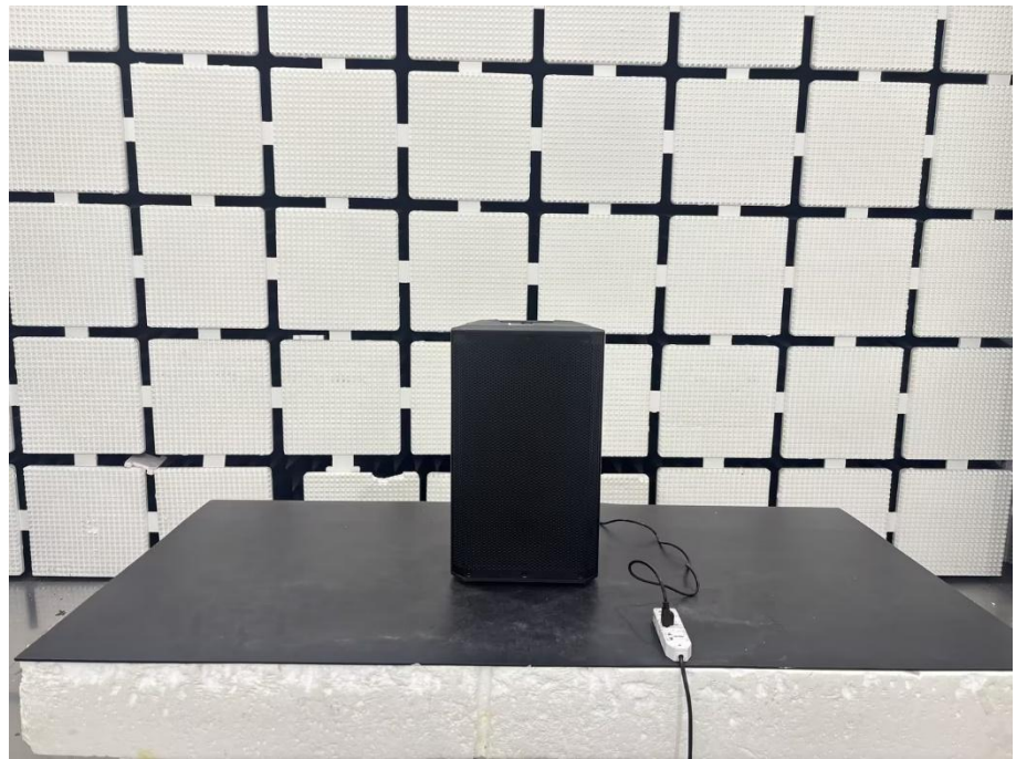
Radiation Emission Test Setup (close up)
