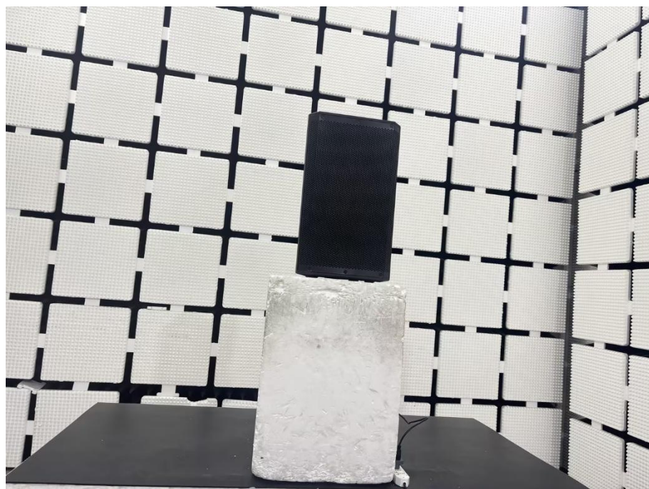
Radiation Emission Test Setup (close up)
