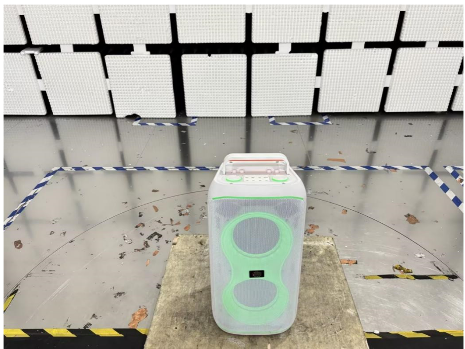
Radiation Emission Test Setup (close-up)
