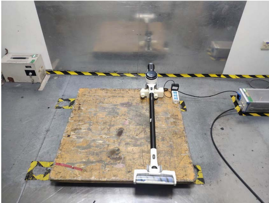
Test setup Conducted Emission
