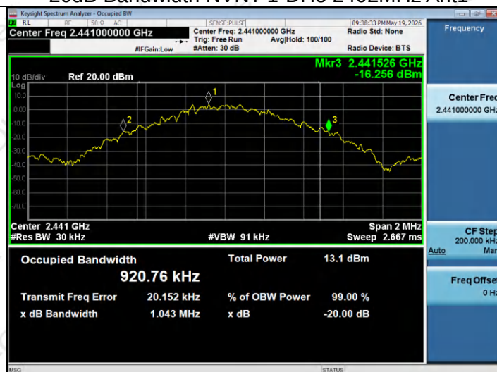
-20dB Bandwidth NVNT 1-DH5 2441MHz Ant1
