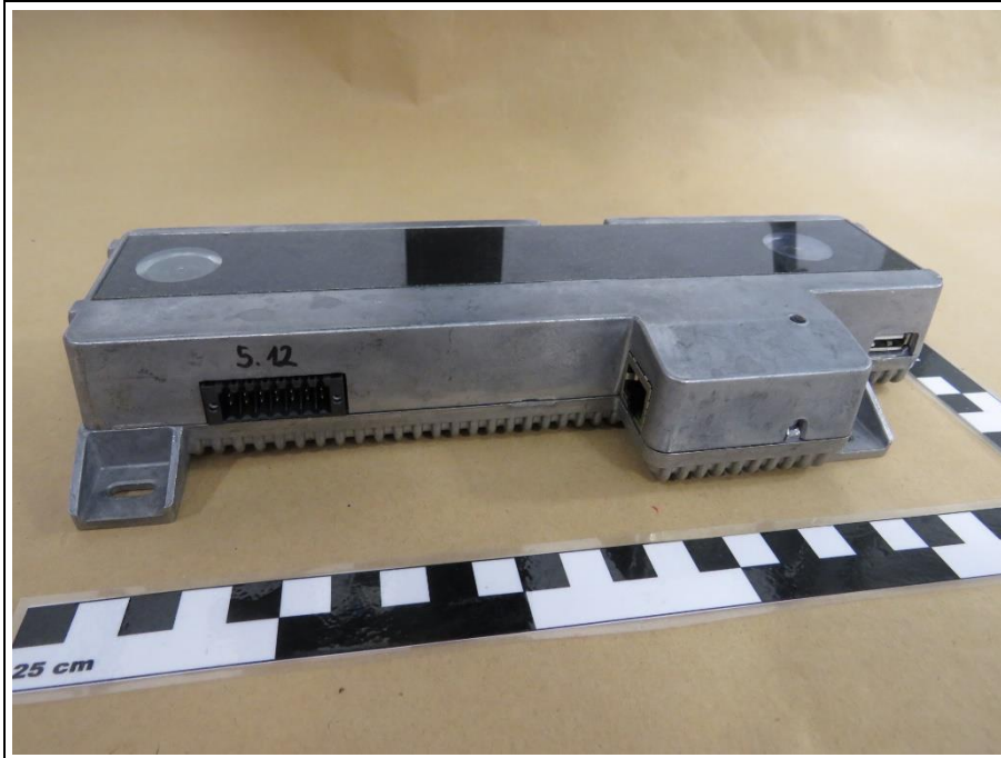
EUT SIDE WITH ETHERNET, USB AND I/O SOCKET
