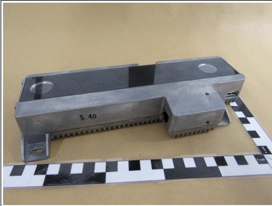
EUT SIDE WITH ETHERNET AND USB SOCKET
