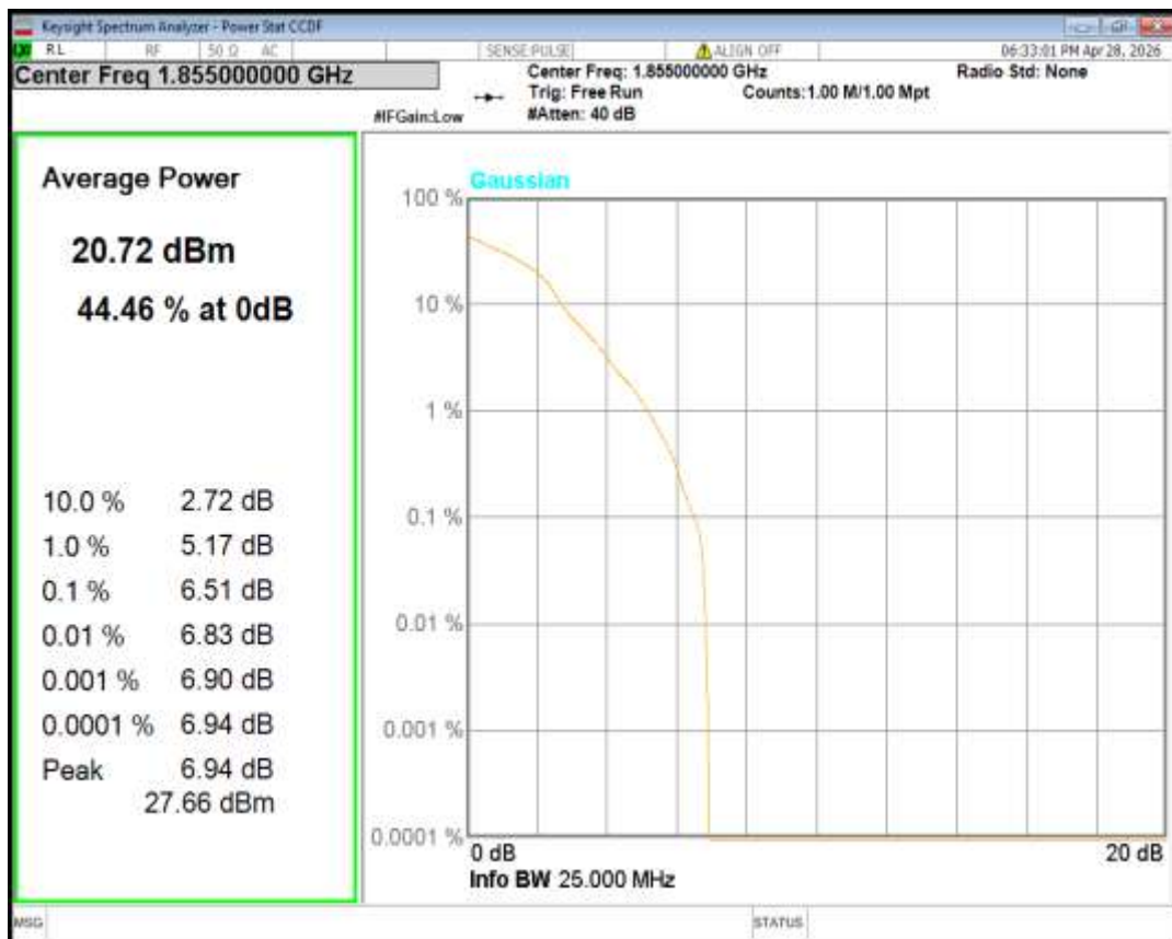
Band2 16QAM BW=10MHz Channel=18900 RB Size=1 Position=#0
