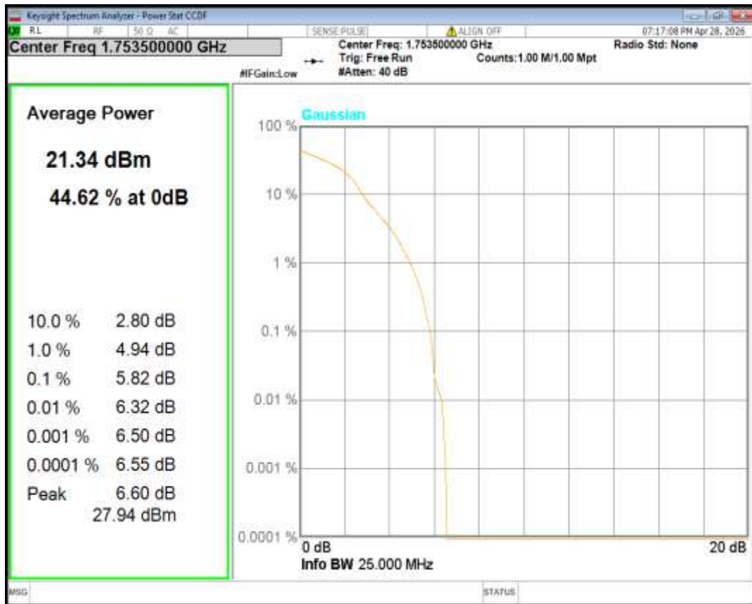
Band4 16QAM BW=5MHz Channel=19975 RB Size=1 Position=#0
