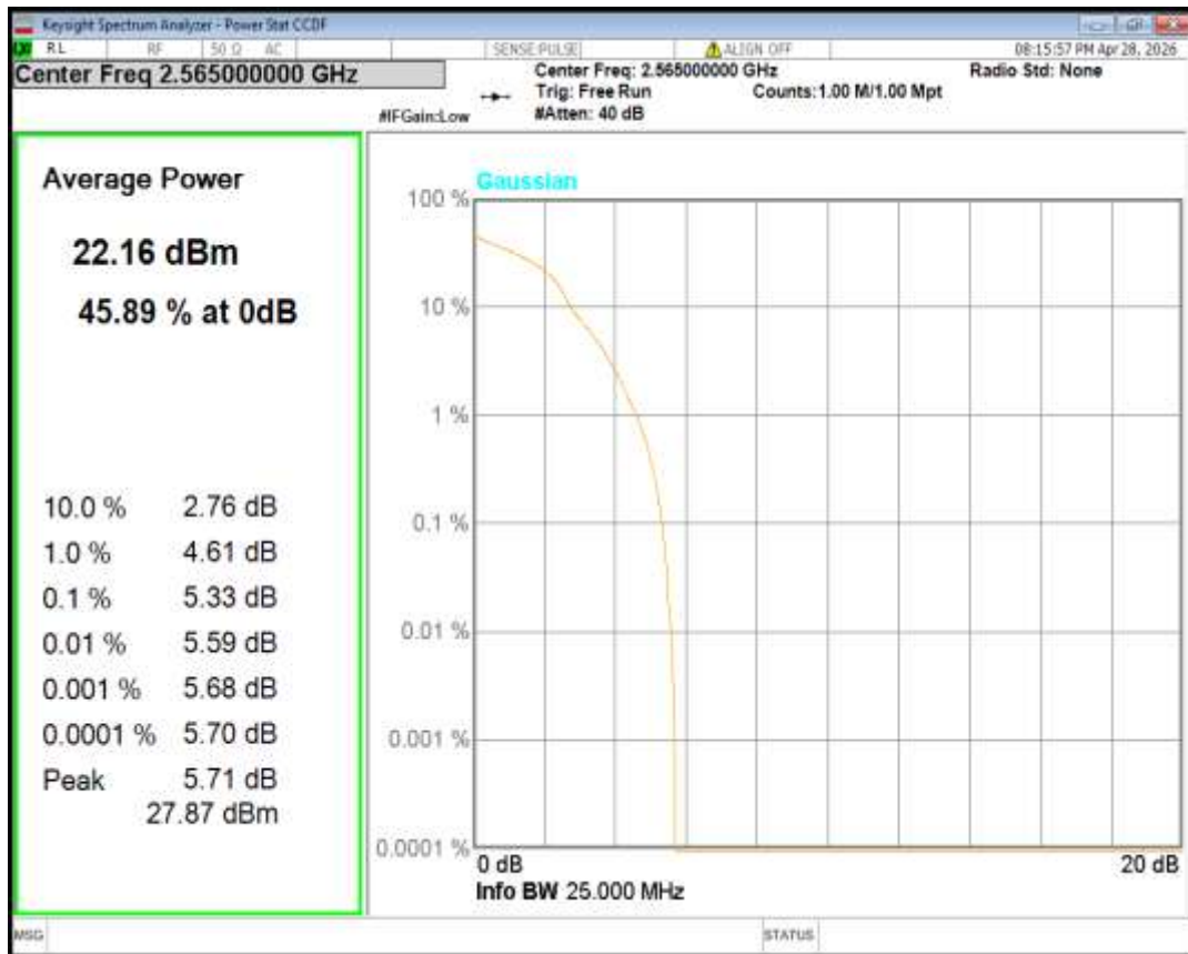
Band7 16QAM BW=15MHz Channel=20825 RB Size=1 Position=#0
