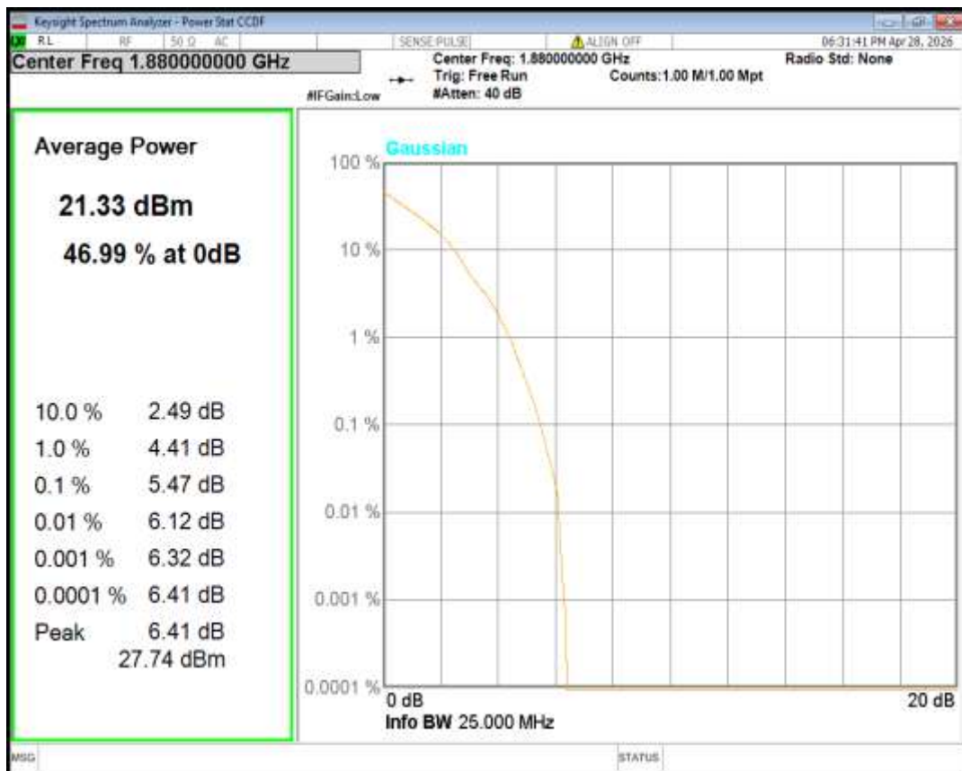
Band2 QPSK BW=10MHz Channel=18900 RB Size=1 Position=#0
