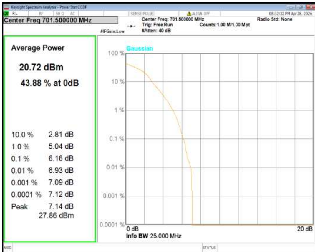
Band12 16QAM BW=5MHz Channel=23095 RB Size=1 Position=#0
