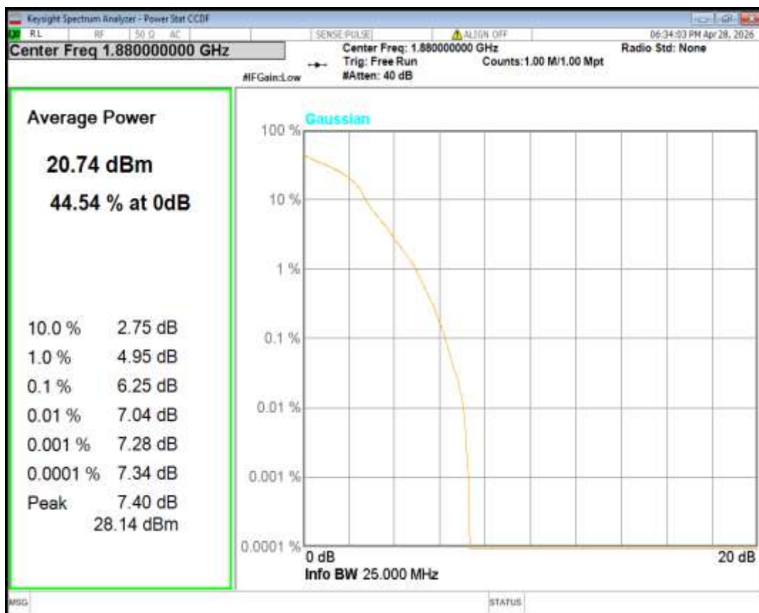
Band2 16QAM BW=20MHz Channel=18700 RB Size=1 Position=#0
