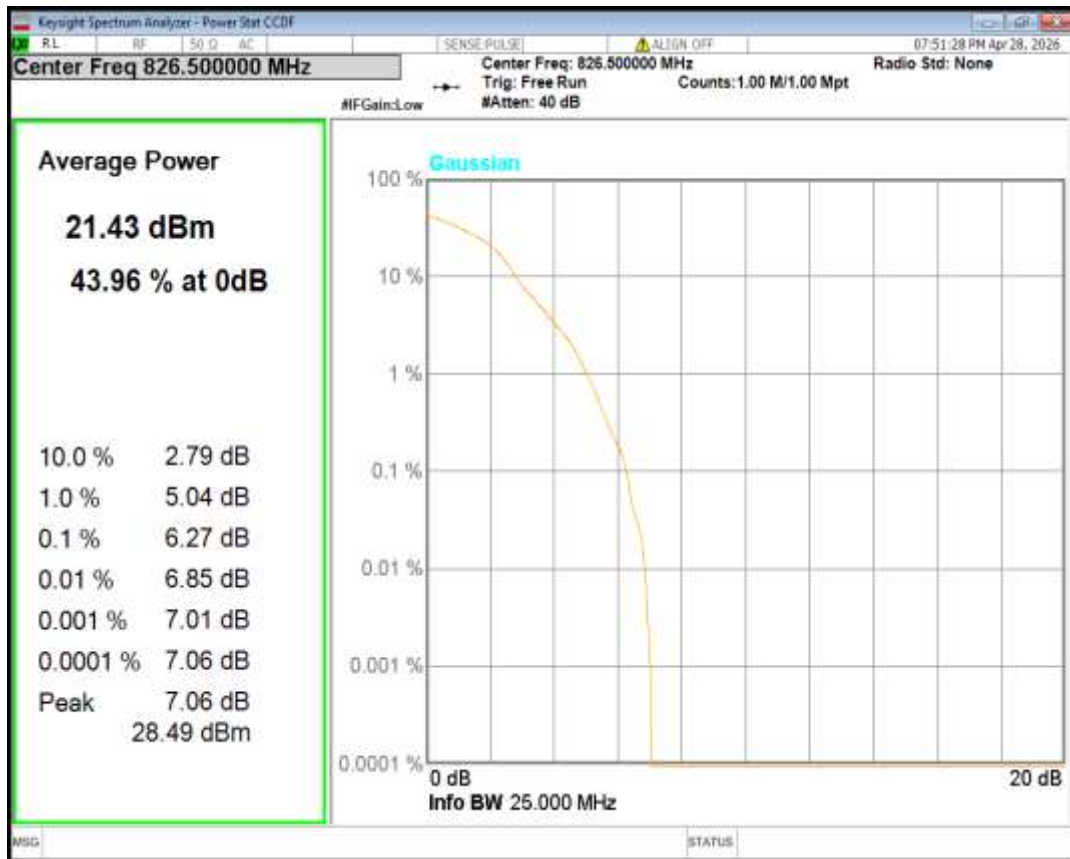
Band5 QPSK BW=1.4MHz Channel=20525 RB Size=1 Position=#0
