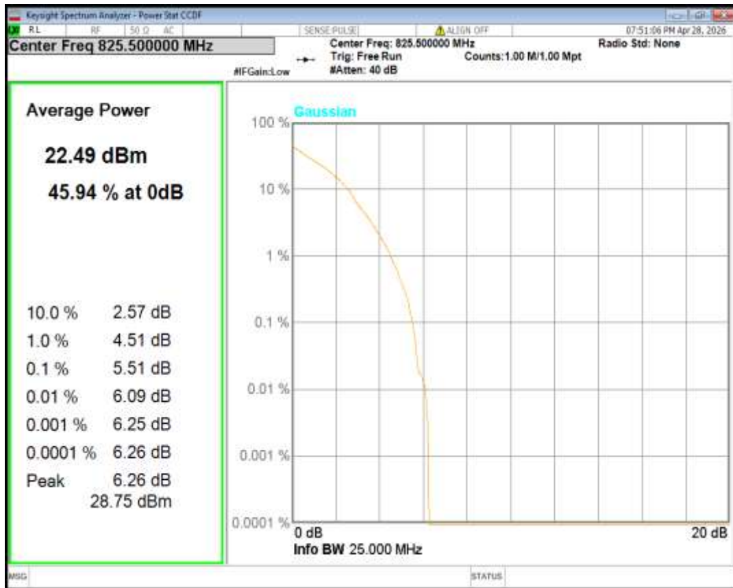
Band5 QPSK BW=3MHz Channel=20525 RB Size=1 Position=#0
