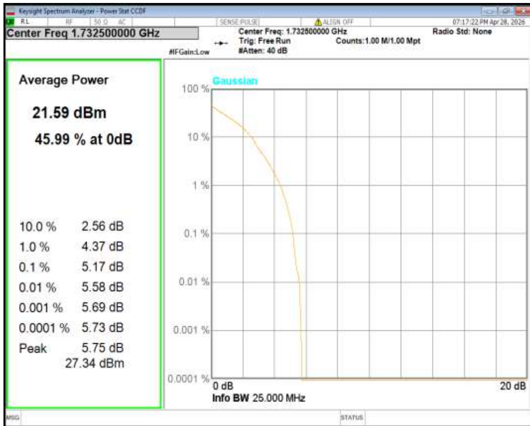
Band4 QPSK BW=5MHz Channel=20375 RB Size=1 Position=#0
