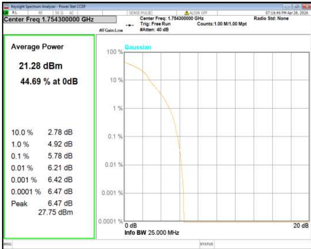
Band4 16QAM BW=10MHz Channel=20000 RB Size=1 Position=#0
