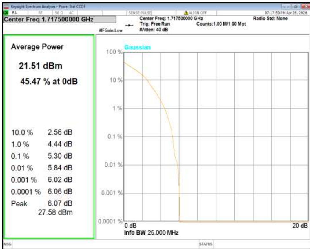
Band4 QPSK BW=20MHz Channel=20300 RB Size=1 Position=#0
