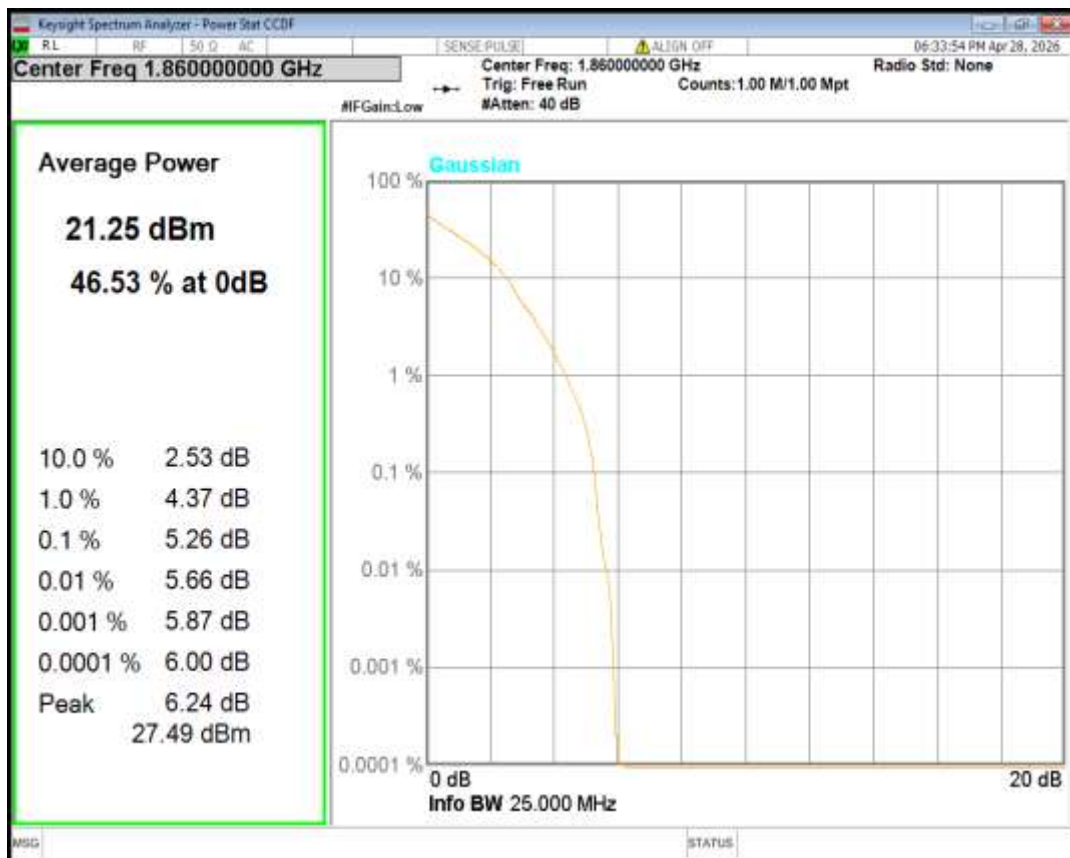
Band2 QPSK BW=20MHz Channel=18900 RB Size=1 Position=#0
