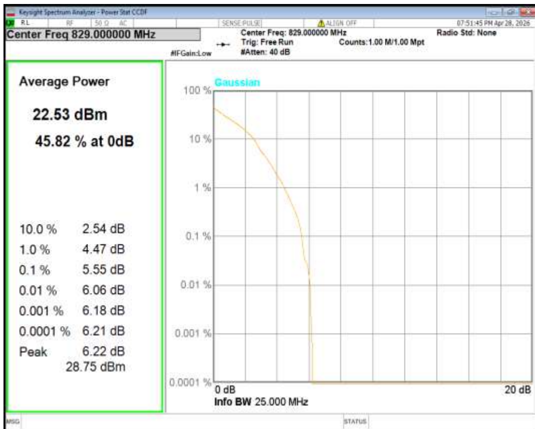
Band5 QPSK BW=10MHz Channel=20525 RB Size=1 Position=#0
