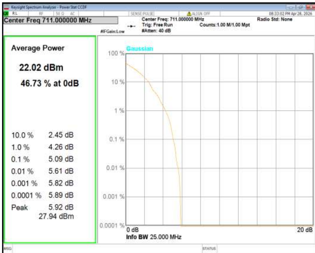
Band12 QPSK BW=3MHz Channel=23025 RB Size=1 Position=#0
