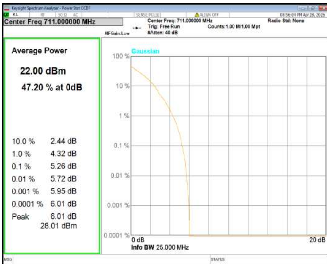
Band17 QPSK BW=5MHz Channel=23755 RB Size=1 Position=#0
