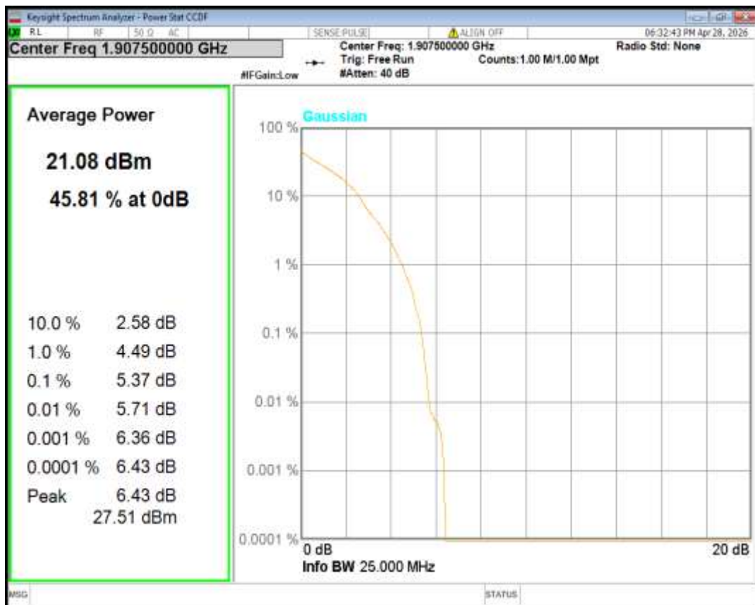
Band4 16QAM BW=1.4MHz Channel=19957 RB Size=1 Position=#0
