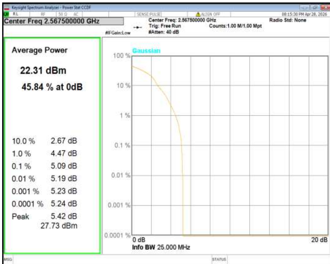
Band7 QPSK BW=10MHz Channel=20800 RB Size=1 Position=#0
