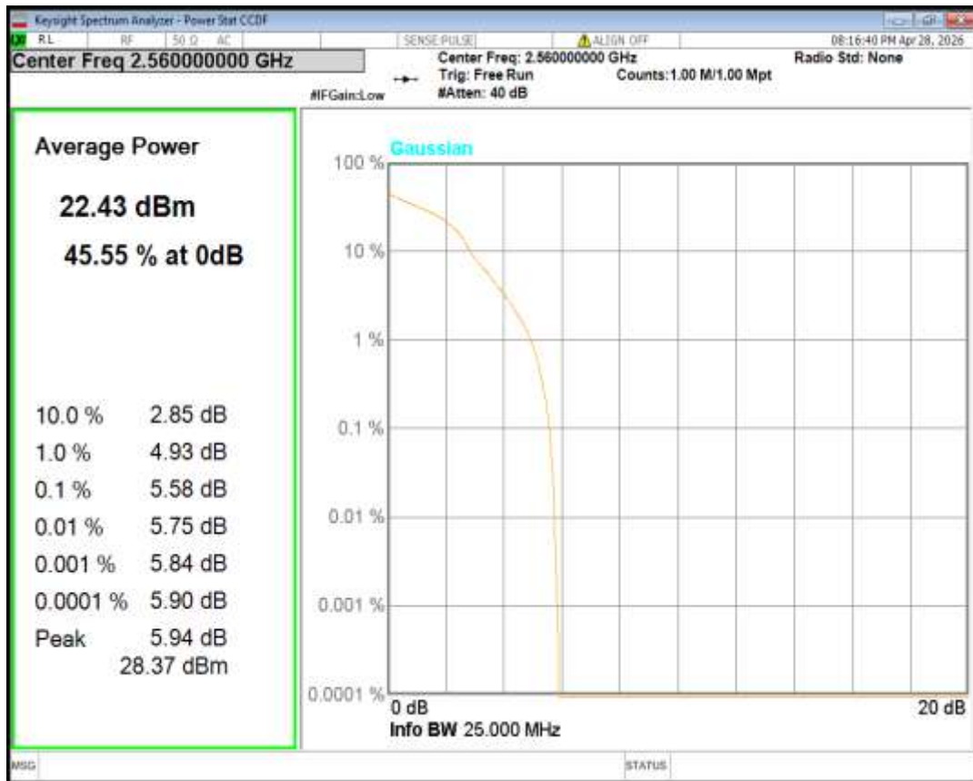
Band7 16QAM BW=5MHz Channel=20775 RB Size=1 Position=#0
