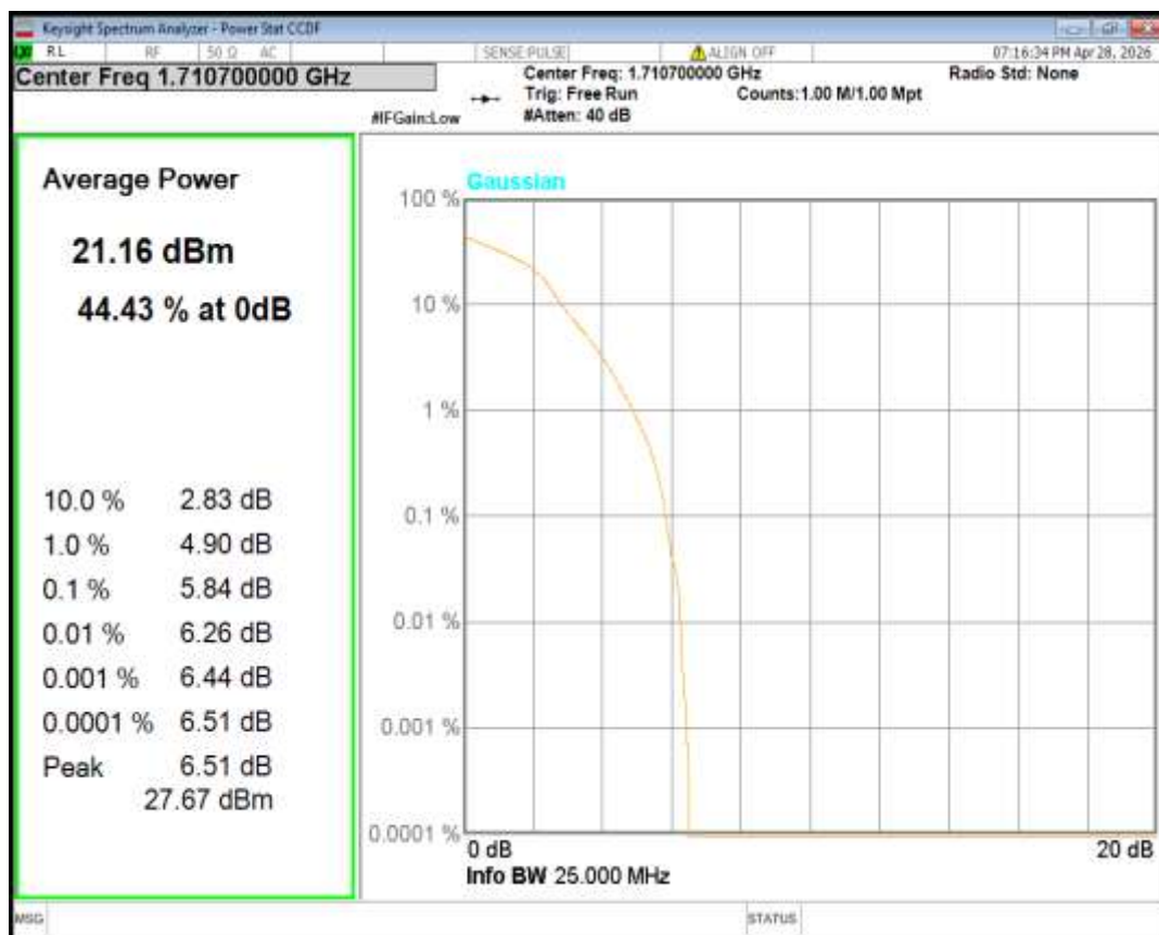
Band4 16QAM BW=1.4MHz Channel=20175 RB Size=1 Position=#0
