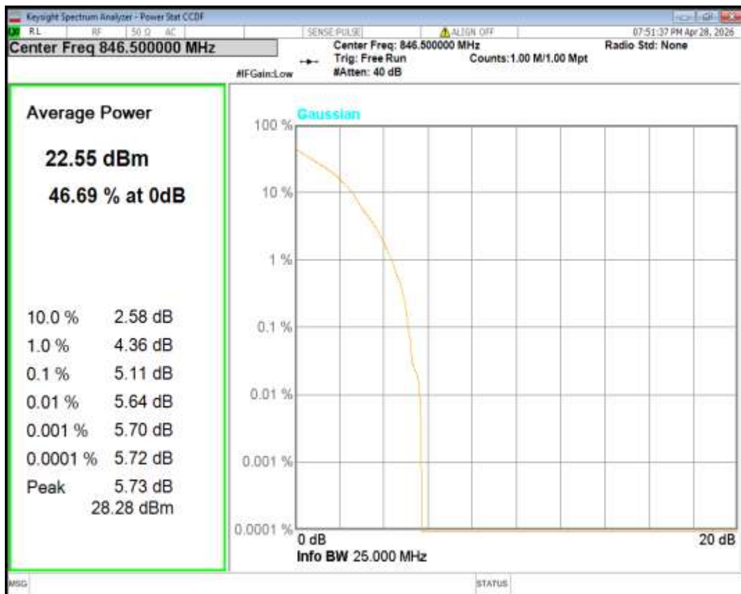
Band7 16QAM BW=10MHz Channel=20800 RB Size=1 Position=#0
