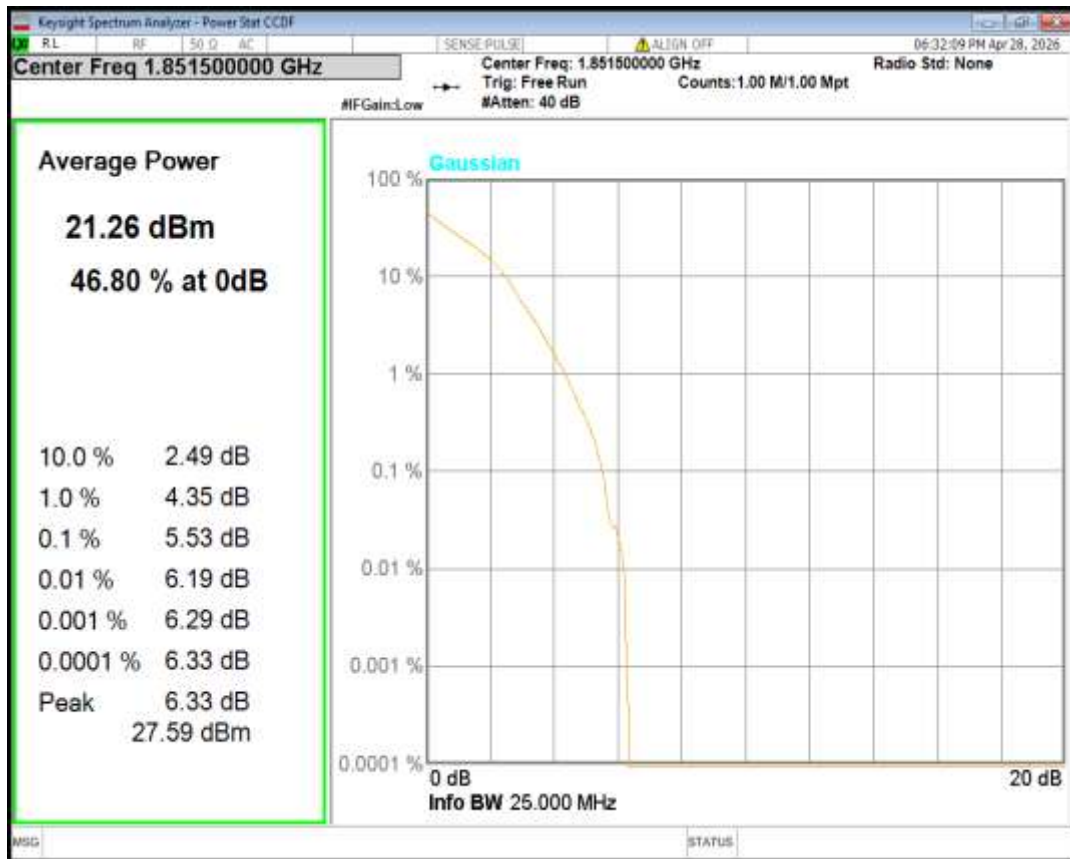
Band2 QPSK BW=5MHz Channel=18900 RB Size=1 Position=#0
