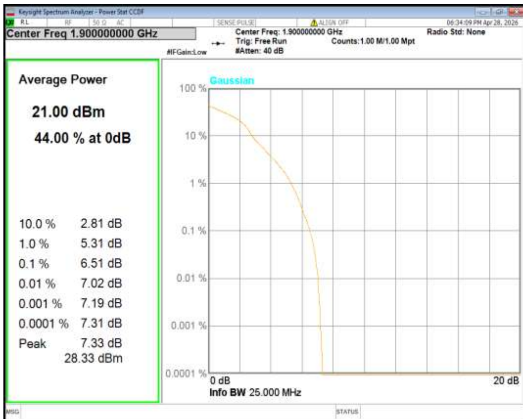
Band2 16QAM BW=20MHz Channel=18900 RB Size=1 Position=#0
