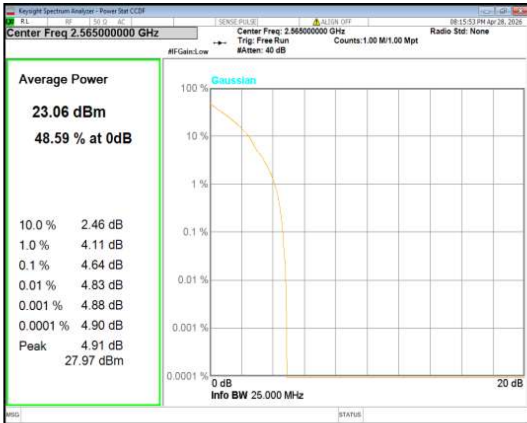
Band7 QPSK BW=15MHz Channel=20825 RB Size=1 Position=#0
