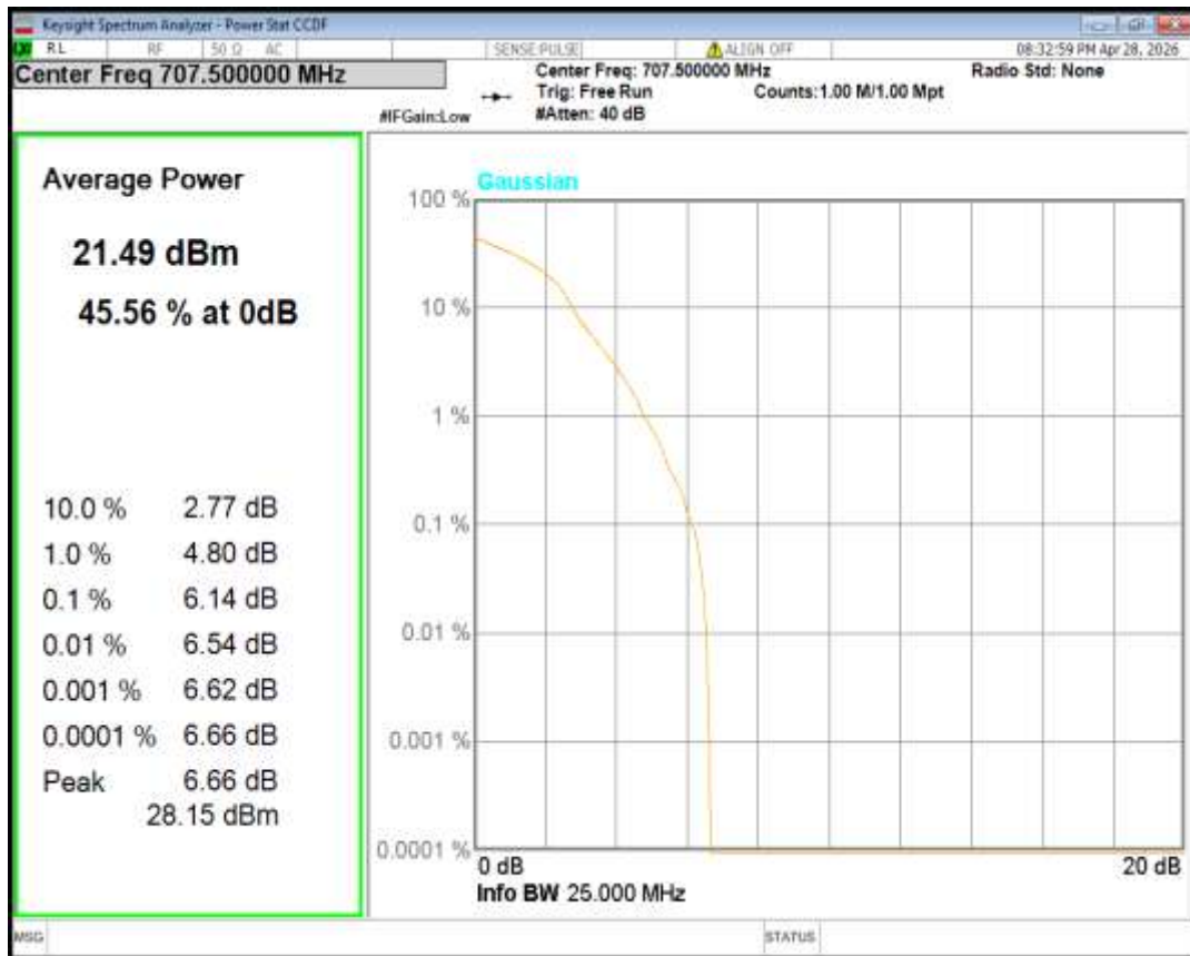
Band12 16QAM BW=10MHz Channel=23130 RB Size=1 Position=#0
