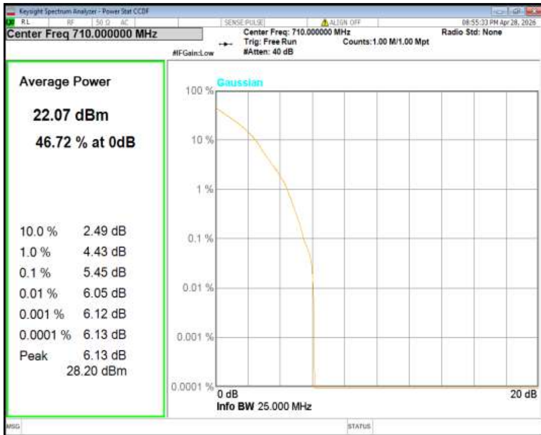
Band17 QPSK BW=5MHz Channel=23825 RB Size=1 Position=#0
