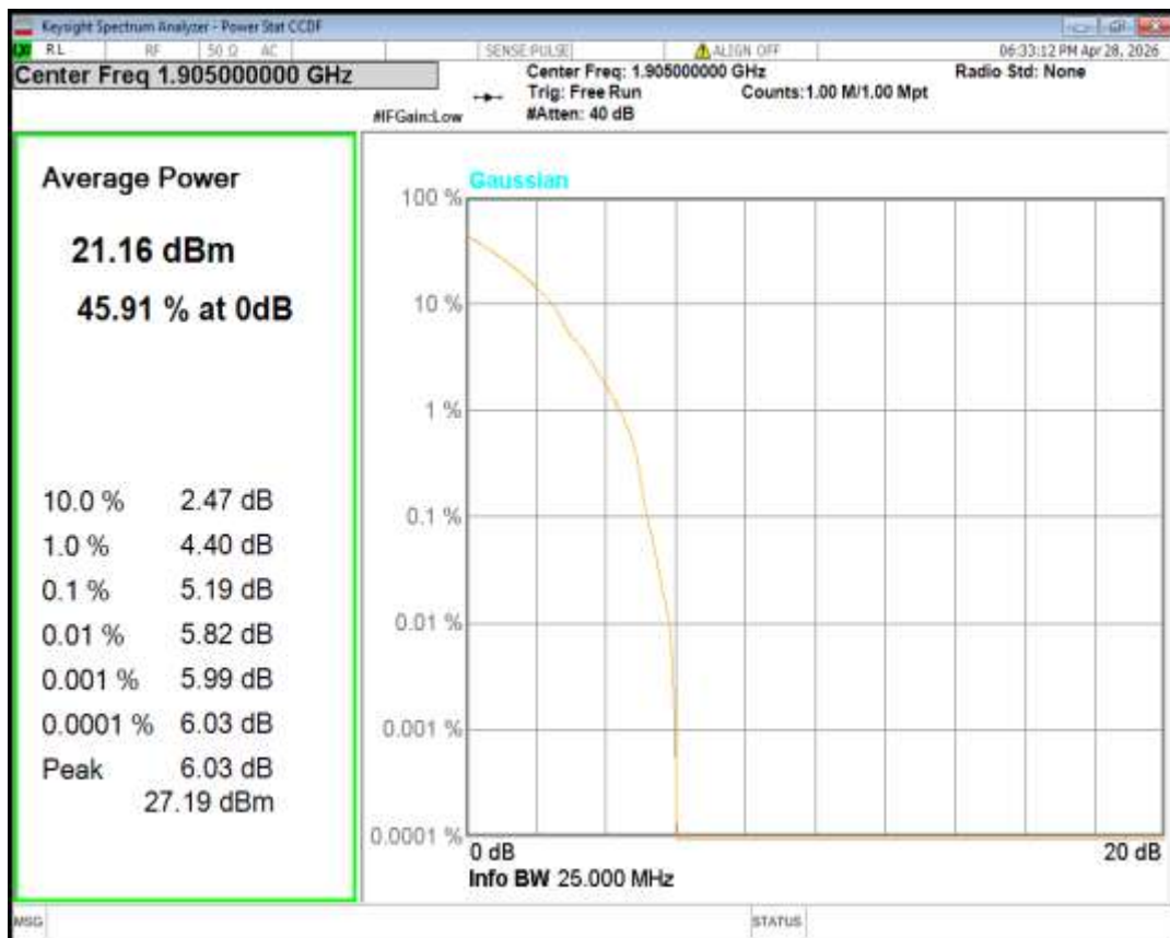
Band2 QPSK BW=15MHz Channel=18675 RB Size=1 Position=#0
