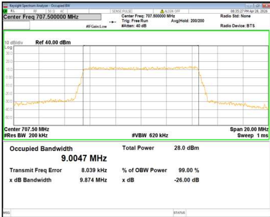
Band12 16QAM BW=10MHz Channel=23130 RB Size=50 Position=#0
