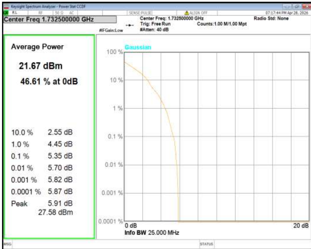
Band4 QPSK BW=10MHz Channel=20350 RB Size=1 Position=#0
