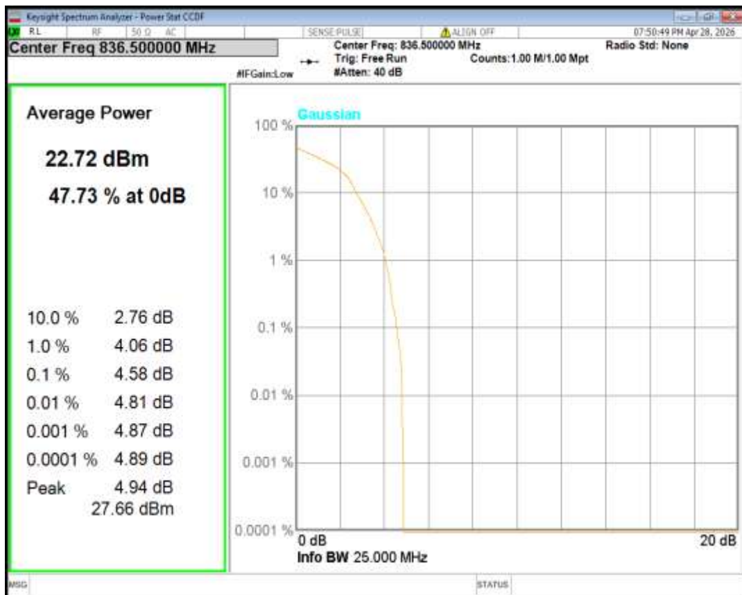
Band5 16QAM BW=1.4MHz Channel=20643 RB Size=1 Position=#0
