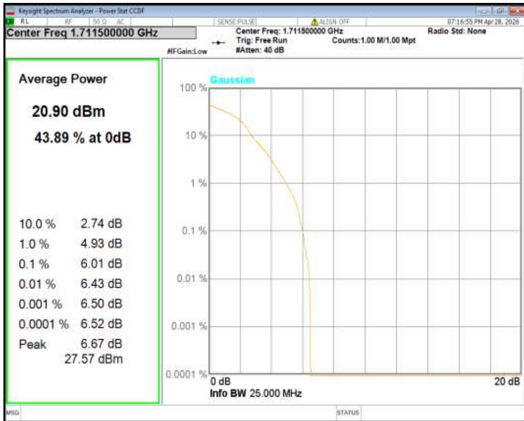
Band4 16QAM BW=3MHz Channel=20175 RB Size=1 Position=#0
