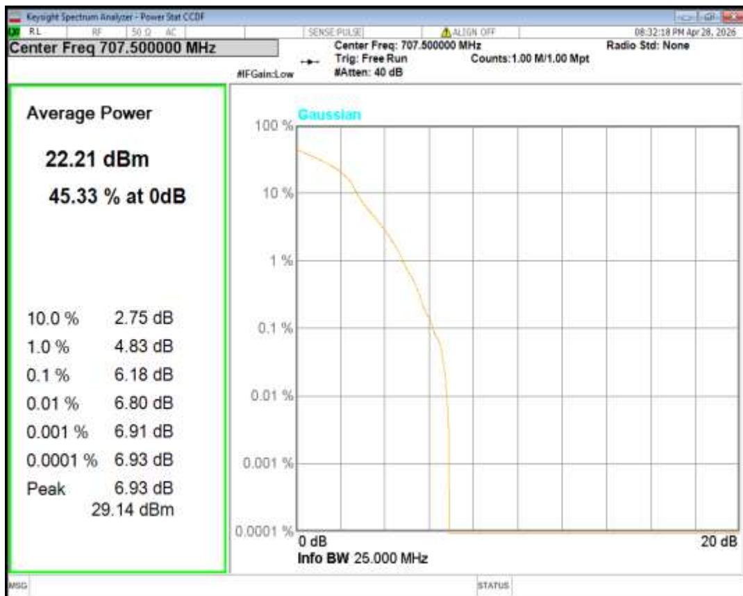
Band12 16QAM BW=3MHz Channel=23165 RB Size=1 Position=#0
