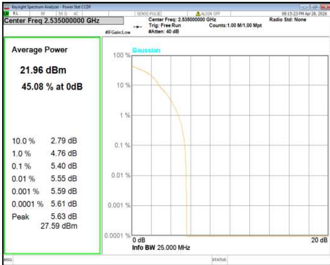
Band7 16QAM BW=5MHz Channel=21425 RB Size=1 Position=#0
