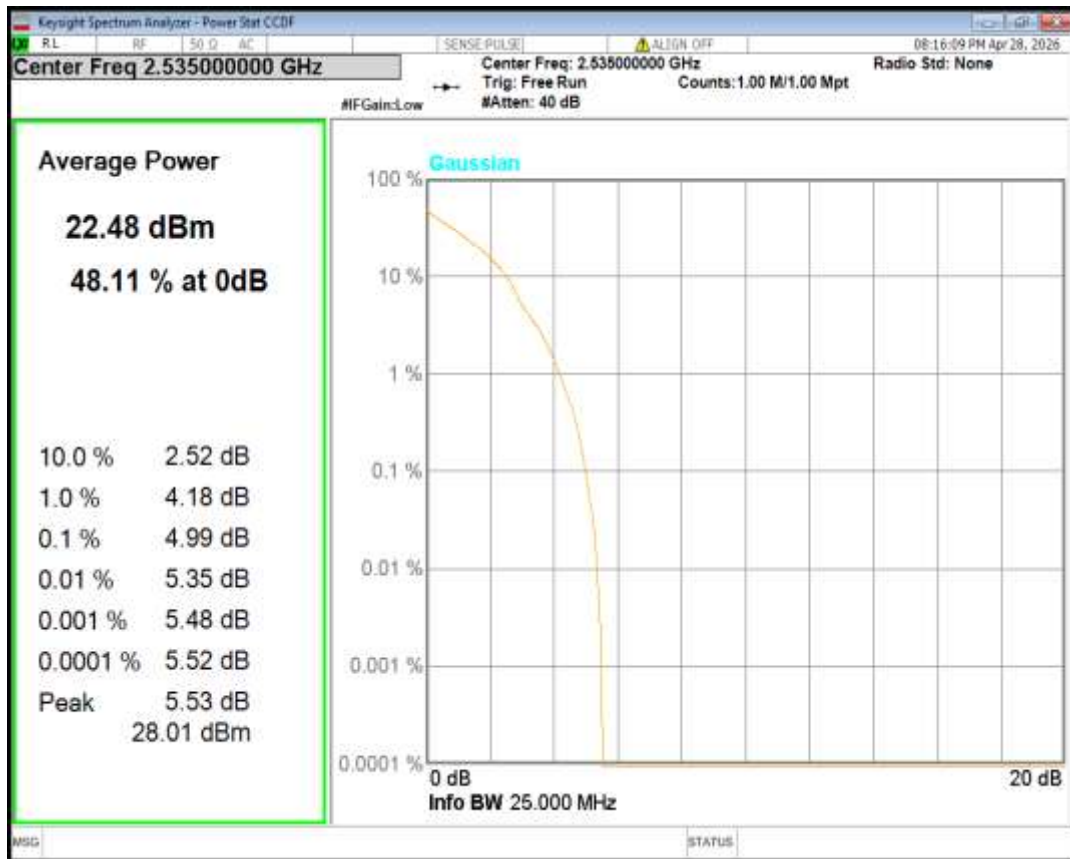
Band7 QPSK BW=15MHz Channel=21375 RB Size=1 Position=#0
