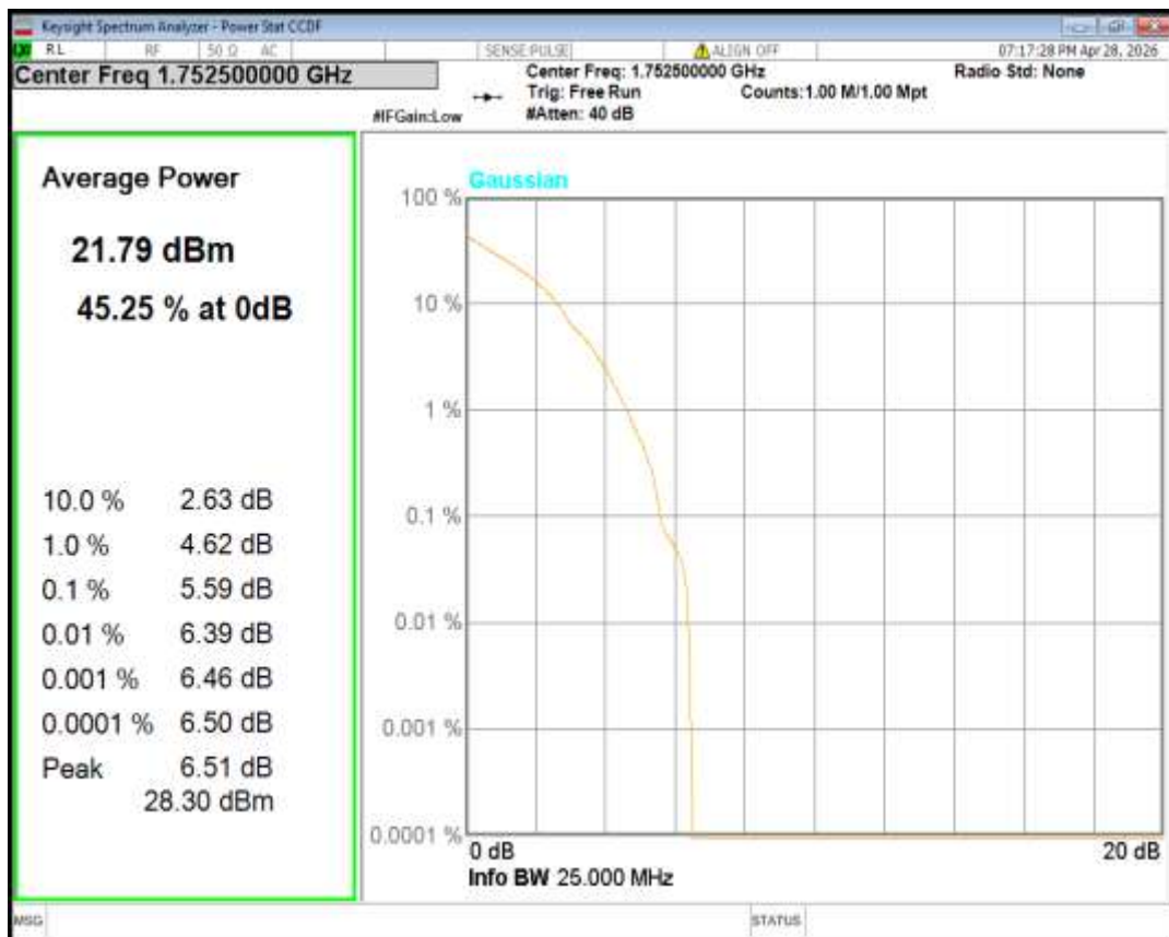
Band5 16QAM BW=1.4MHz Channel=20407 RB Size=1 Position=#0
