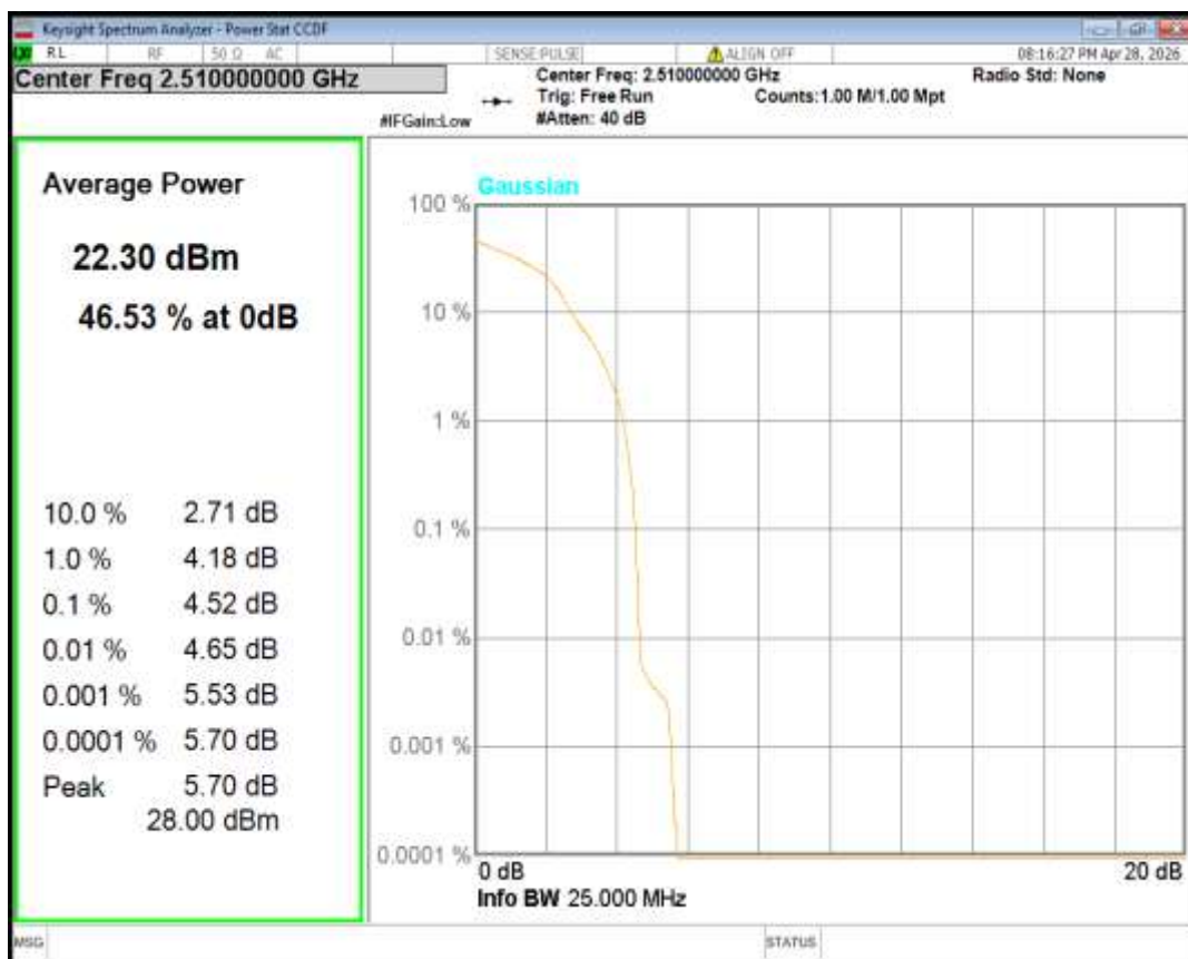
Band7 16QAM BW=20MHz Channel=21100 RB Size=1 Position=#0
