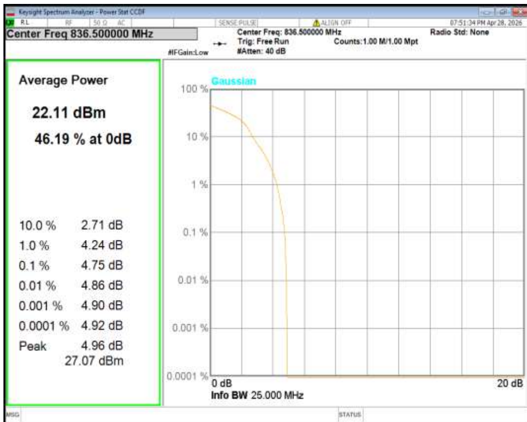
Band5 16QAM BW=5MHz Channel=20625 RB Size=1 Position=#0
