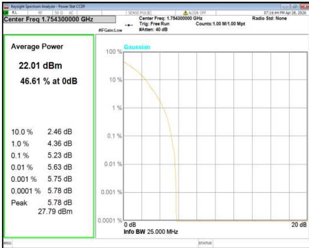
Band4 QPSK BW=10MHz Channel=20000 RB Size=1 Position=#0
