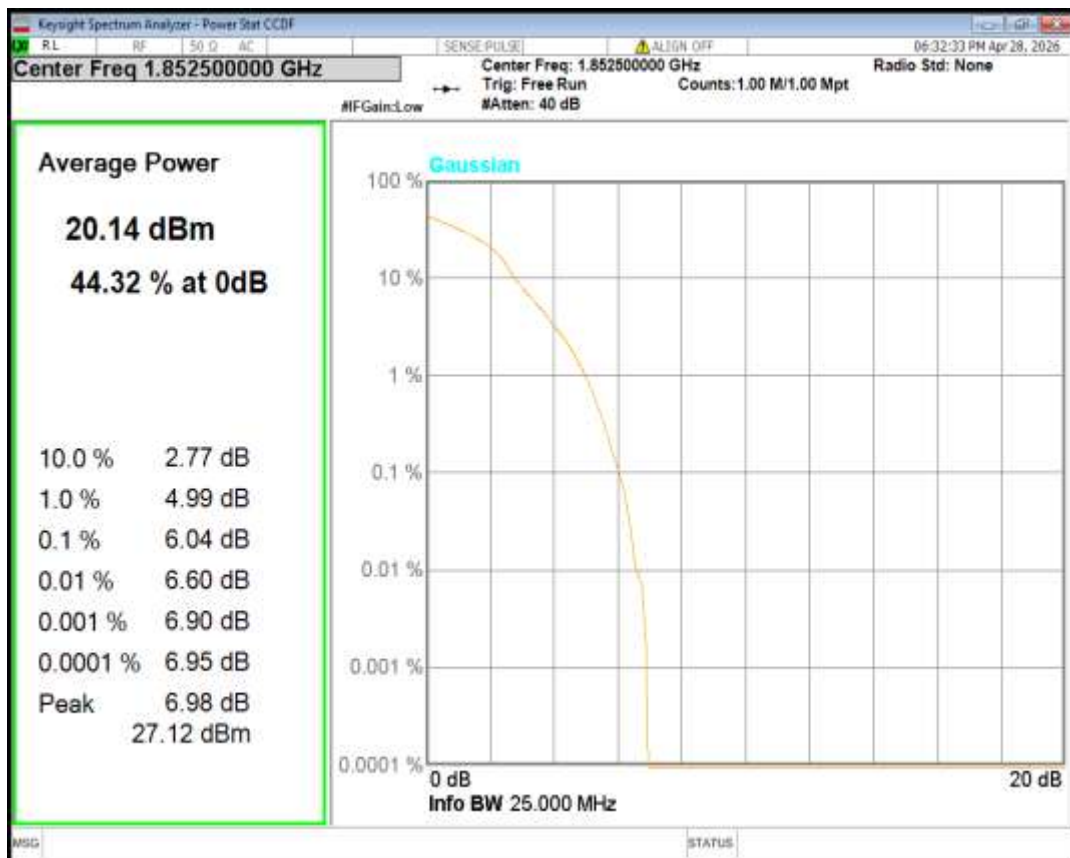
Band2 16QAM BW=5MHz Channel=18900 RB Size=1 Position=#0
