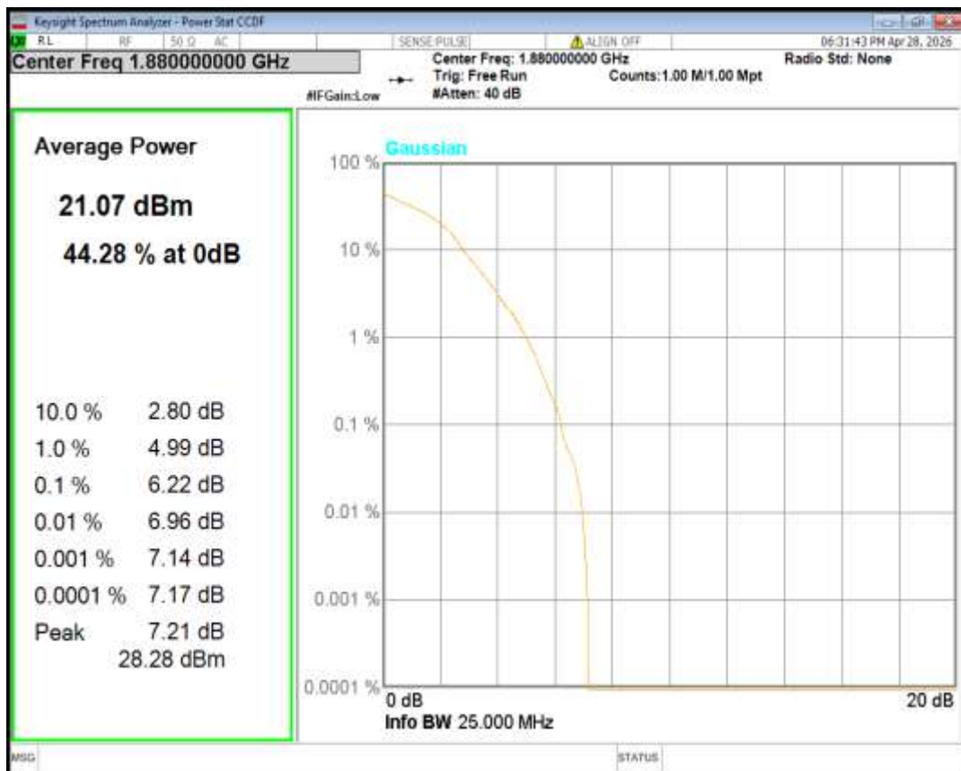
Band2 16QAM BW=1.4MHz Channel=19193 RB Size=1 Position=#0
