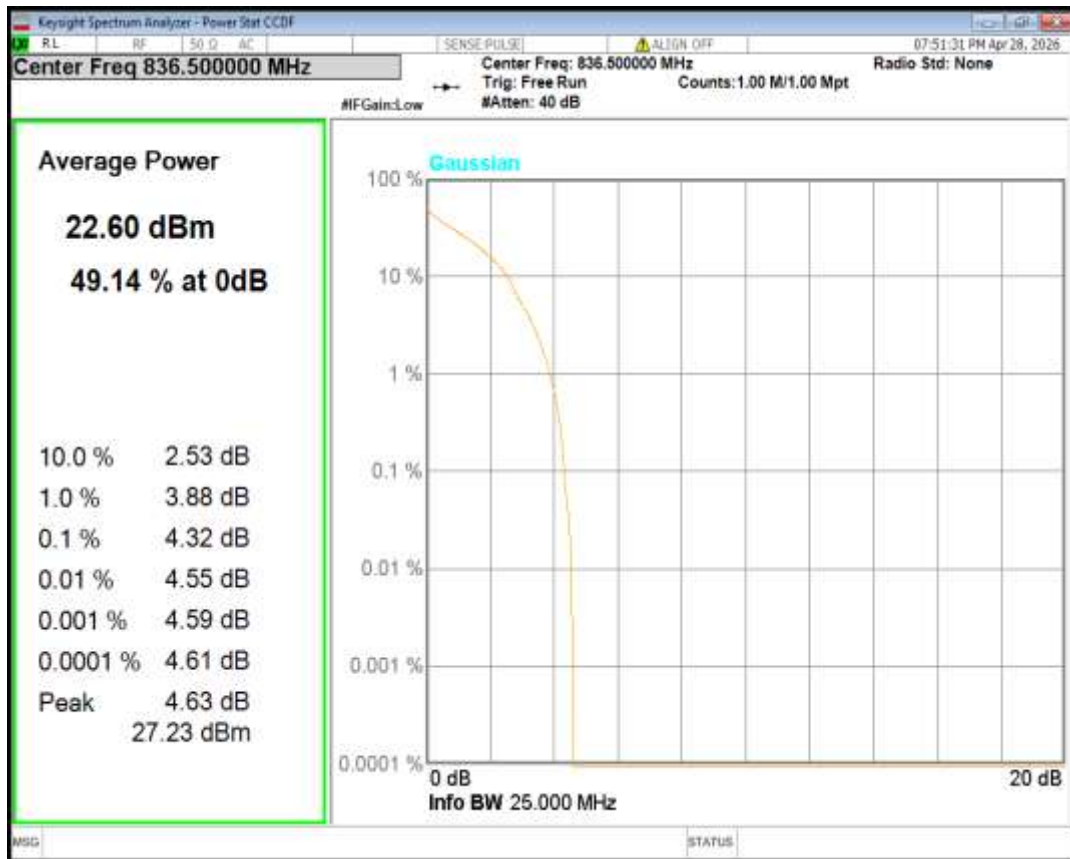
Band5 QPSK BW=5MHz Channel=20625 RB Size=1 Position=#0
