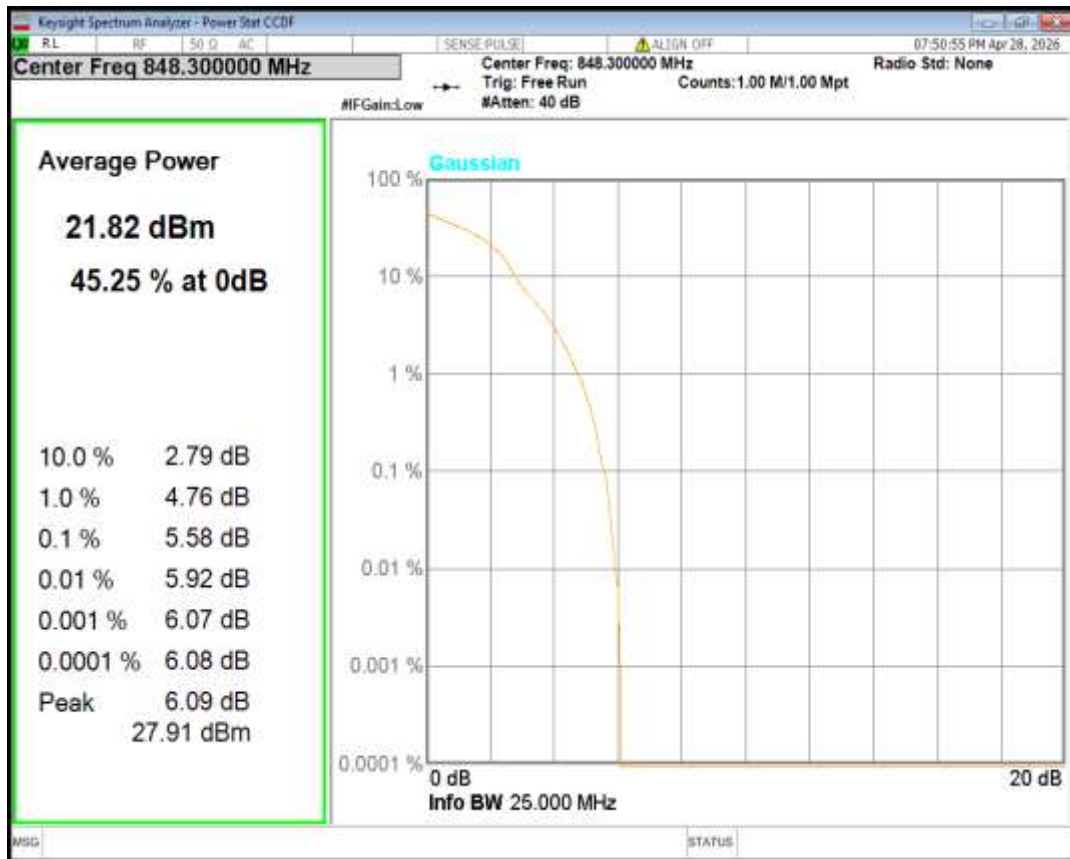
Band5 16QAM BW=10MHz Channel=20450 RB Size=1 Position=#0
