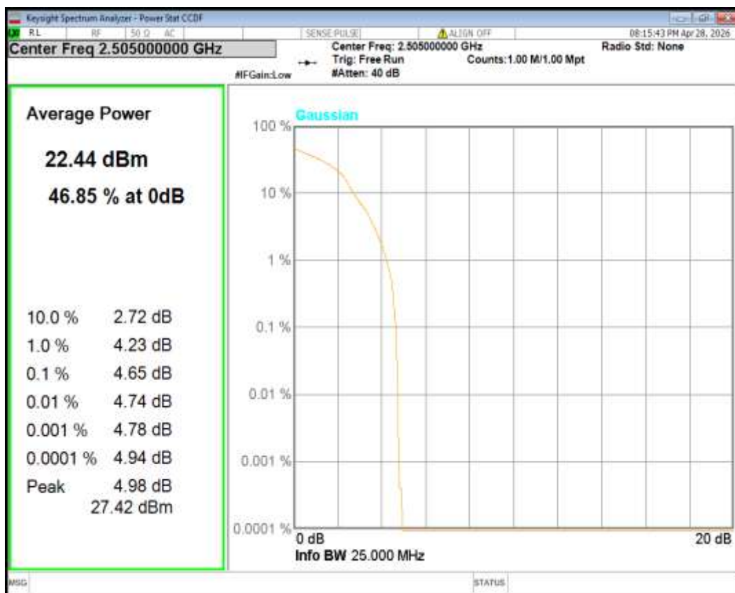
Band7 16QAM BW=10MHz Channel=21100 RB Size=1 Position=#0
