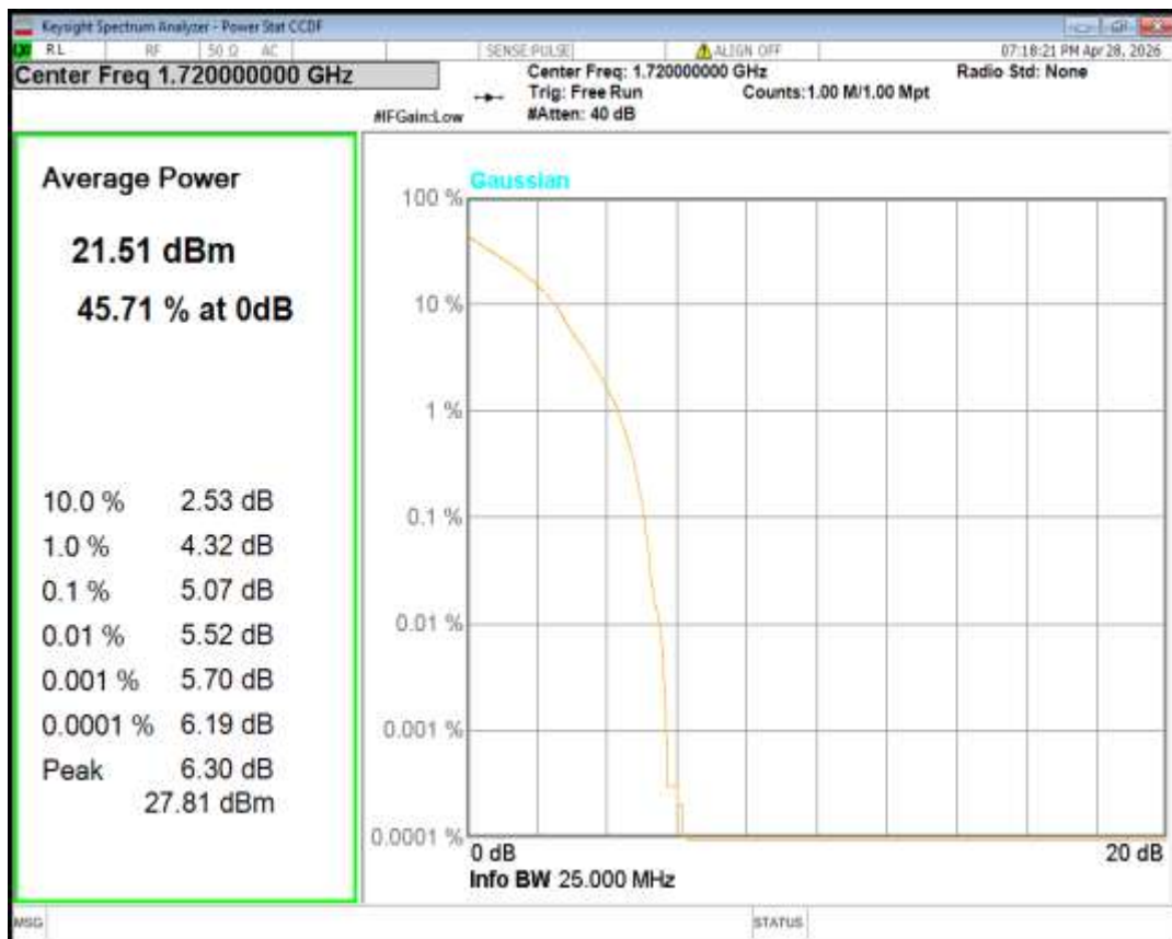
Band4 QPSK BW=15MHz Channel=20325 RB Size=1 Position=#0
