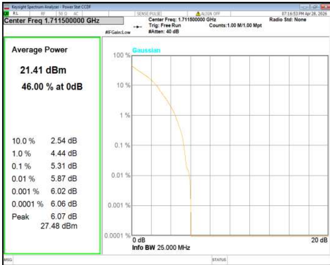
Band4 QPSK BW=3MHz Channel=20175 RB Size=1 Position=#0
