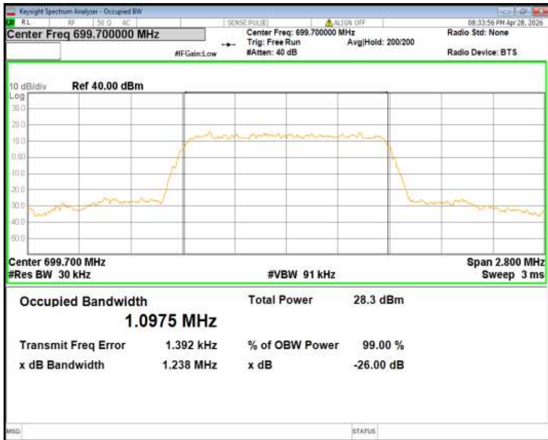
Band12 16QAM BW=1.4MHz Channel=23095 RB Size=6 Position=#0
