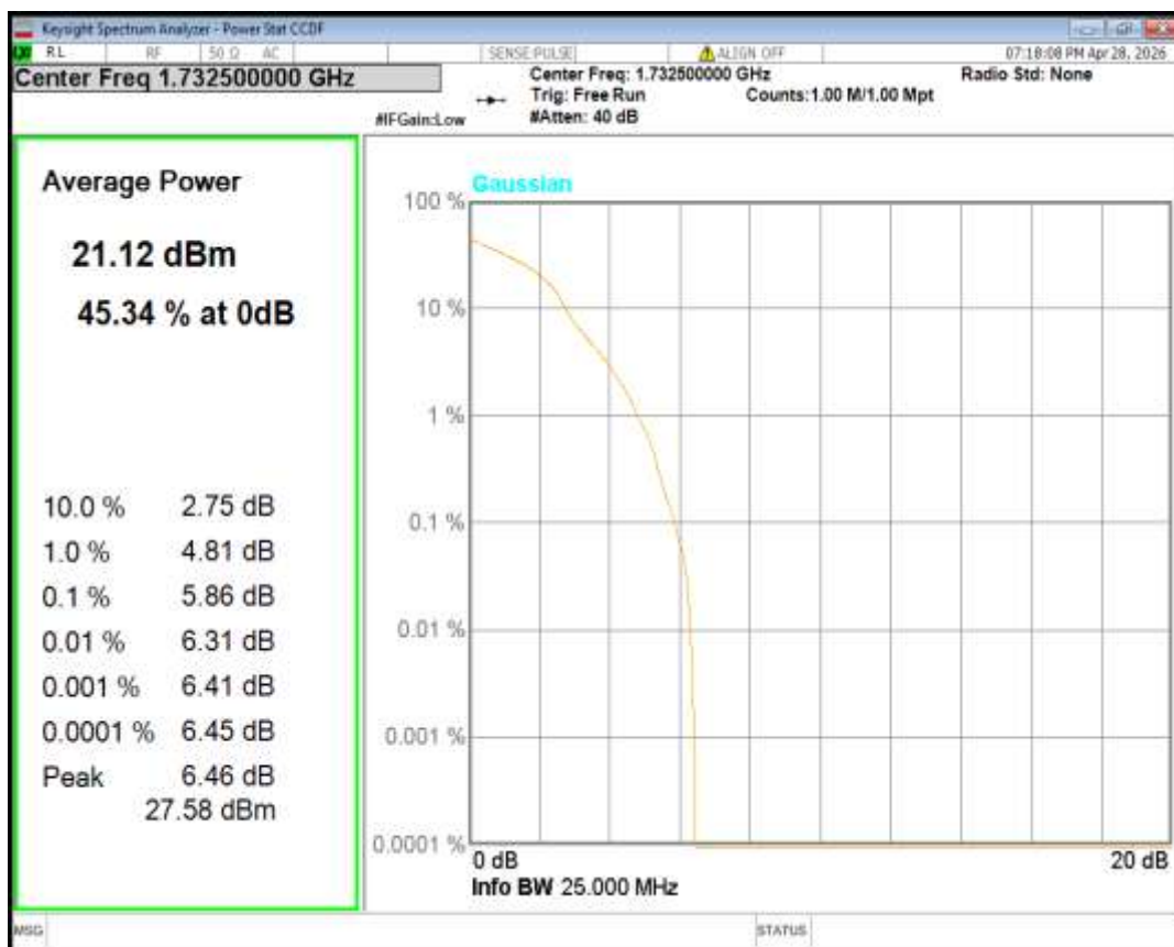
Band4 16QAM BW=15MHz Channel=20025 RB Size=1 Position=#0
