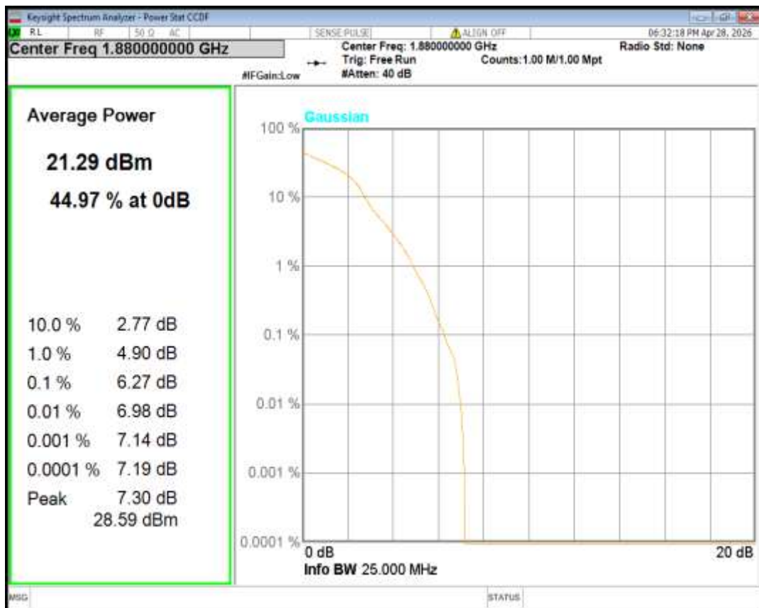
Band2 16QAM BW=3MHz Channel=19185 RB Size=1 Position=#0
