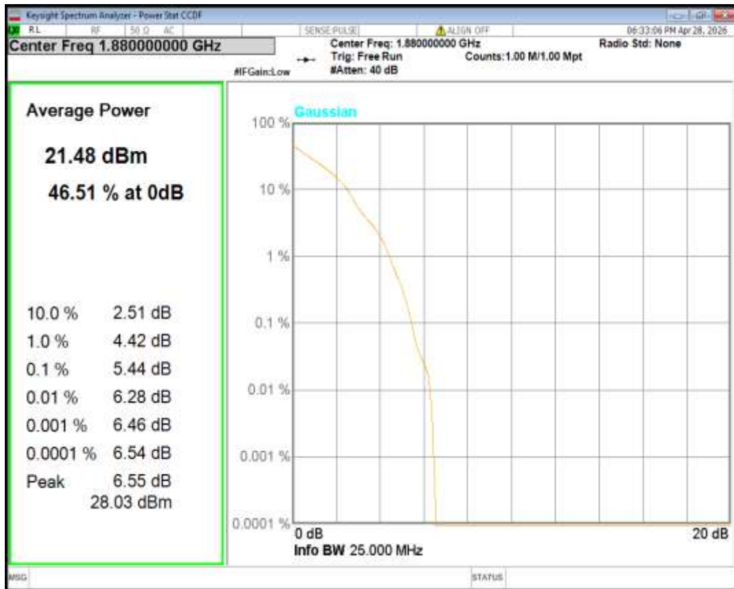
Band2 QPSK BW=10MHz Channel=19150 RB Size=1 Position=#0
