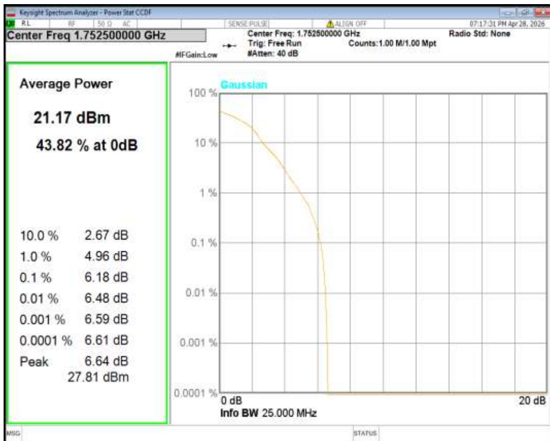
Band4 16QAM BW=5MHz Channel=20175 RB Size=1 Position=#0
