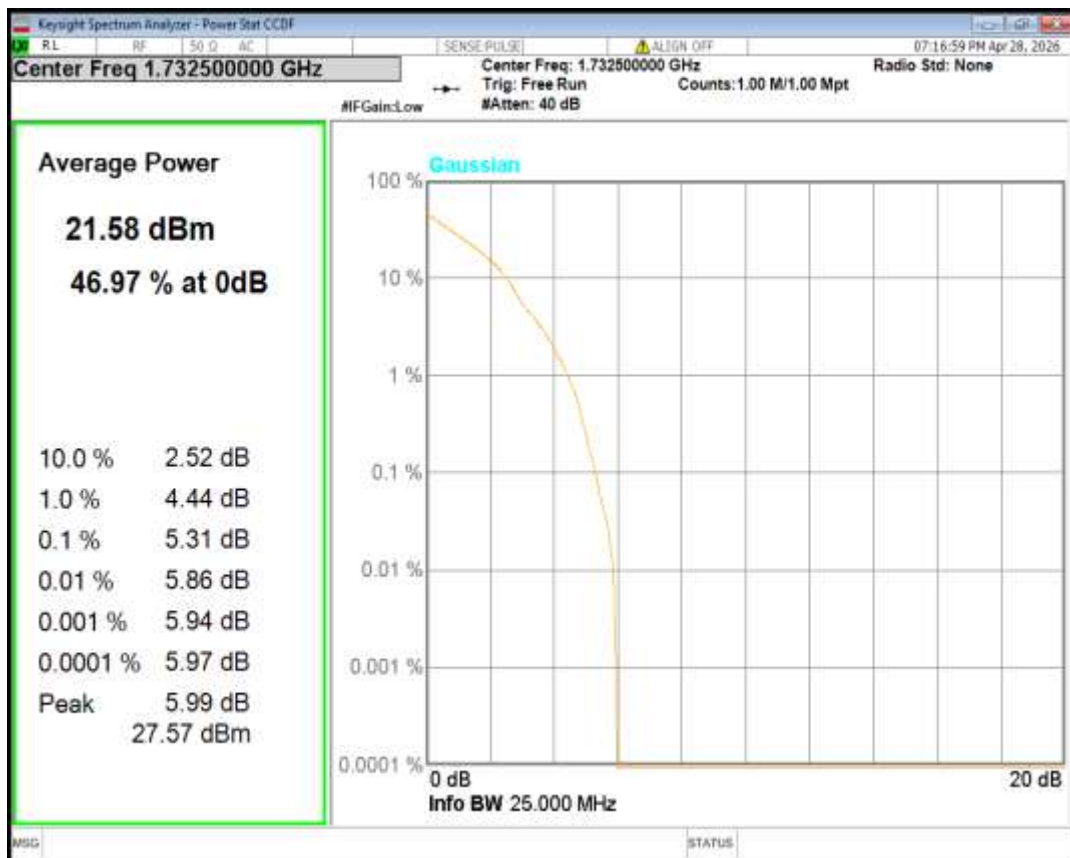
Band4 QPSK BW=3MHz Channel=20385 RB Size=1 Position=#0
