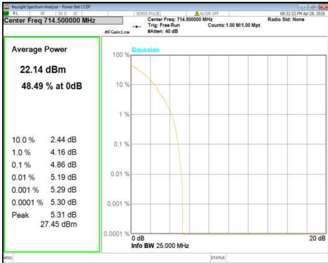
Band12 QPSK BW=5MHz Channel=23095 RB Size=1 Position=#0
