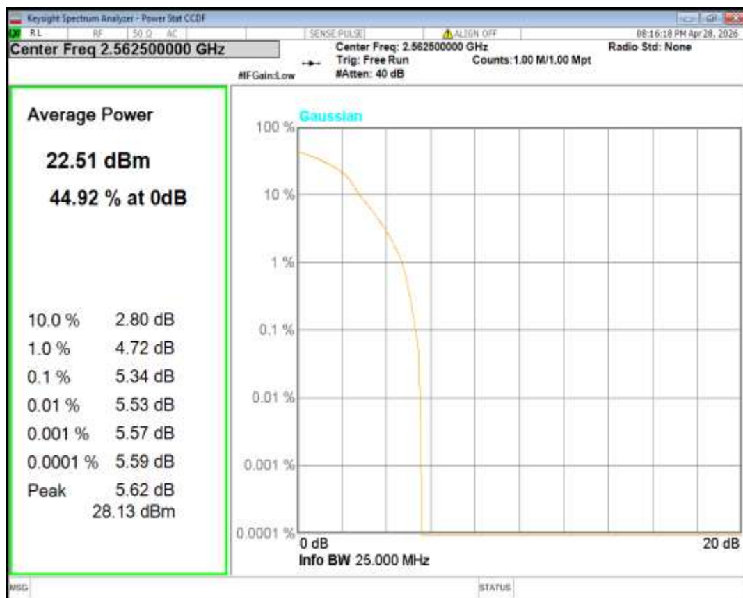
Band7 16QAM BW=20MHz Channel=20850 RB Size=1 Position=#0
