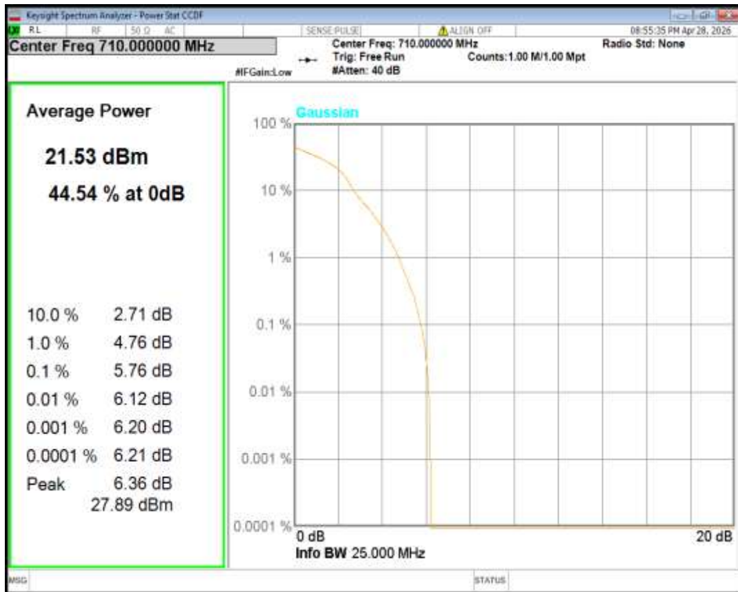
Band17 16QAM BW=5MHz Channel=23825 RB Size=1 Position=#0
