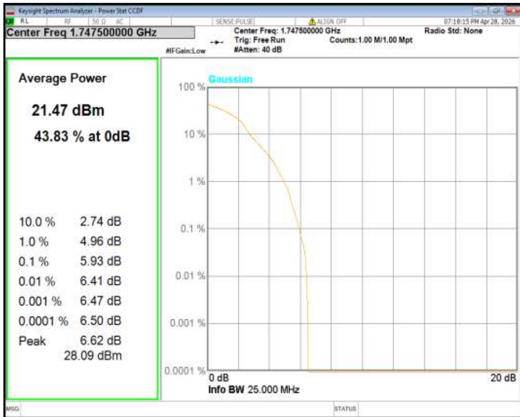
Band4 16QAM BW=10MHz Channel=20175 RB Size=1 Position=#0
