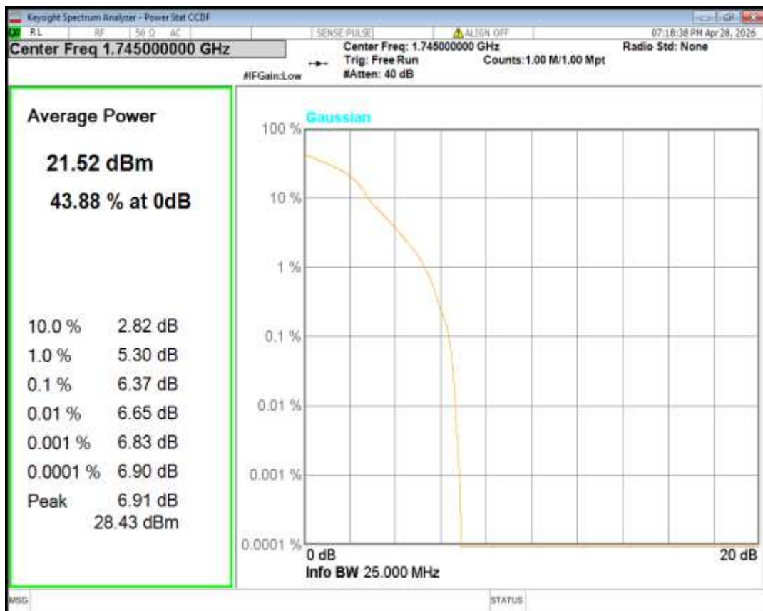
Band4 16QAM BW=3MHz Channel=19965 RB Size=1 Position=#0
