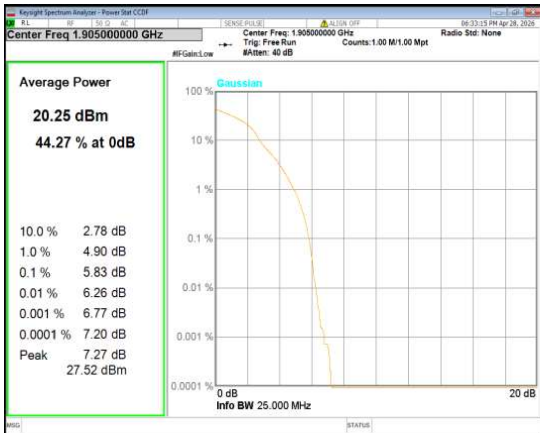
Band2 16QAM BW=15MHz Channel=18675 RB Size=1 Position=#0
