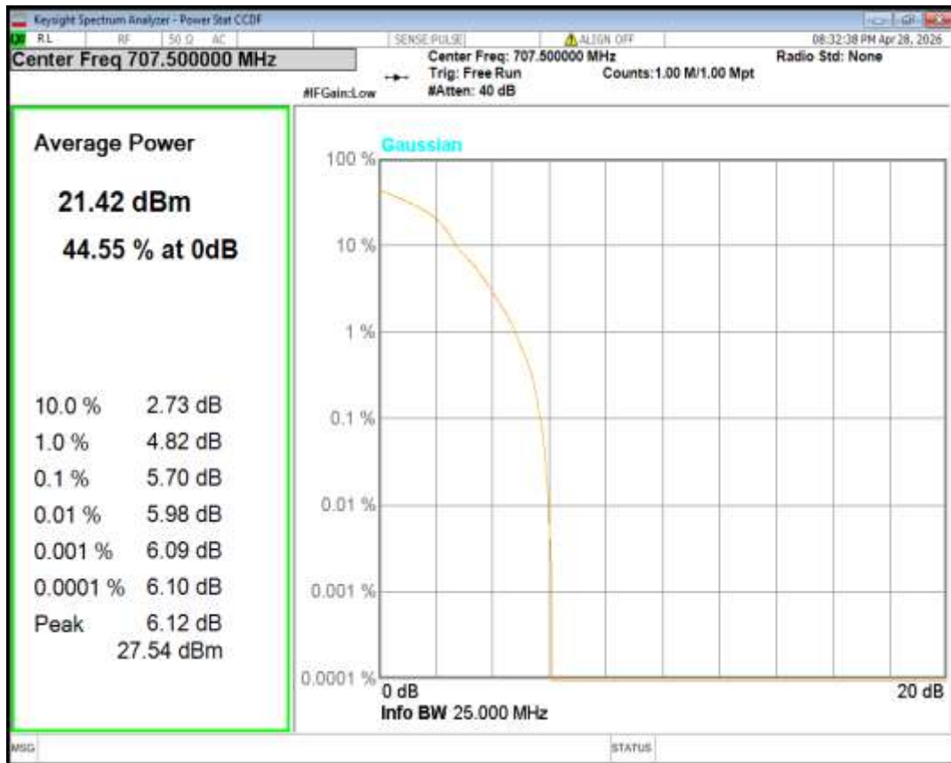
Band12 QPSK BW=10MHz Channel=23060 RB Size=1 Position=#0
