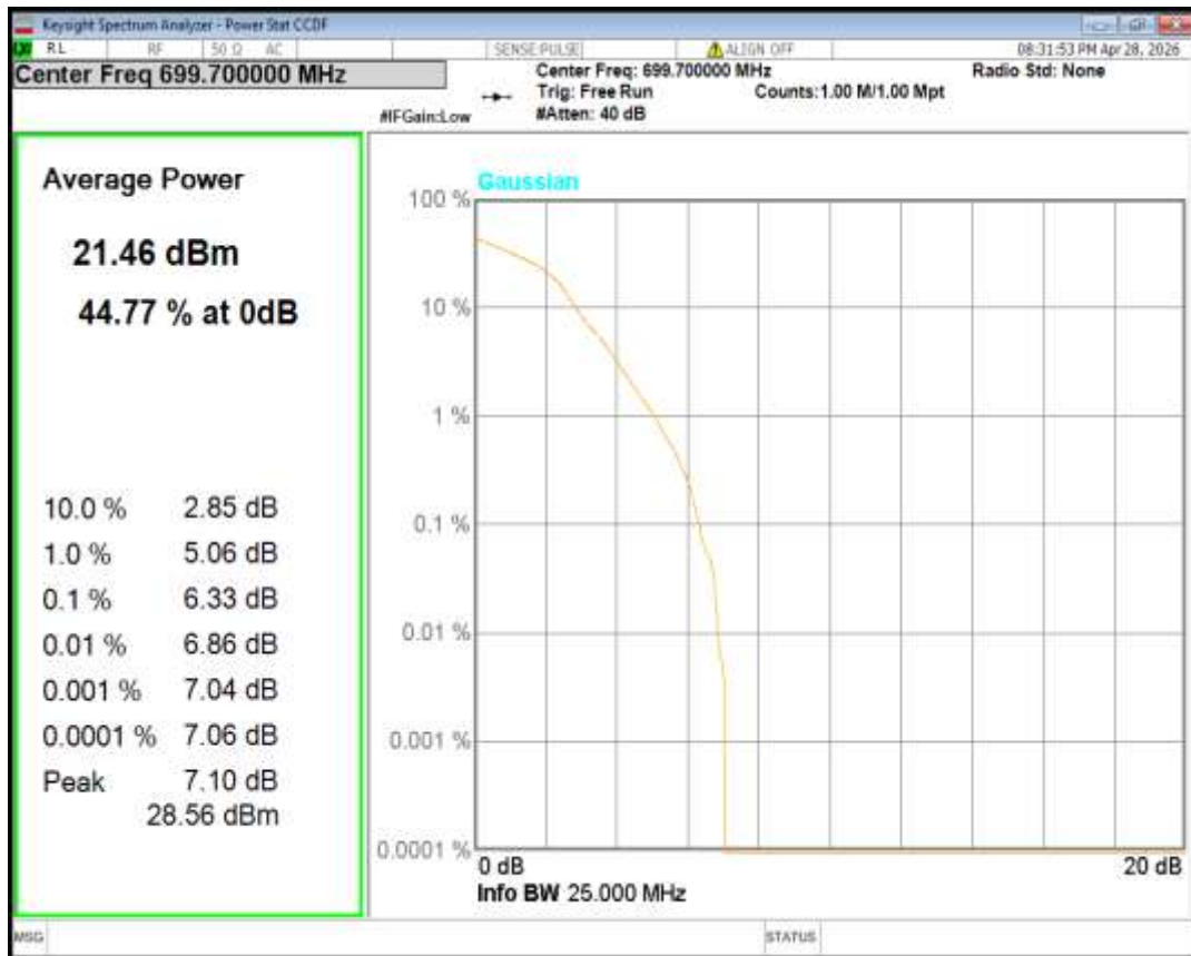
Band12 16QAM BW=1.4MHz Channel=23095 RB Size=1 Position=#0
