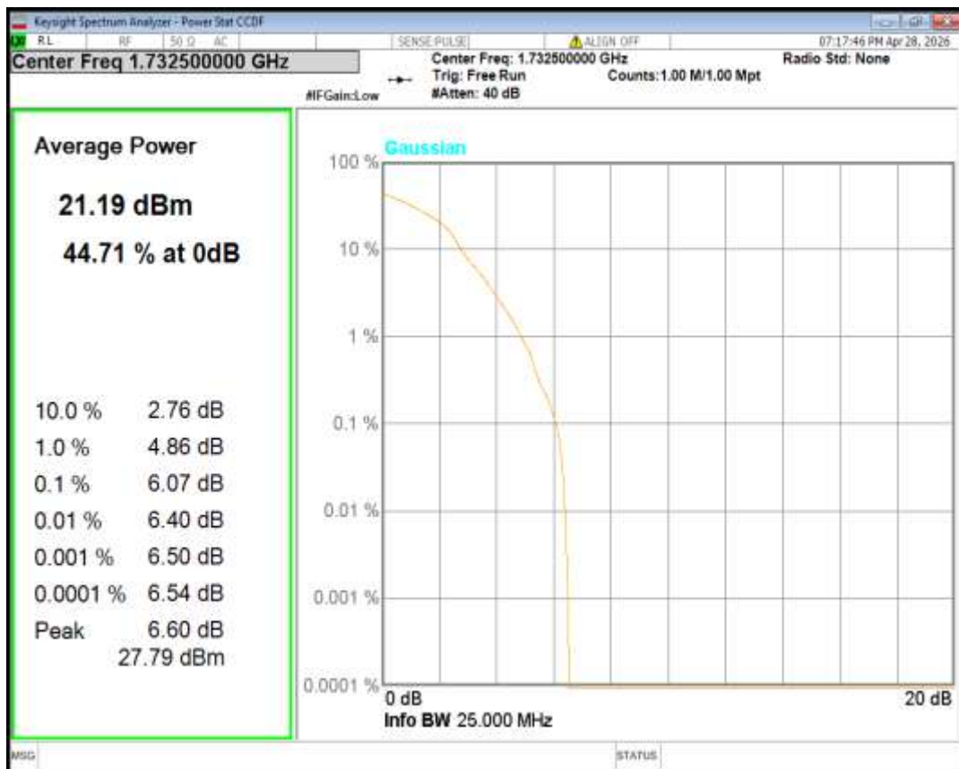
Band4 16QAM BW=10MHz Channel=20350 RB Size=1 Position=#0
