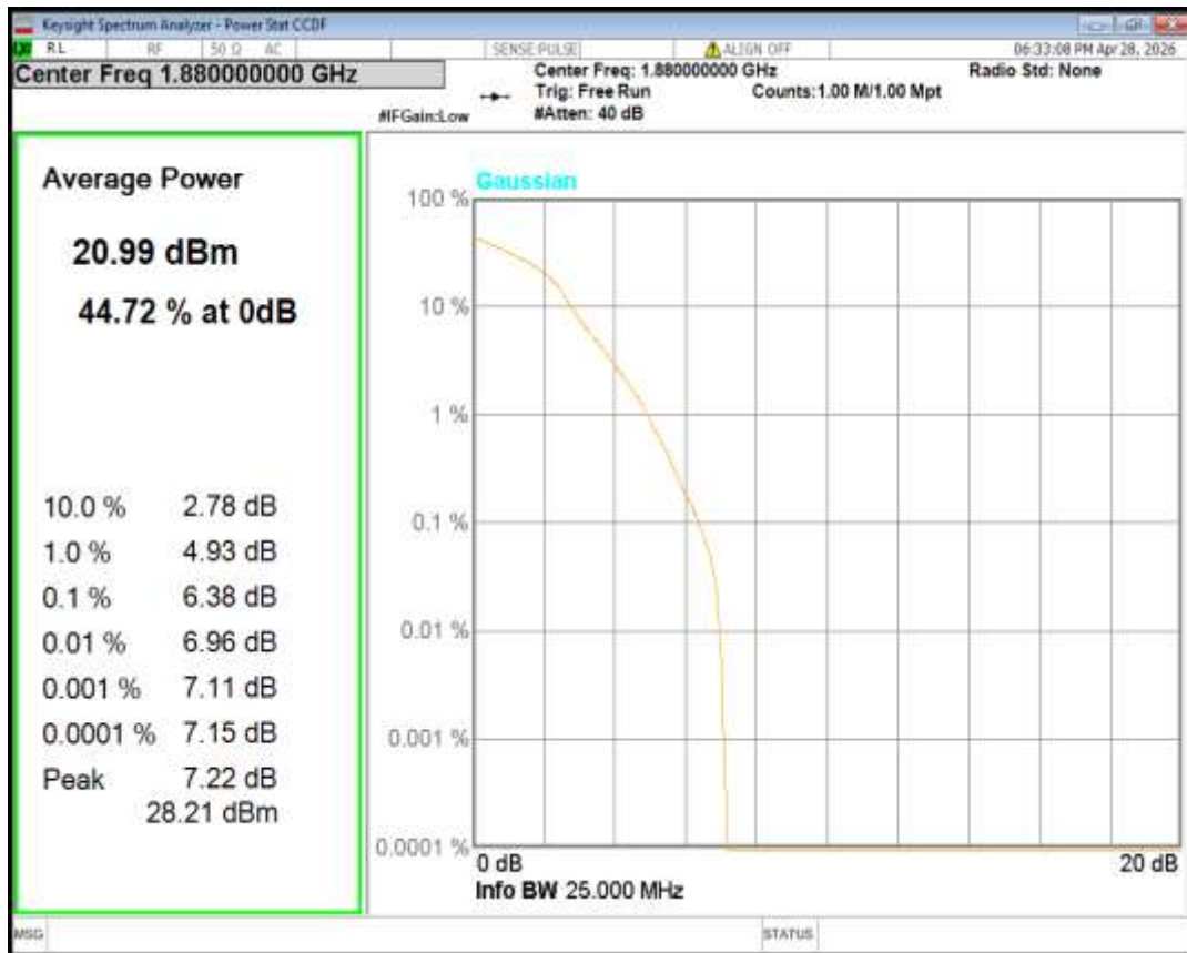
Band2 16QAM BW=10MHz Channel=19150 RB Size=1 Position=#0
