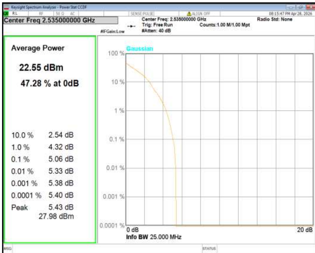
Band7 QPSK BW=10MHz Channel=21400 RB Size=1 Position=#0
