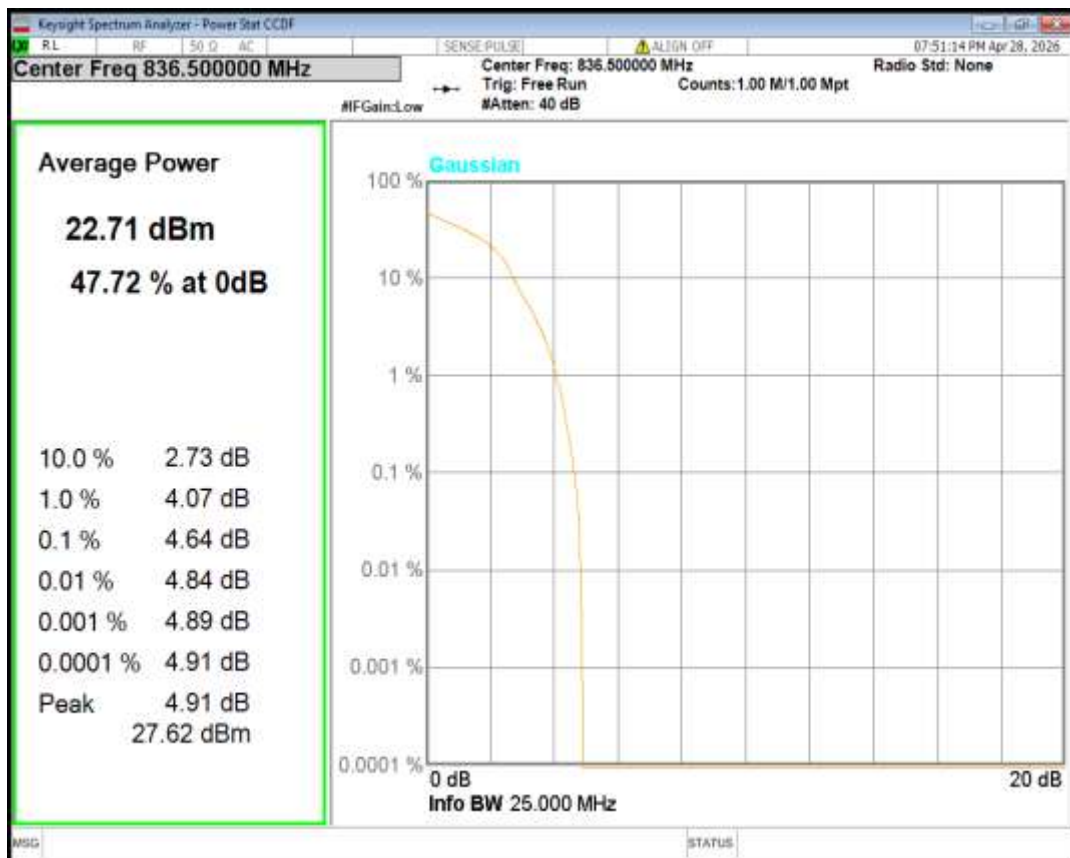
Band5 QPSK BW=1.4MHz Channel=20407 RB Size=1 Position=#0
