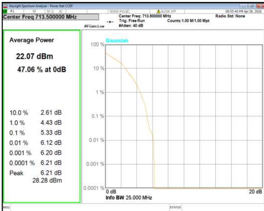
Band2 16QAM BW=1.4MHz Channel=18607 RB Size=1 Position=#0
