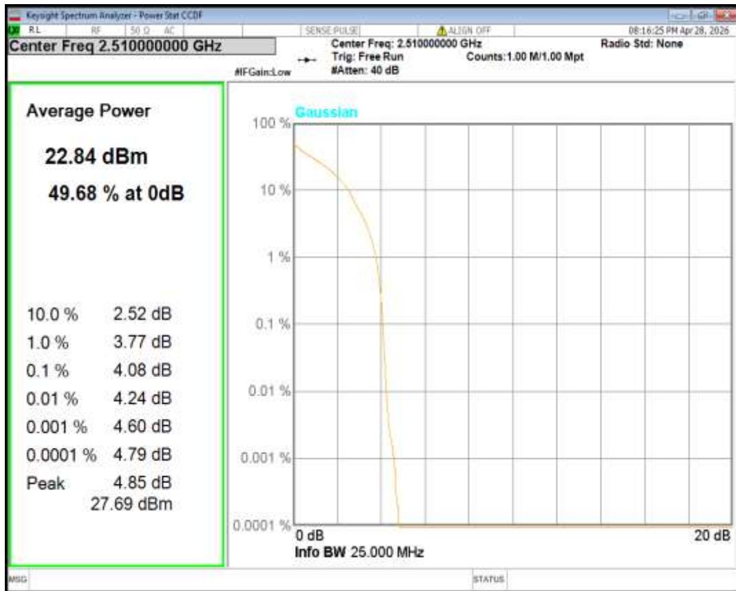
Band7 QPSK BW=20MHz Channel=21100 RB Size=1 Position=#0
