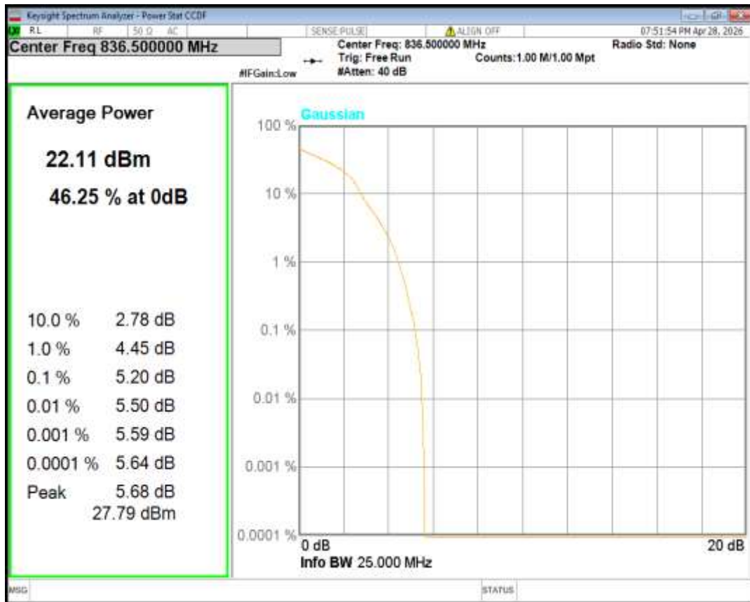
Band5 16QAM BW=10MHz Channel=20600 RB Size=1 Position=#0
