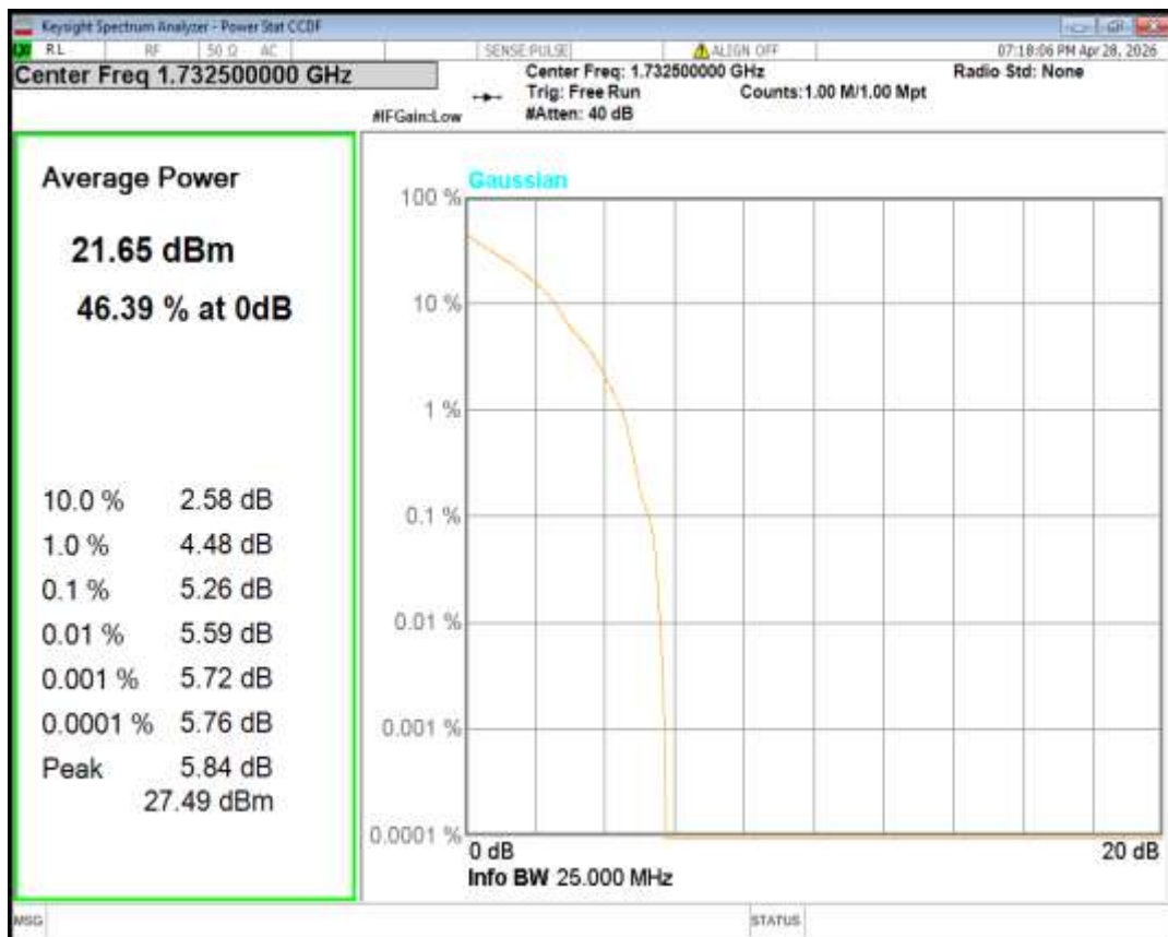
Band4 QPSK BW=15MHz Channel=20025 RB Size=1 Position=#0
