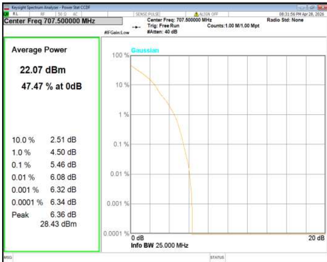
Band12 QPSK BW=10MHz Channel=23095 RB Size=1 Position=#0
