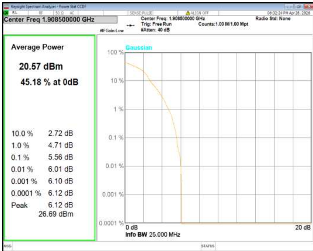
Band2 16QAM BW=5MHz Channel=18625 RB Size=1 Position=#0
