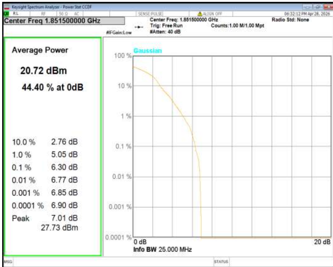
Band2 16QAM BW=3MHz Channel=18900 RB Size=1 Position=#0
