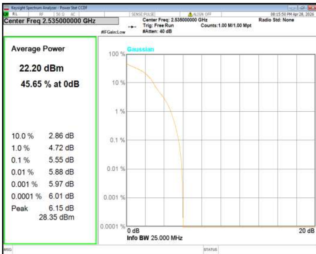
Band7 16QAM BW=10MHz Channel=21400 RB Size=1 Position=#0
