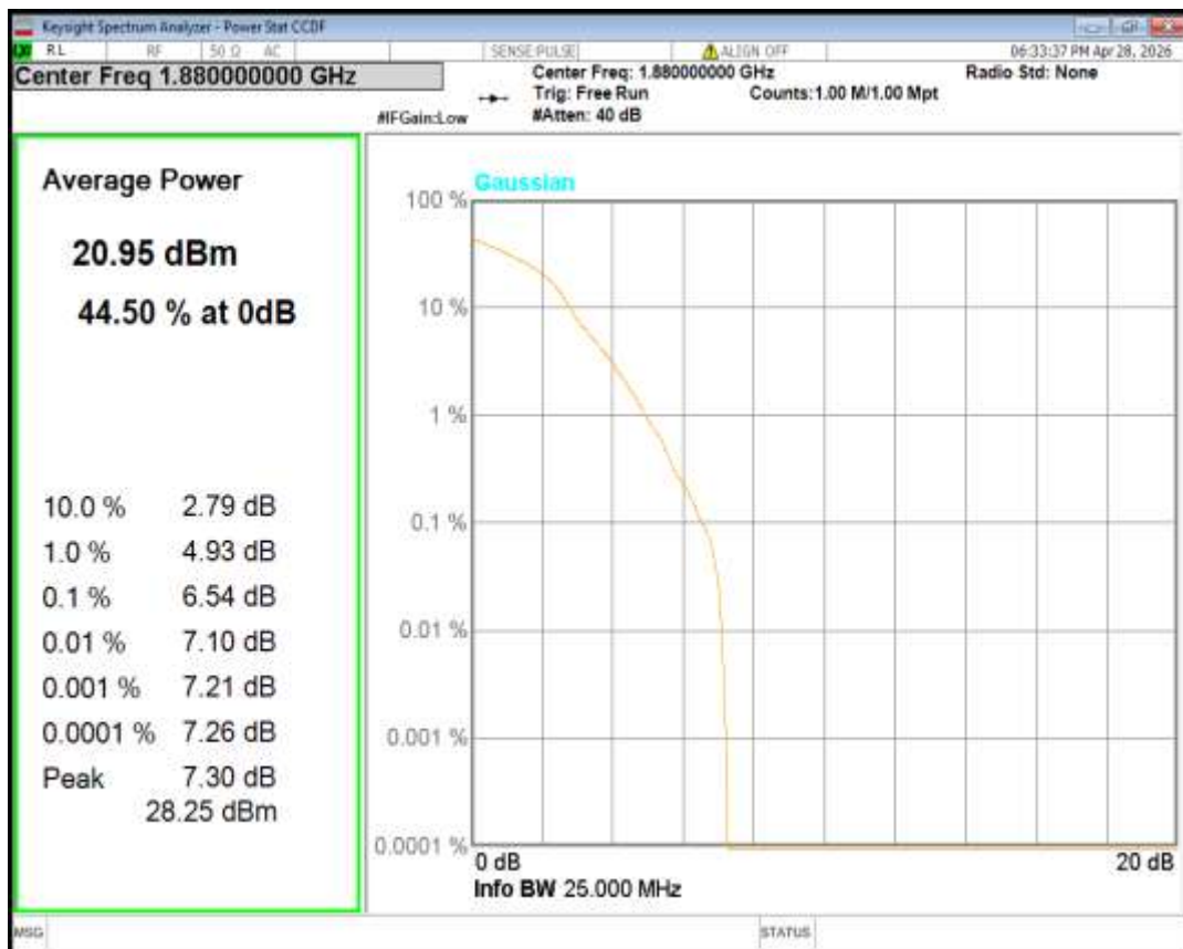
Band2 16QAM BW=3MHz Channel=18615 RB Size=1 Position=#0
