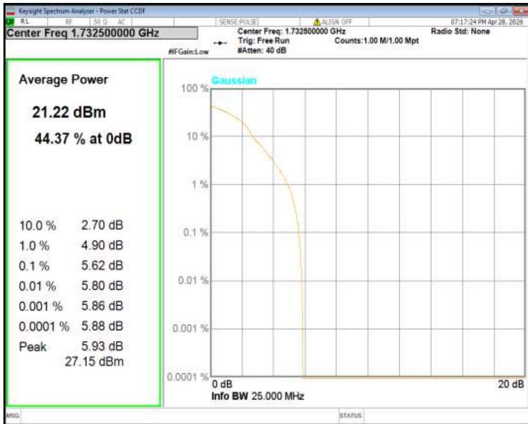
Band4 QPSK BW=1.4MHz Channel=20175 RB Size=1 Position=#0
