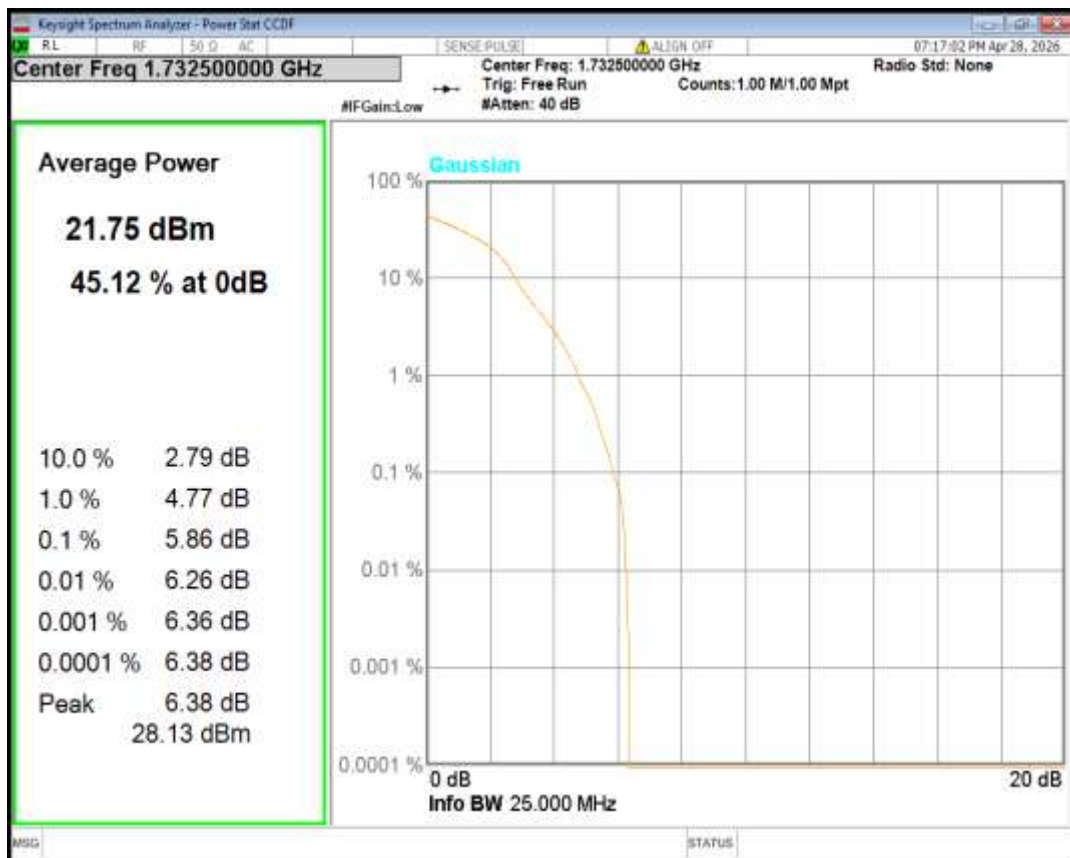
Band4 16QAM BW=3MHz Channel=20385 RB Size=1 Position=#0
