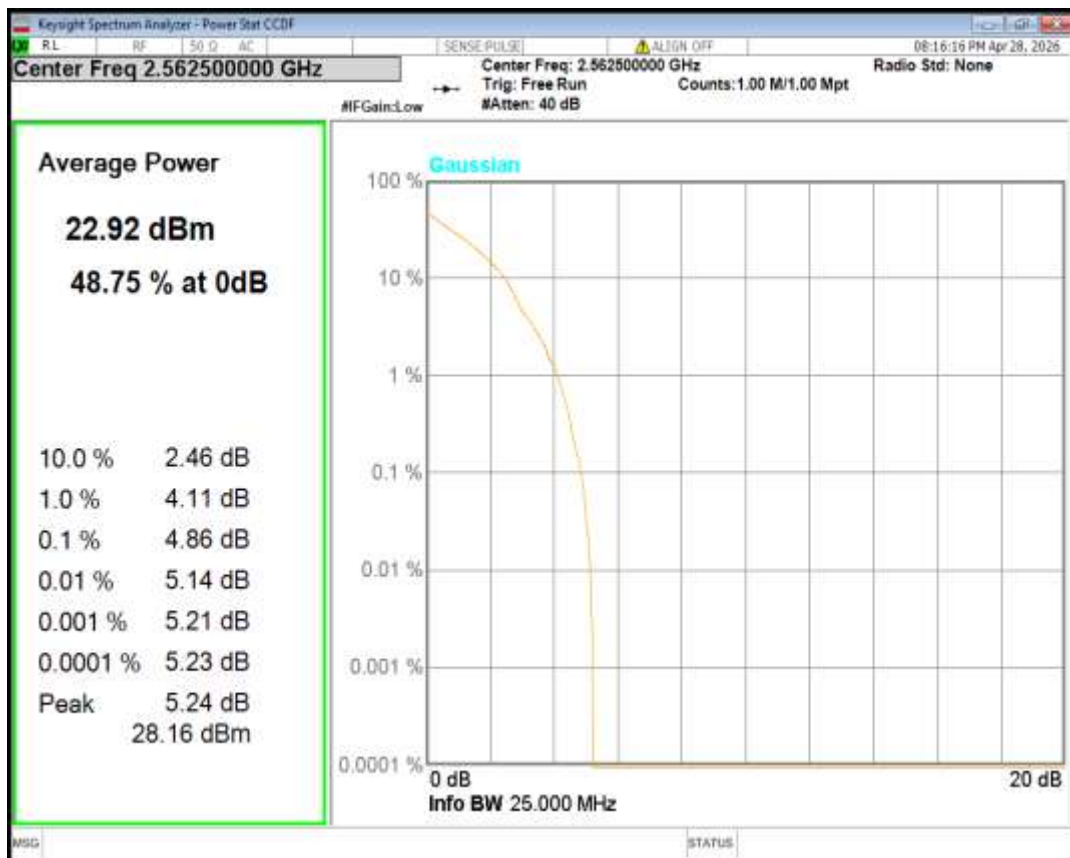
Band7 QPSK BW=20MHz Channel=20850 RB Size=1 Position=#0
