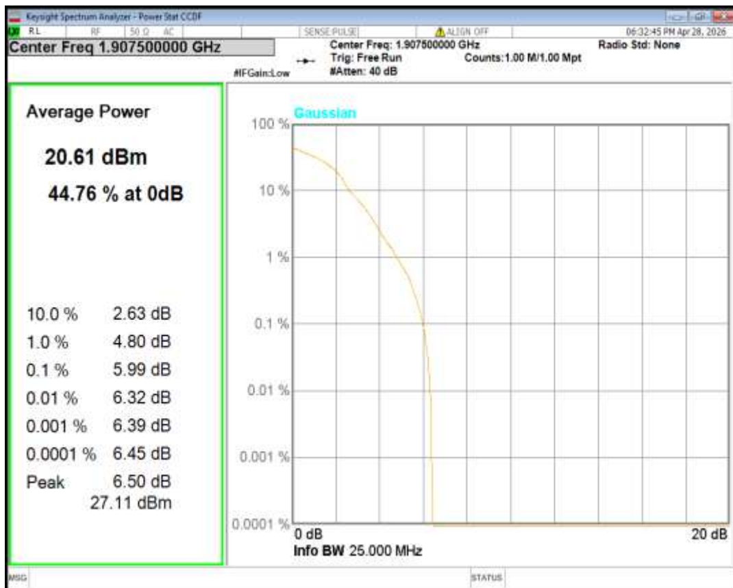
Band2 QPSK BW=1.4MHz Channel=18607 RB Size=1 Position=#0
