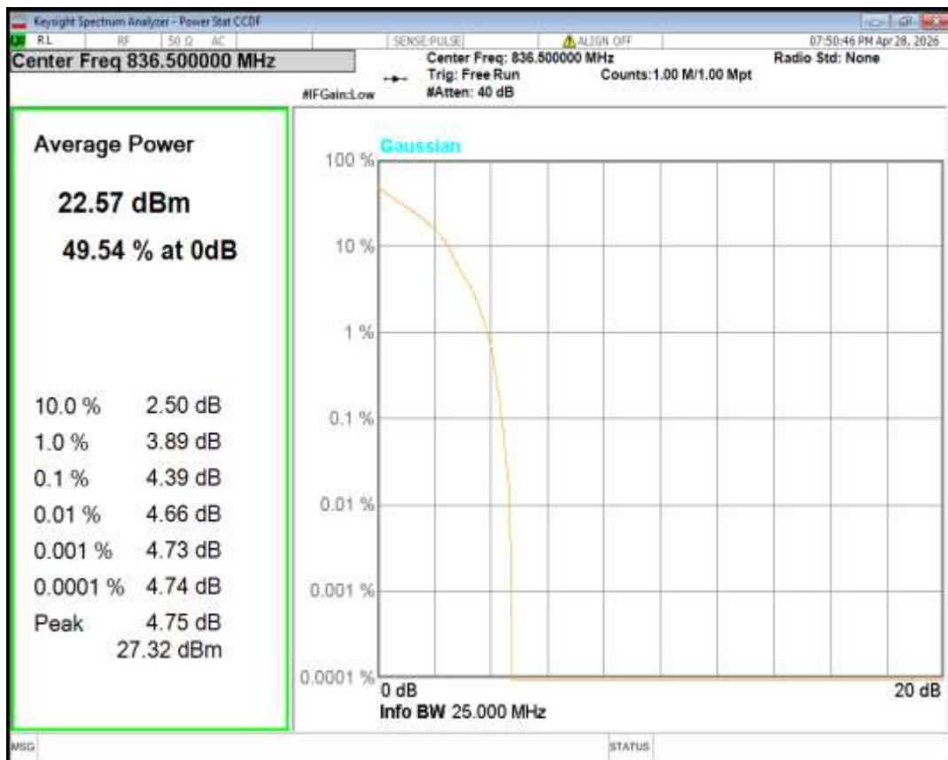
Band5 QPSK BW=1.4MHz Channel=20643 RB Size=1 Position=#0
