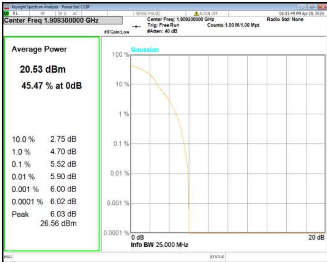
Band2 16QAM BW=10MHz Channel=18650 RB Size=1 Position=#0
