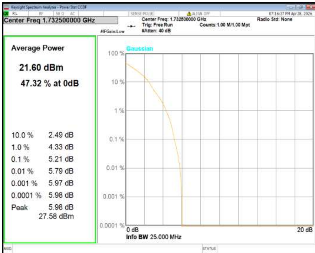
Band4 QPSK BW=1.4MHz Channel=20393 RB Size=1 Position=#0
