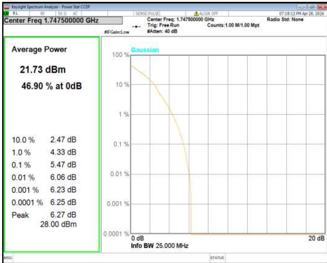
Band4 QPSK BW=15MHz Channel=20175 RB Size=1 Position=#0
