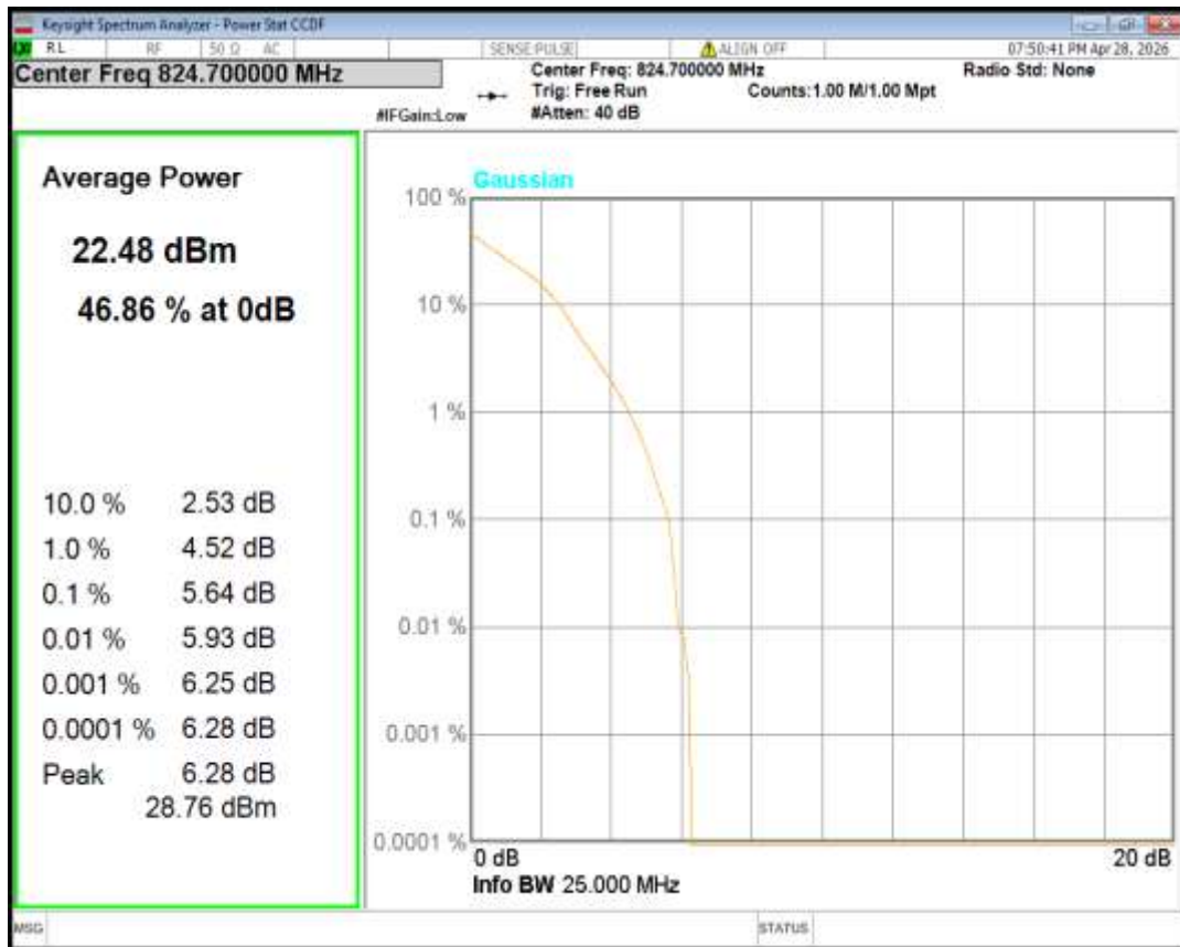
Band5 16QAM BW=5MHz Channel=20525 RB Size=1 Position=#0
