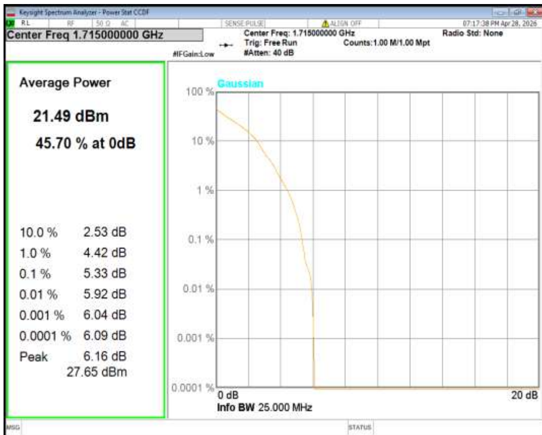
Band4 QPSK BW=10MHz Channel=20175 RB Size=1 Position=#0
