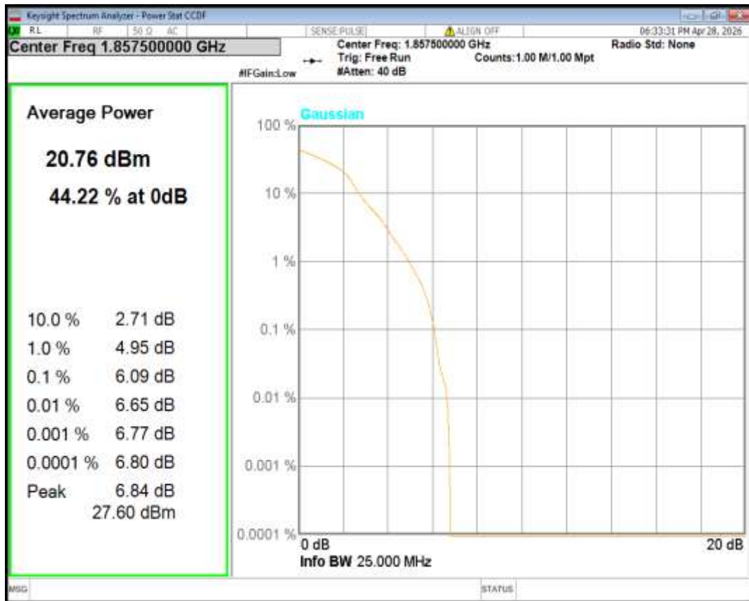
Band2 16QAM BW=20MHz Channel=19100 RB Size=1 Position=#0
