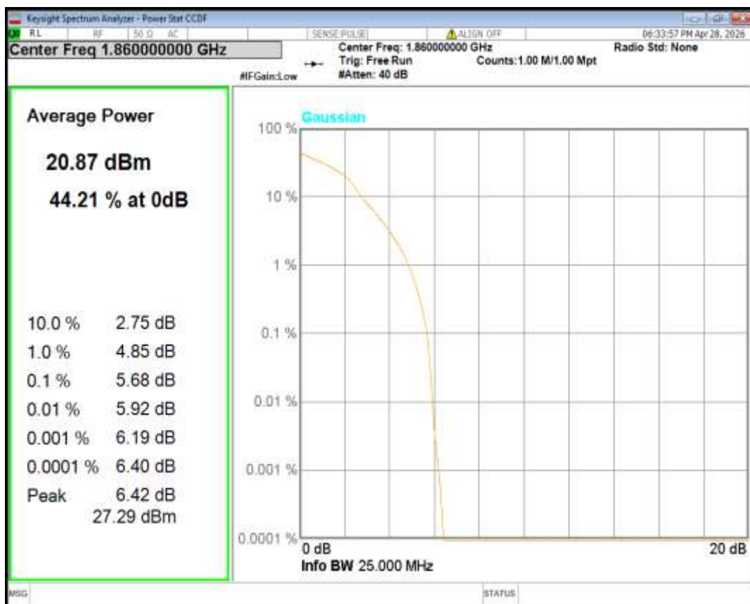
Band2 16QAM BW=15MHz Channel=19125 RB Size=1 Position=#0
