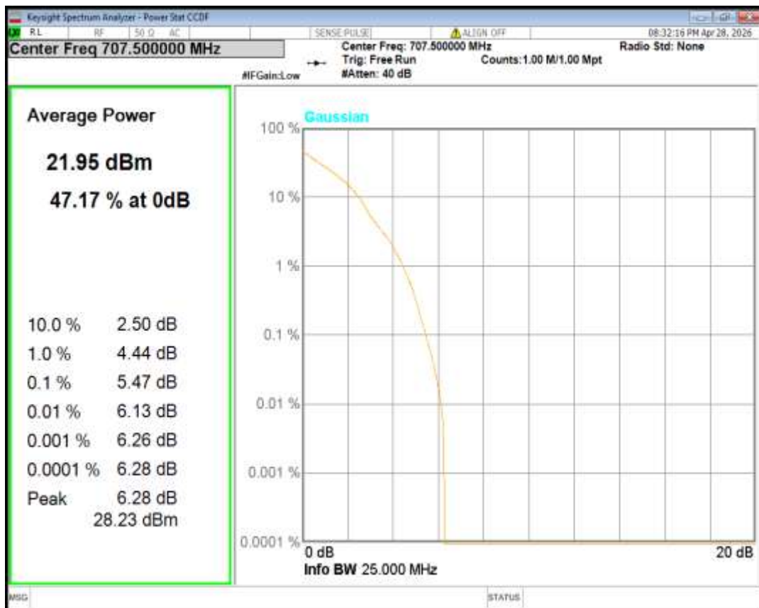
Band12 QPSK BW=3MHz Channel=23165 RB Size=1 Position=#0
