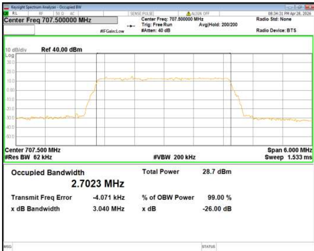
Band12 16QAM BW=3MHz Channel=23165 RB Size=15 Position=#0
