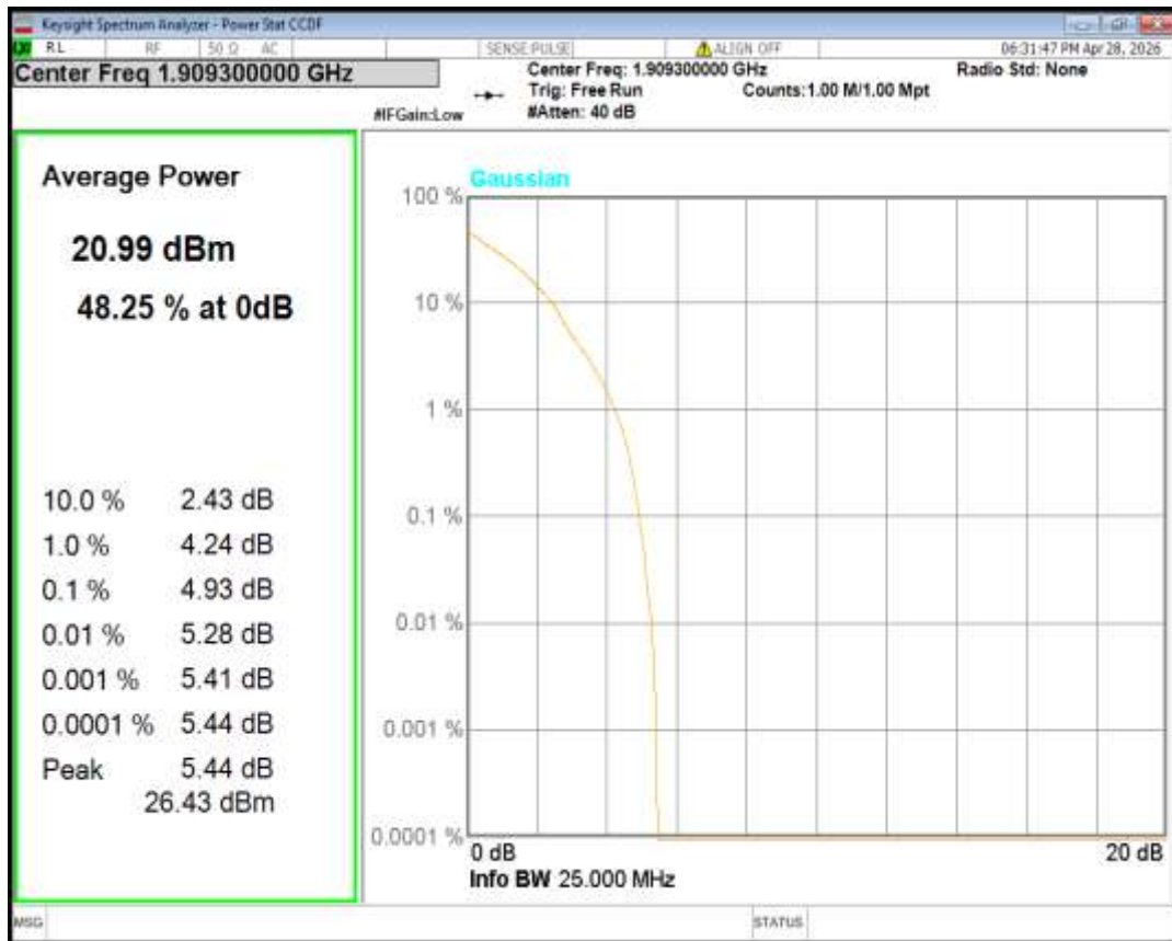
Band2 16QAM BW=5MHz Channel=19175 RB Size=1 Position=#0
