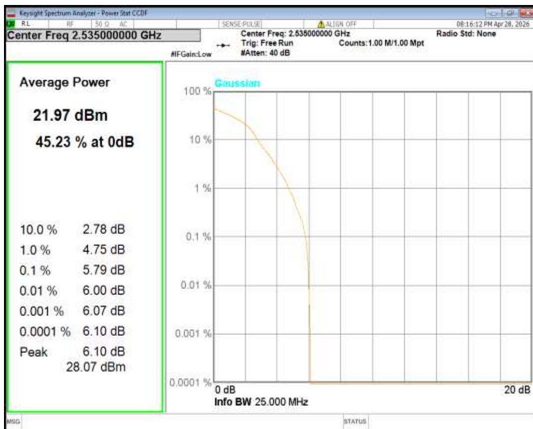
Band7 16QAM BW=15MHz Channel=21375 RB Size=1 Position=#0
