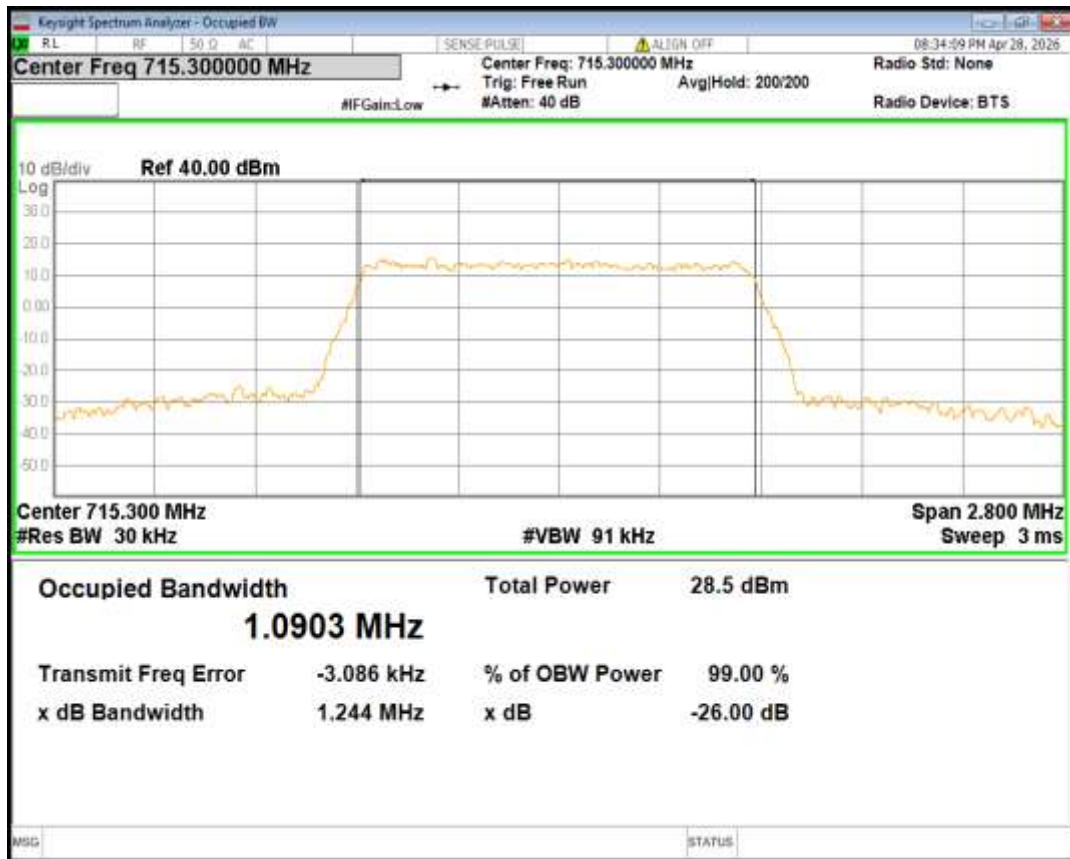
Band12 16QAM BW=10MHz Channel=23060 RB Size=50 Position=#0
