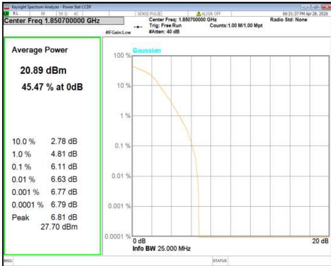
Band2 16QAM BW=1.4MHz Channel=18900 RB Size=1 Position=#0
