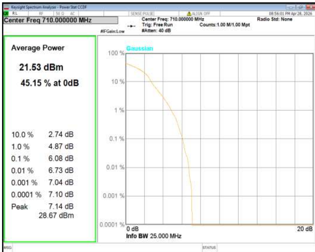
Band17 16QAM BW=10MHz Channel=23800 RB Size=1 Position=#0
