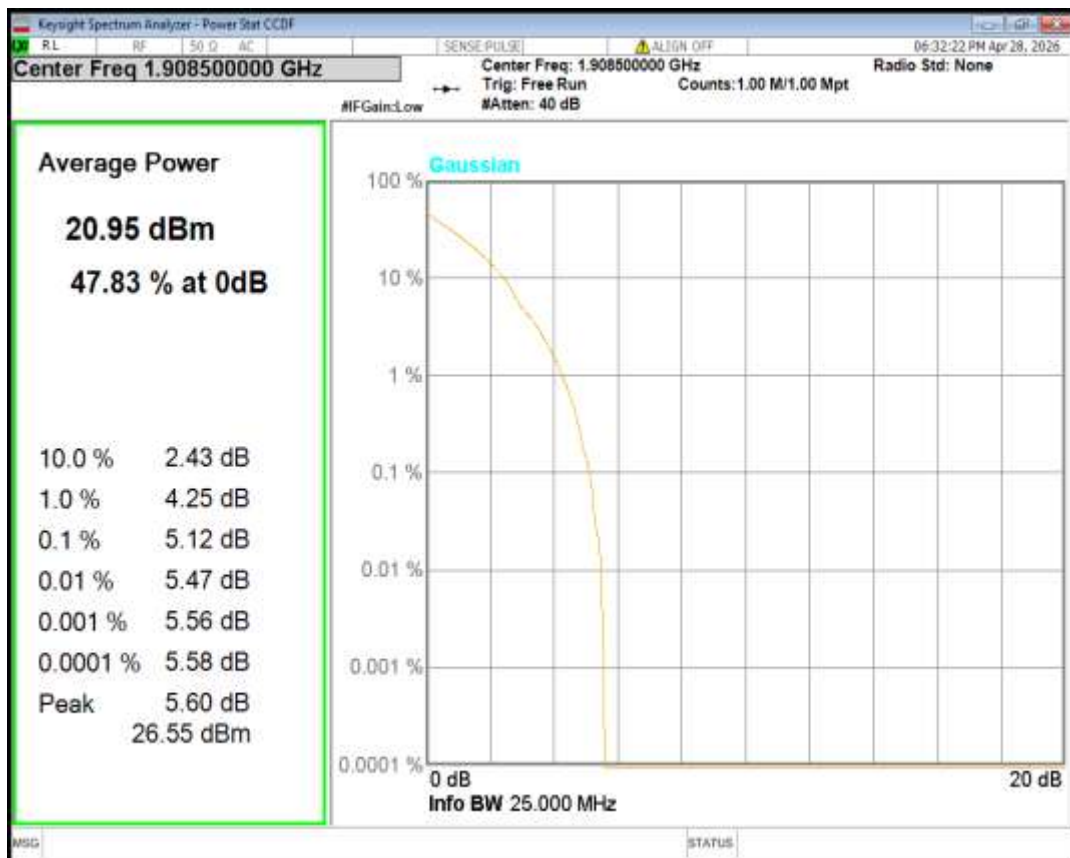
Band2 QPSK BW=5MHz Channel=18625 RB Size=1 Position=#0
