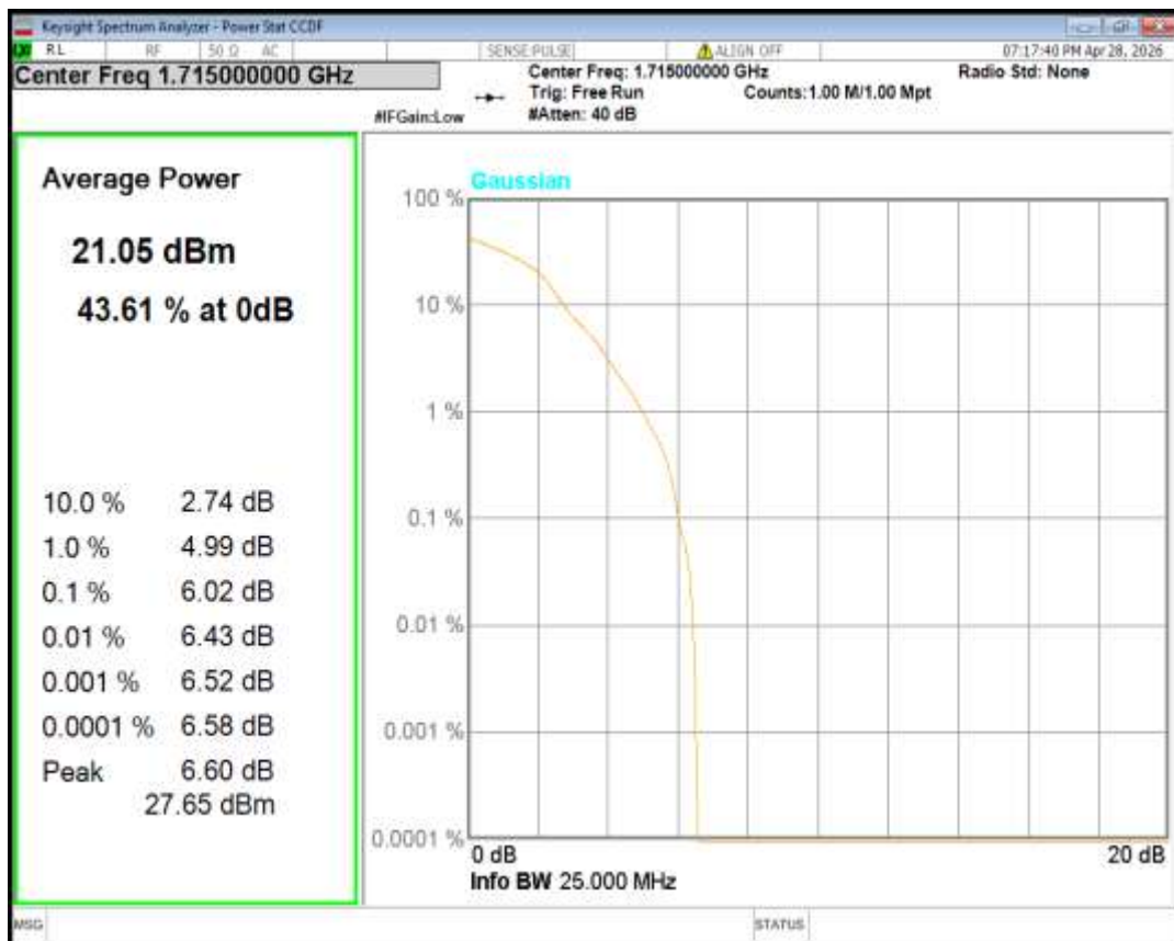
Band4 16QAM BW=15MHz Channel=20175 RB Size=1 Position=#0
