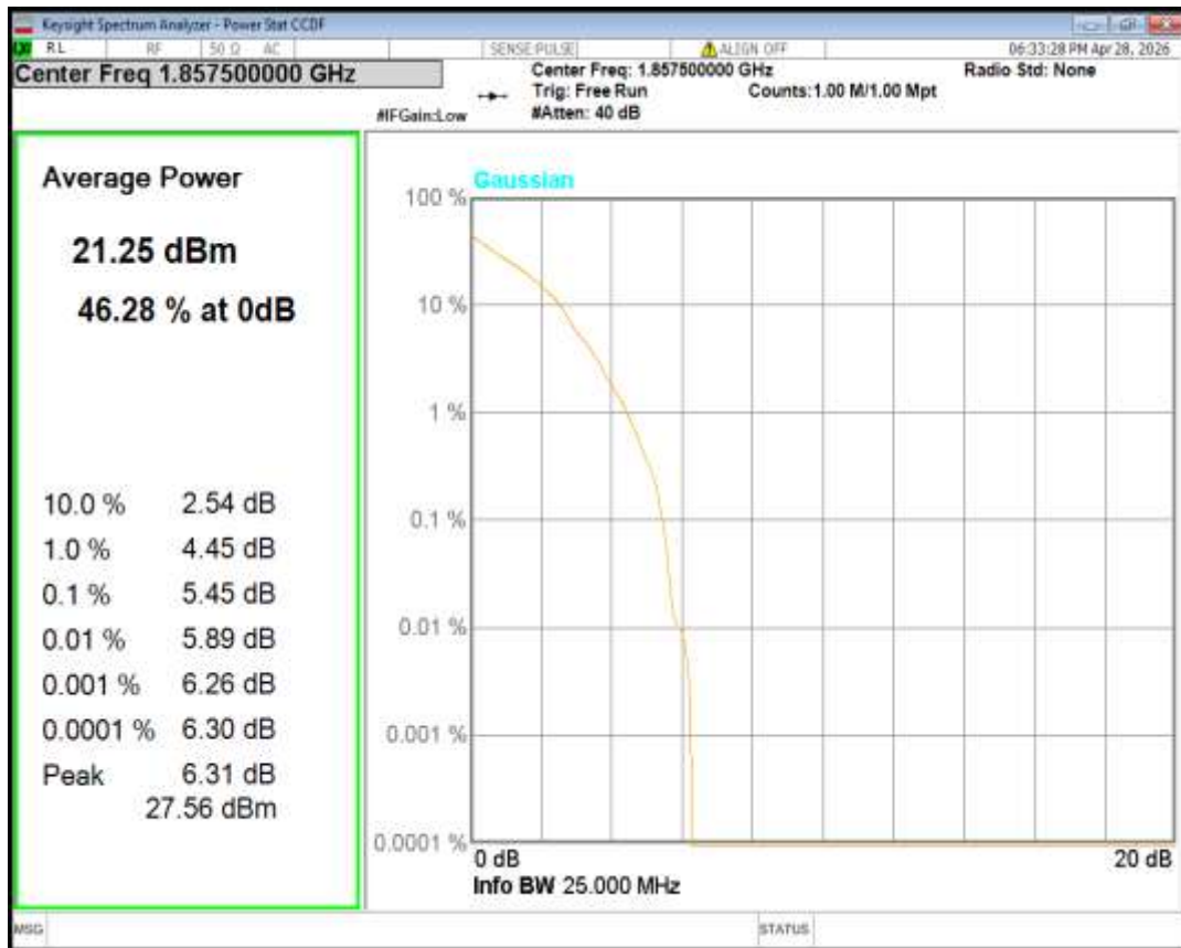
Band2 QPSK BW=15MHz Channel=18900 RB Size=1 Position=#0
