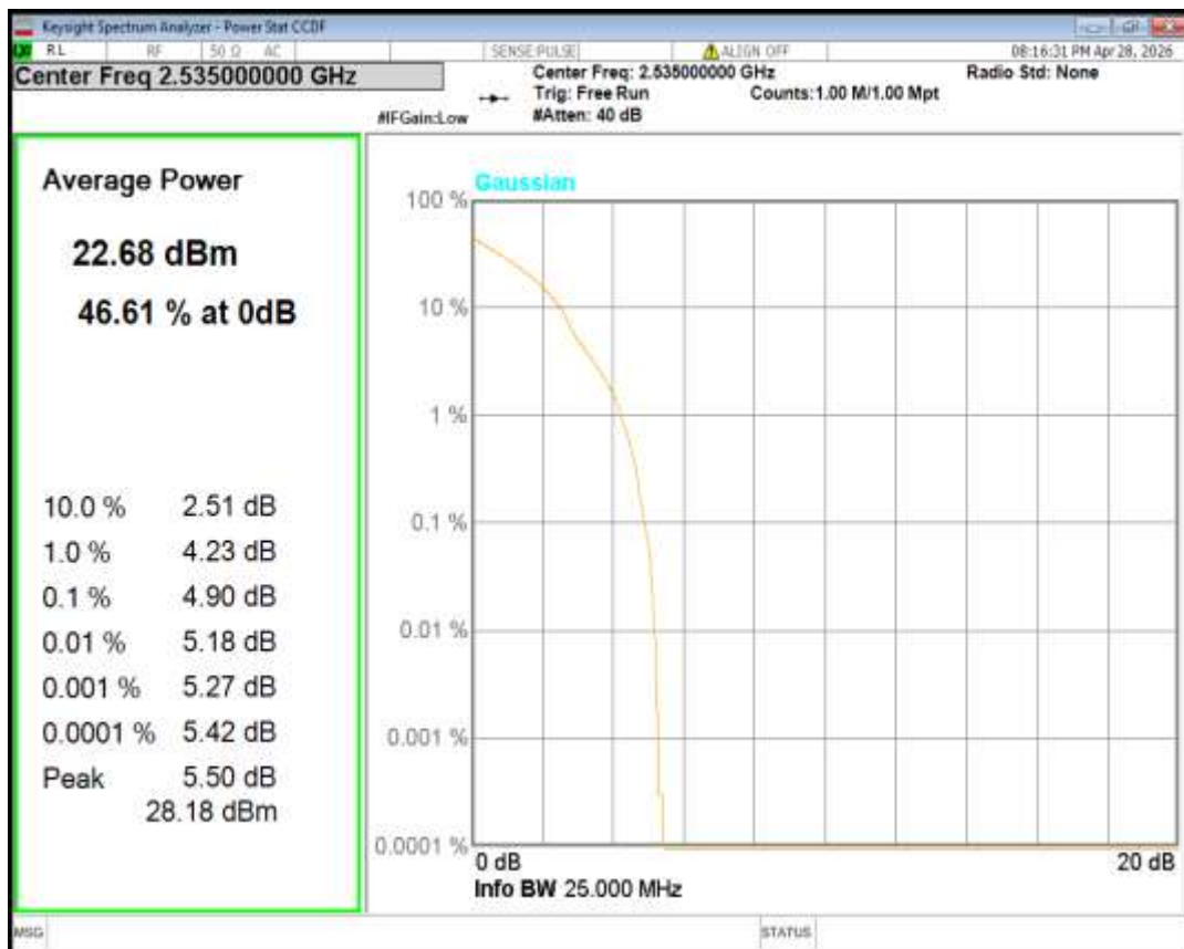
Band7 QPSK BW=20MHz Channel=21350 RB Size=1 Position=#0
