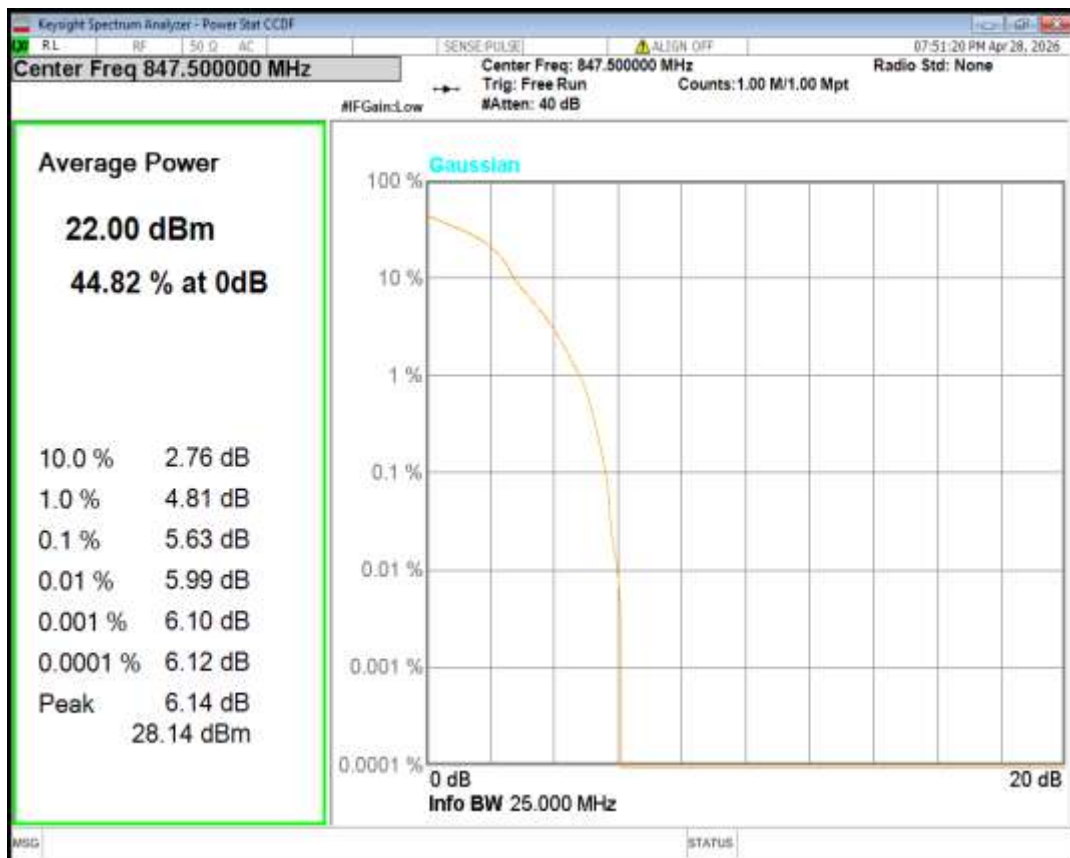
Band5 16QAM BW=5MHz Channel=20425 RB Size=1 Position=#0
