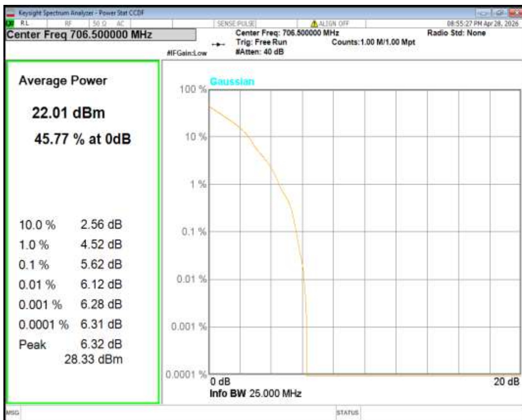
Band17 QPSK BW=5MHz Channel=23790 RB Size=1 Position=#0
