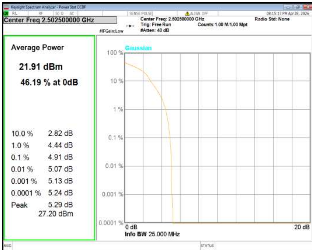
Band7 16QAM BW=5MHz Channel=21100 RB Size=1 Position=#0
