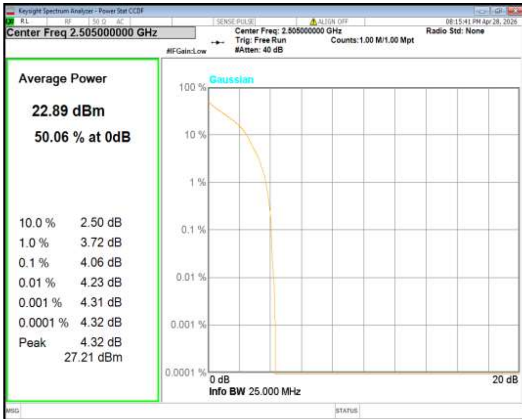
Band7 QPSK BW=10MHz Channel=21100 RB Size=1 Position=#0
