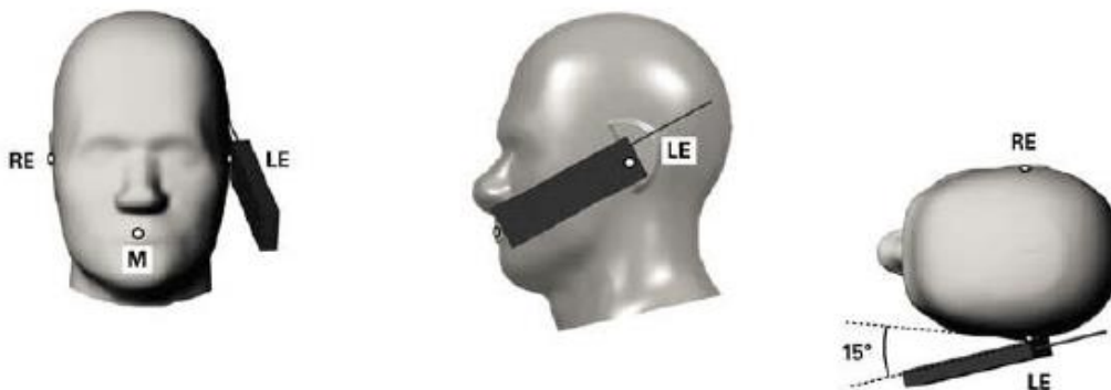
Fig.11.4 Illustration for Tilted Position
