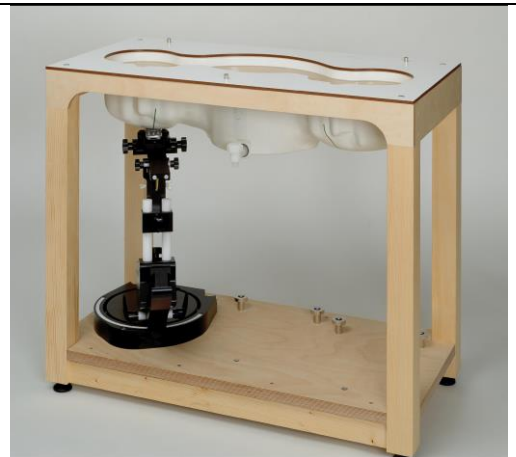
Fig. 8.7 Photo of SAM Twin Phantom
