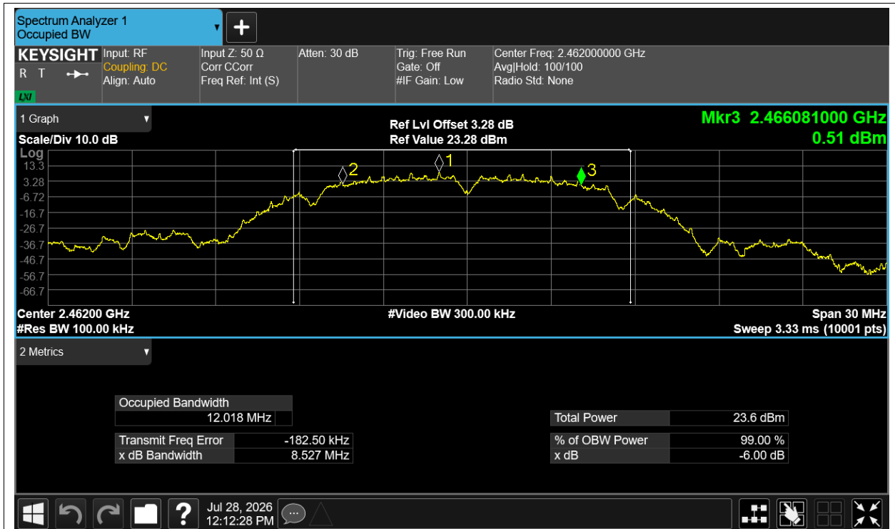
-6dB Bandwidth NVNT g 2412MHz Ant1
