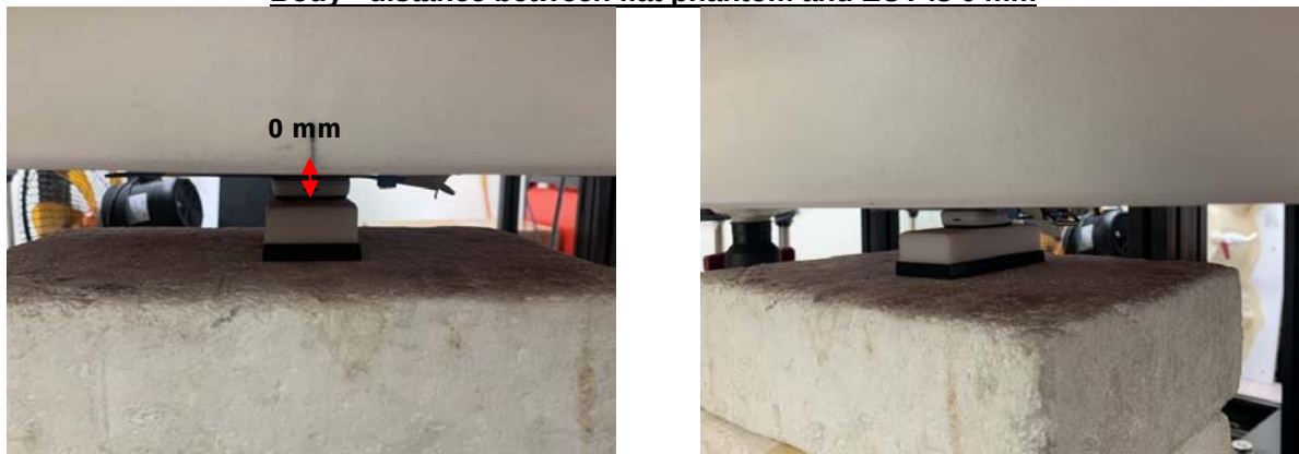
Fig.3 Back side of EUT to flat phantom
