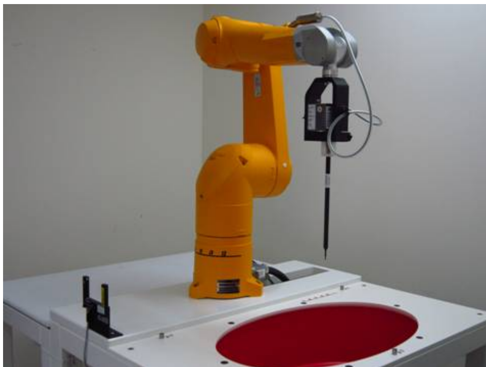
Fig.1 Photograph of the SAR measurement system
