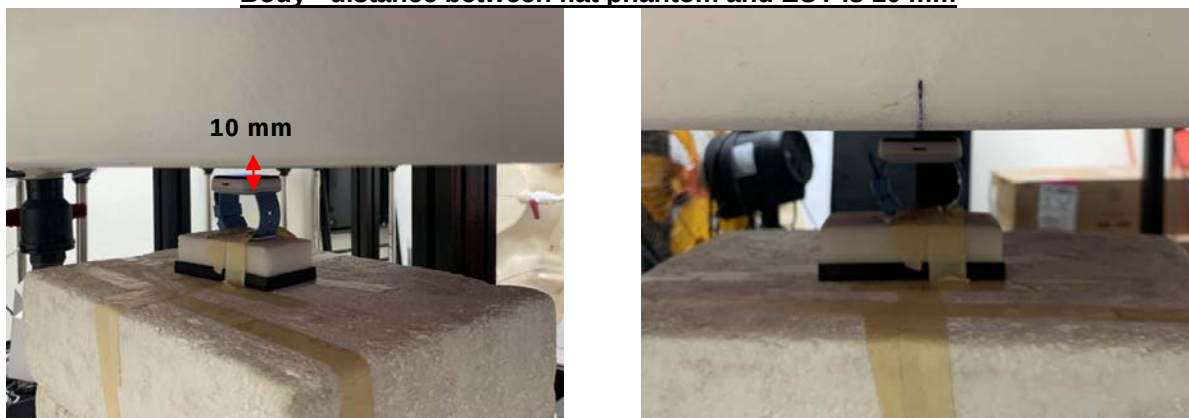
Fig.4 Front side of EUT to flat phantom
