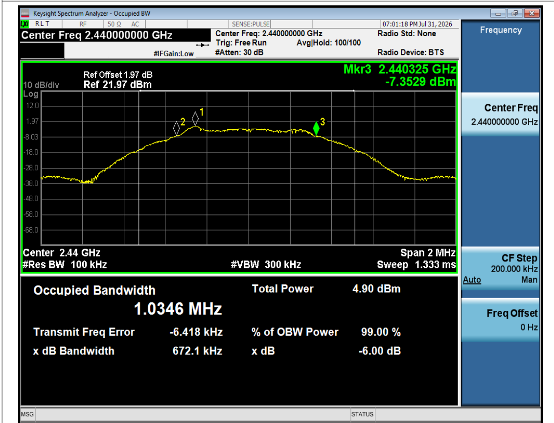
-6dB Bandwidth NVNT GFSK 2440MHz Ant1
