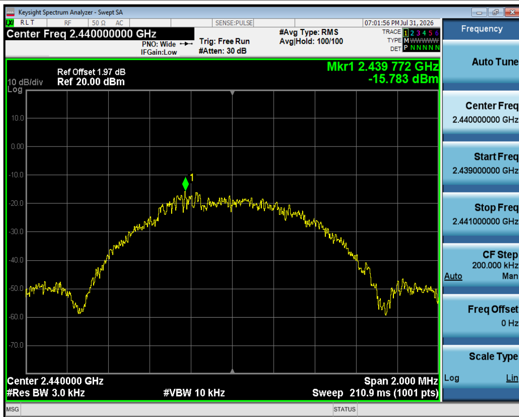
PSD NVNT GFSK 2440MHz Ant1
