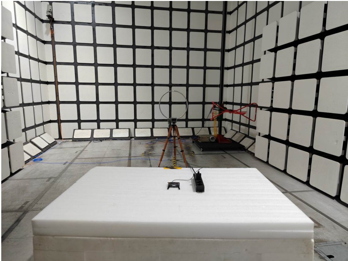
Radiated Emissions View (Below 1 GHz)
