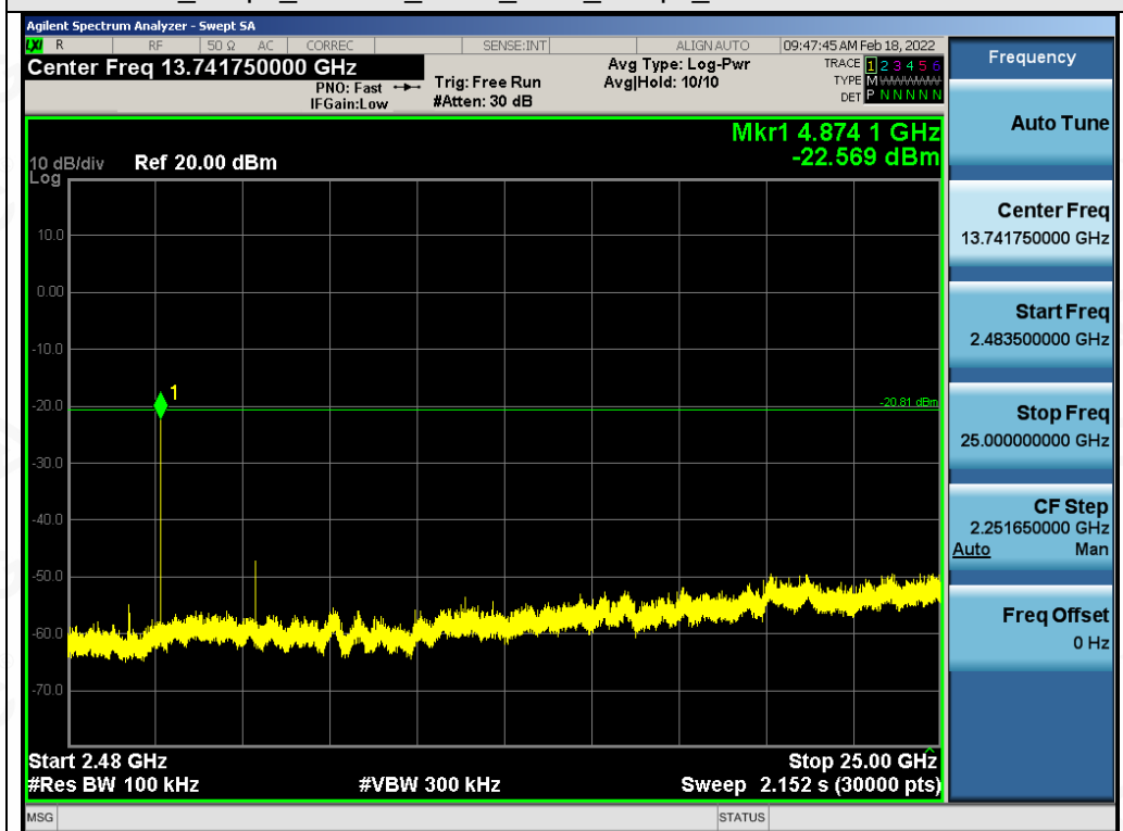
Test_Graph_802.11b_ANT1_2437_1Mbps_Higher Band Emissions
