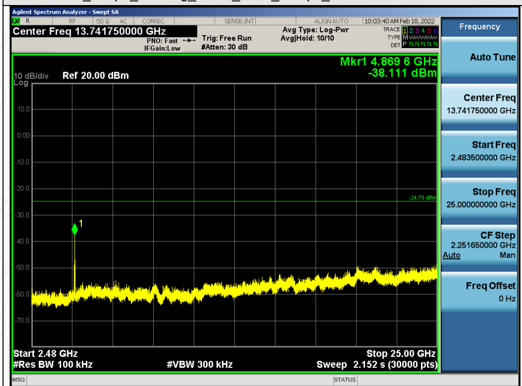
Test_Graph_802.11g_ANT1_2437_6Mbps_Higher Band Emissions
