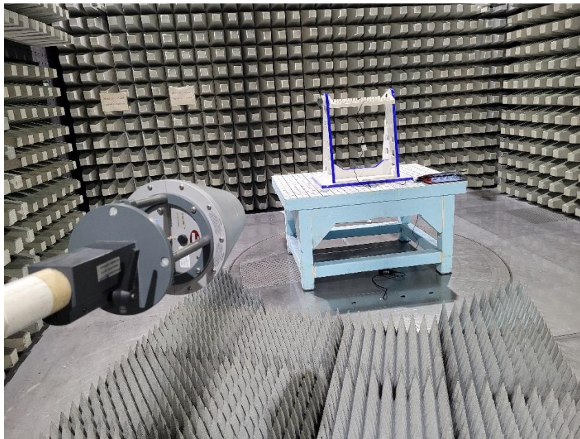
Photo 5 Radiated Test Setup 1 - 18 GHz
