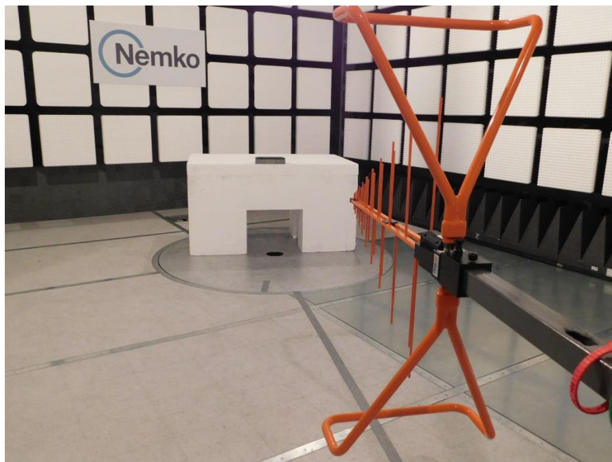
Figure 8.1-3: Radiated emissions setup photo
