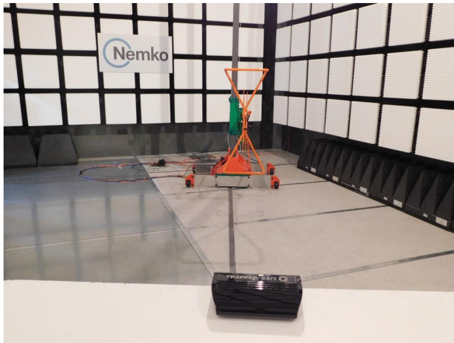
Figure 8.1-2: Radiated emissions setup photo
