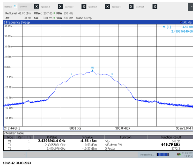
Figure 8.4-1: 6 dB bandwidth, sample plot Mid channel, 1 MHz BW
