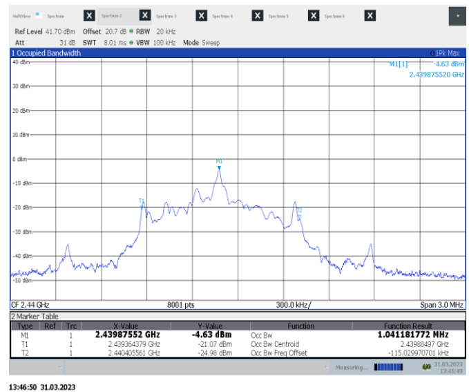
Figure 8.4-2: 99% bandwidth, sample plot Mid channel, 1 MHz BW
