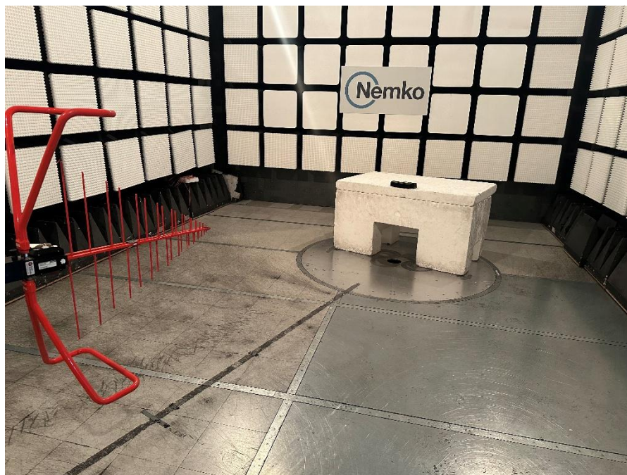
Figure 7.1-4: Radiated spurious emissions – below 1 GHz
