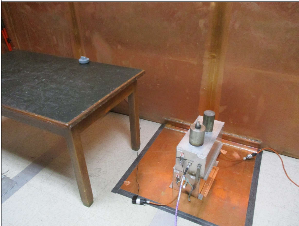
Test Setup for Powerline Conducted Emissions Test
