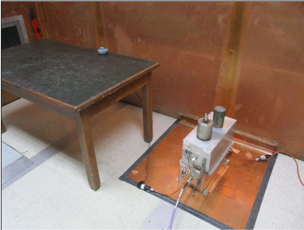
Test Setup for Powerline Conducted Emissions Test
