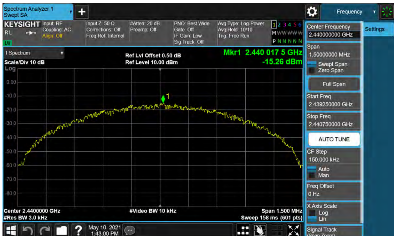
Figure 8: Power Spectral Density, 2440MHz
