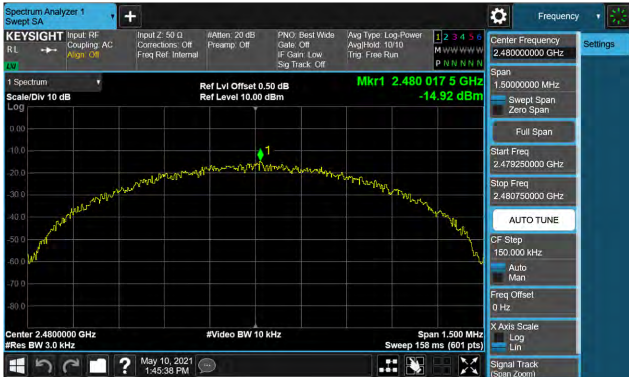
Figure 9: Power Spectral Density, 2480MHz
