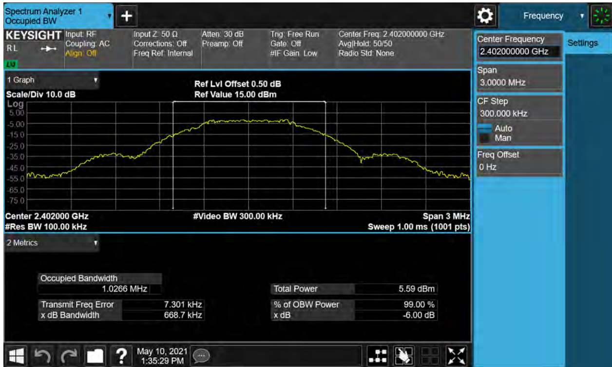
Figure 4: 6dB Bandwidth and 99% Bandwidth, 2402MHz
