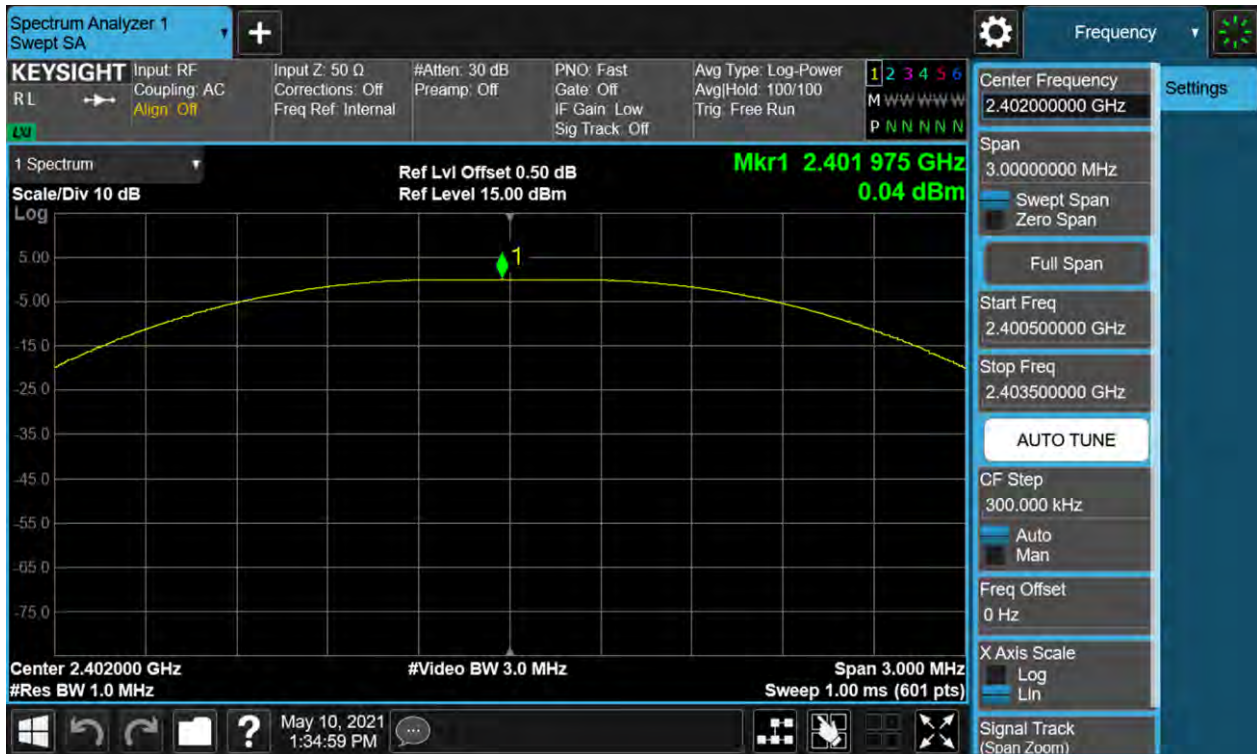
Figure 2: Peak Output Power, 2440MHz
