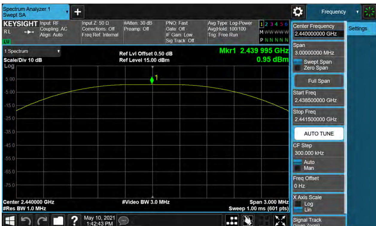
Figure 2: Peak Output Power, 2440MHz
