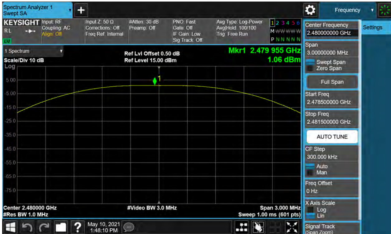
Figure 3: Peak Output Power, 2480MHz
