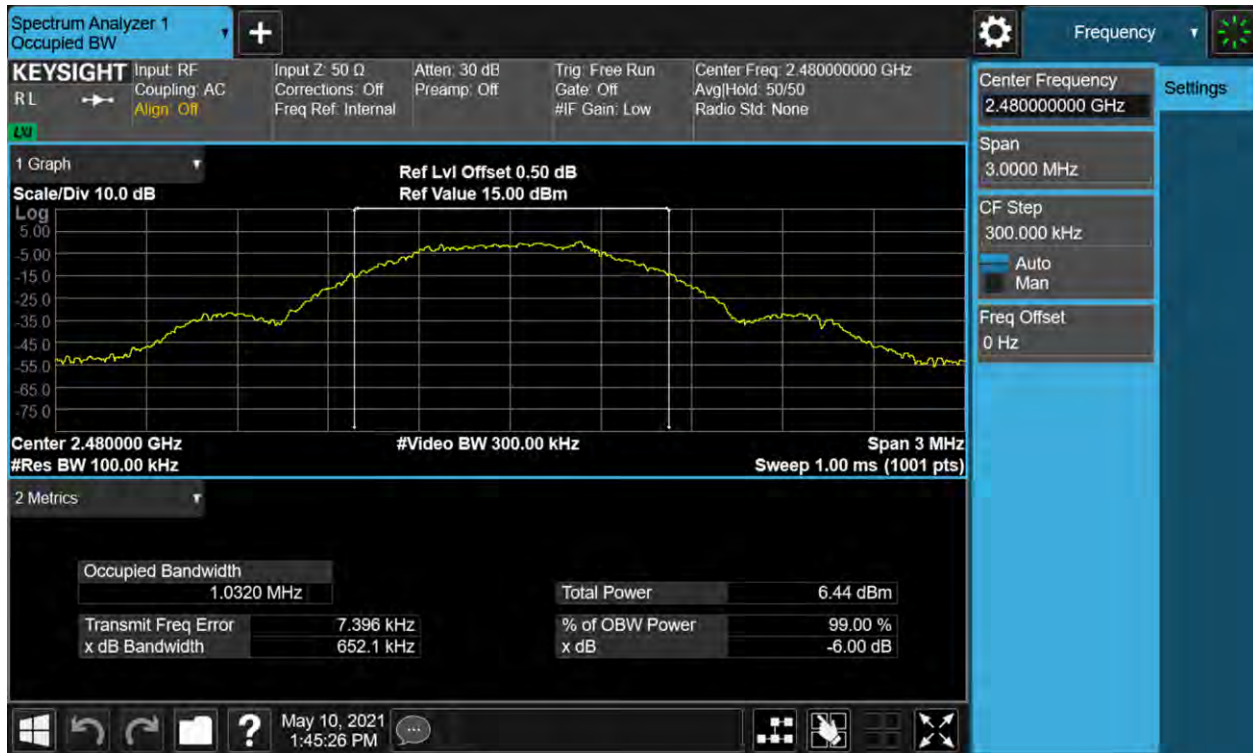
Figure 6: 6dB Bandwidth and 99% Bandwidth, 2480MHz
