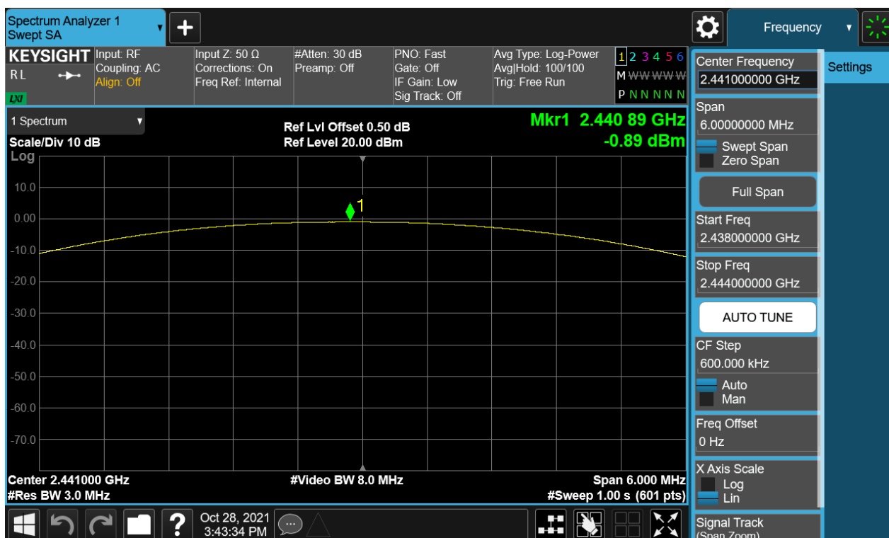
Figure 2: Maximum Conducted Output Power, 2441MHz, GFSK
